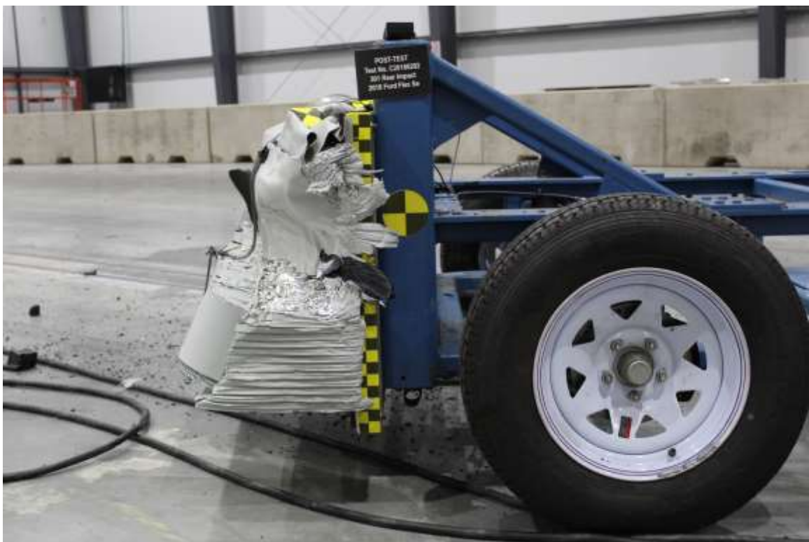
Figure A-22: Post-Test MDB Left Side View
