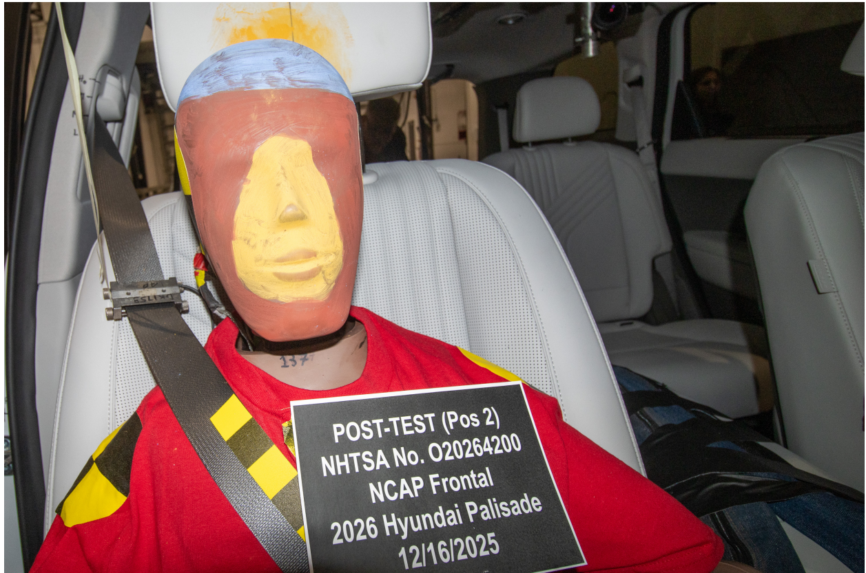
Figure A-71: Post-Test Passenger Dummy Face
