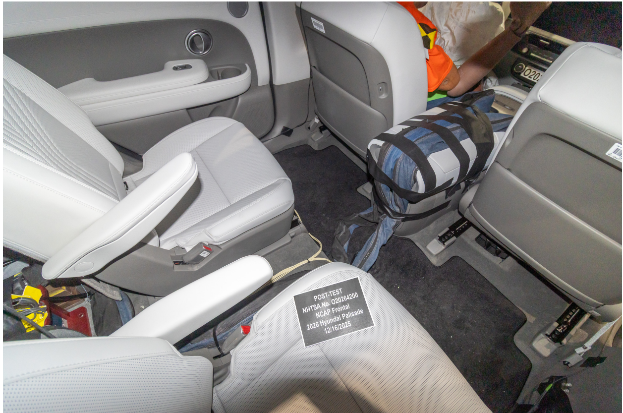
Figure A-29: Post-Test Dummy Cable Routing
