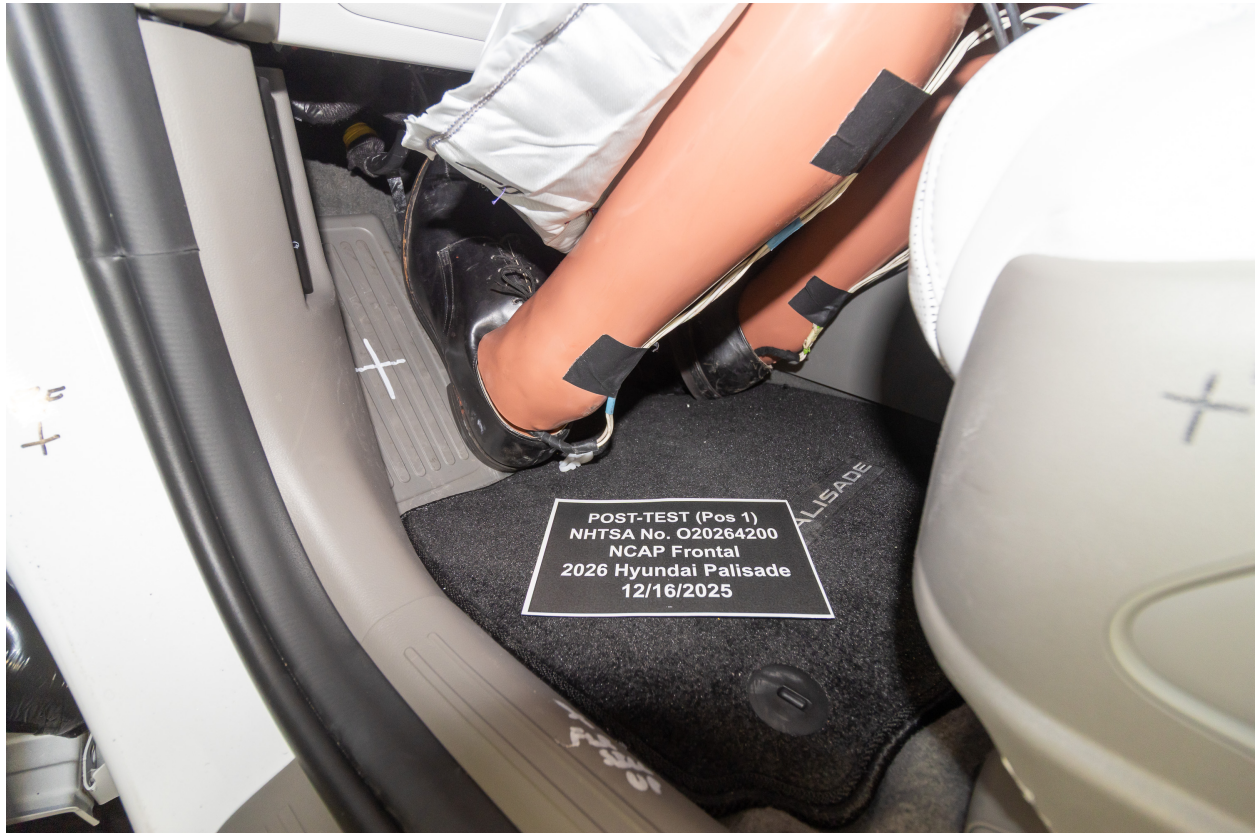
Figure A-43: Post-Test Driver Dummy Feet
