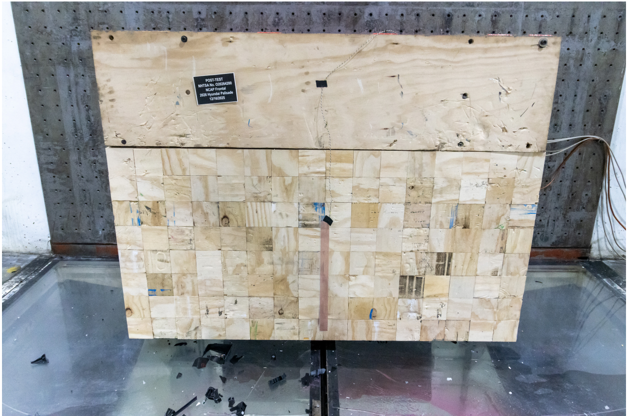
Figure A-3: Post-Test Load Cell Wall
