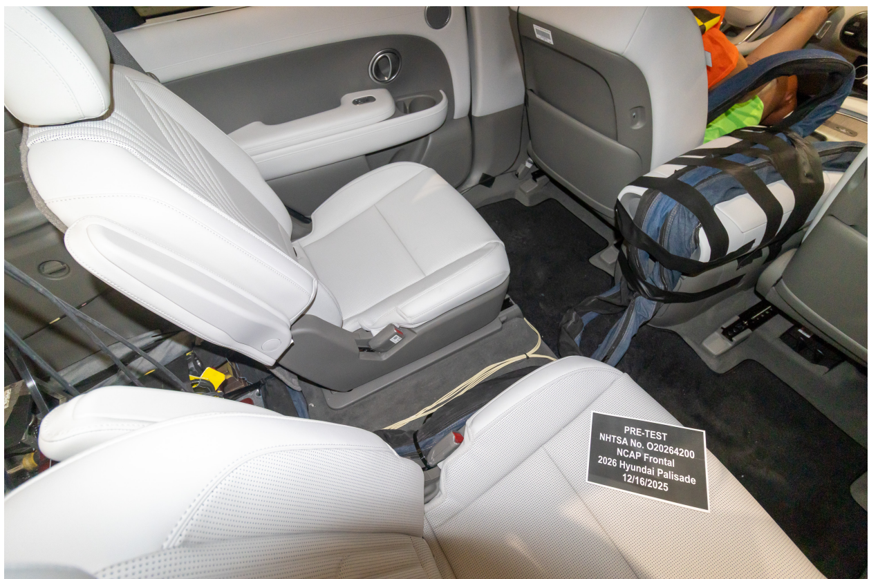
Figure A-28: Pre-Test Dummy Cable Routing
