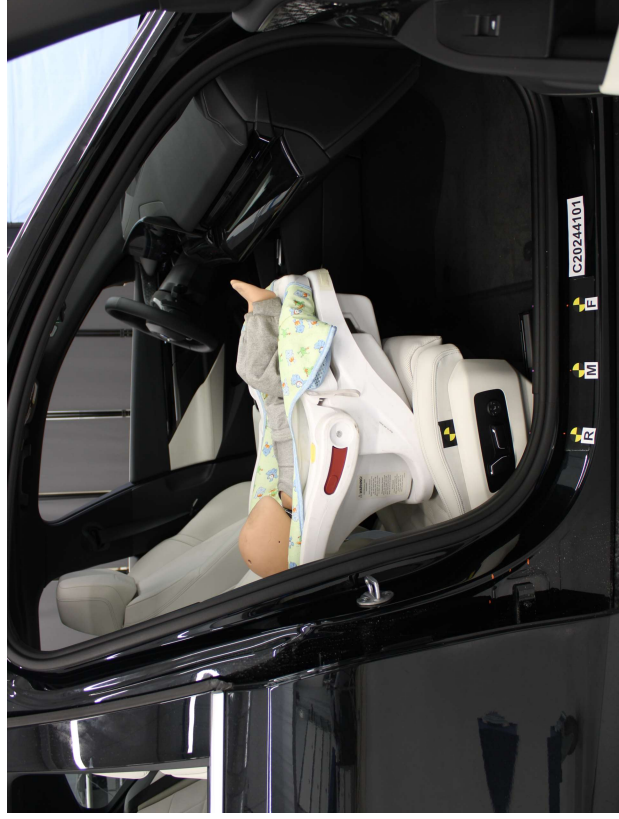
Cosco Arriva WBBase, Unbelted, Forward Facing, Rearward Seat Track
