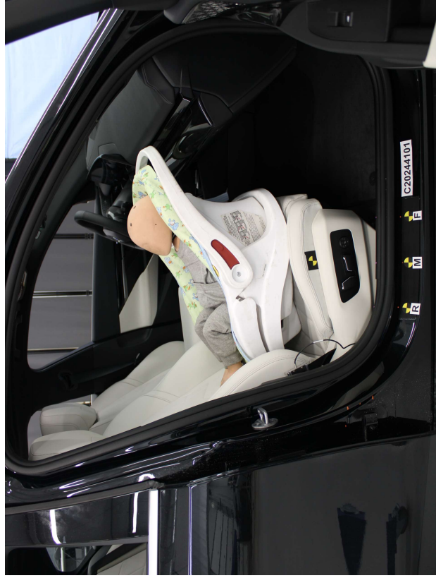
Cosco Arriva WBBase, Unbelted, Rear Facing, Forward Seat Track
