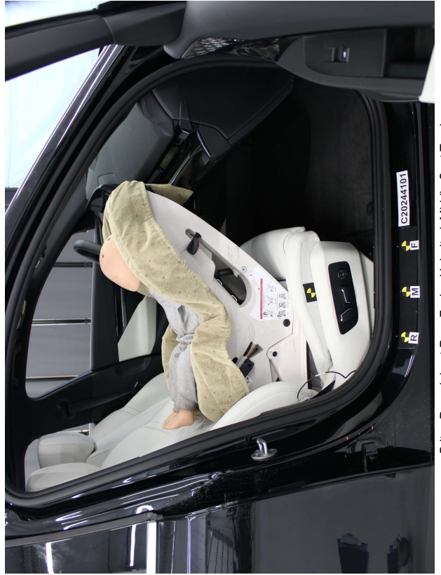
Britax Roundabout Rear Facing Unbelleted, Middle Seat Track
