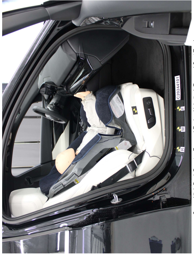
Cosco High Back Booster Forward Facing Unbelted, Forward Seat Track
