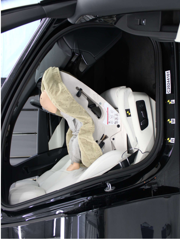
Britax Roundabout Rear Facing Unbelleted, Forward Seat Track
