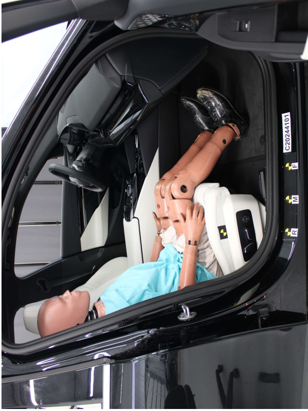
Unbelleted 5th Percentile Female Dummy Reactivation, Rearward Seat Track
