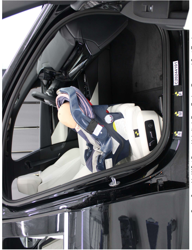
Graco Snugride WOut Base, Unbelted, Rear Facing, Rearward Seat Track
