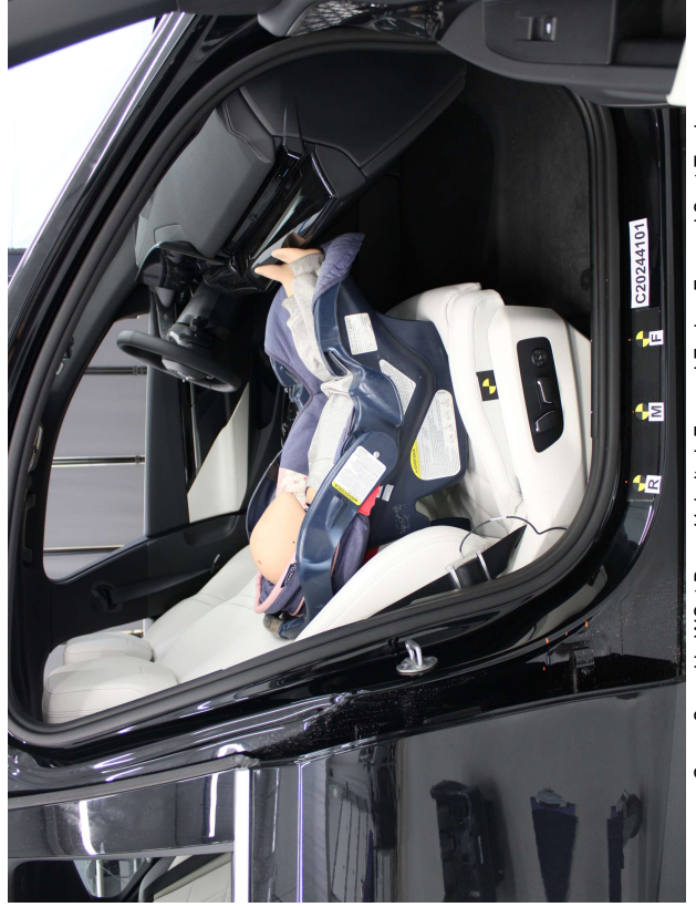
Graco Snugride WOut Base, Unbelted, Forward Facing, Forward Seat Track
