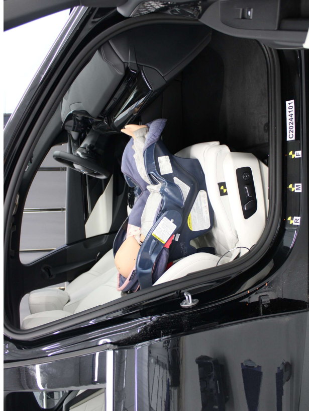
Graco Snugride WOut Base, Unbelleted, Forward Facing, Middle Seat Track
