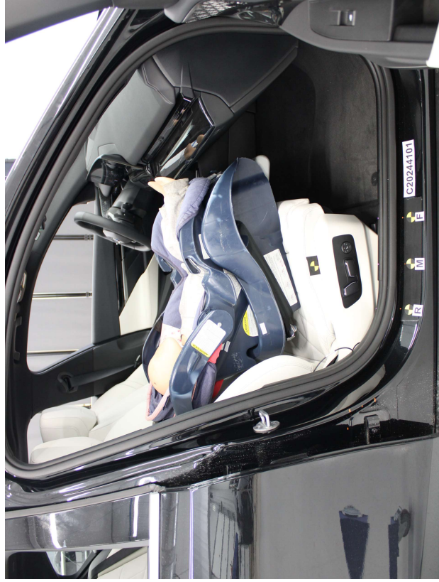
Graco Snugride WBBase, Unbelted, Forward Facing, Middle Seat Track
