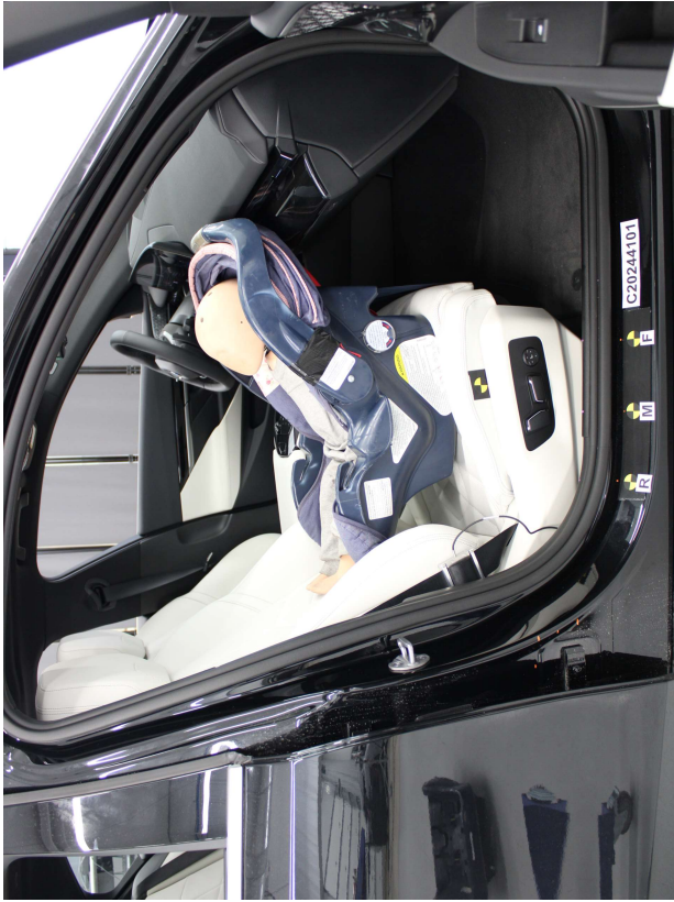
Graco Snugride WOut Base, Unbelted, Rear Facing, Forward Seat Track
