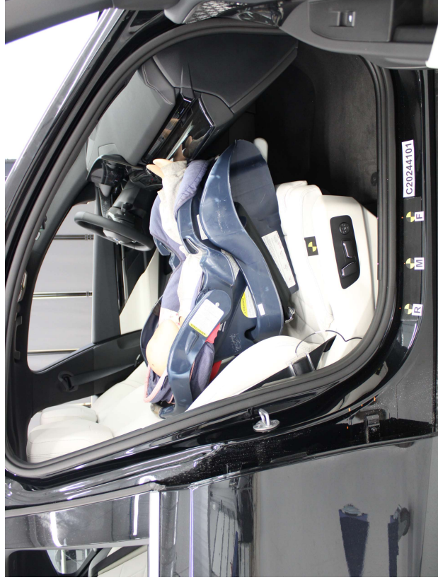
Graco Snugride WBBase, Unbelted, Forward Facing, Forward Seat Track
