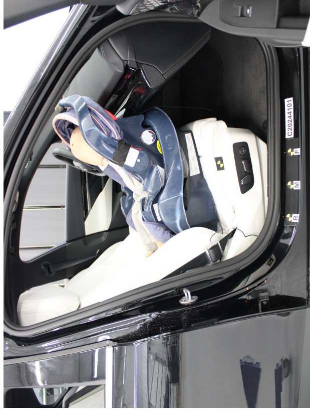
Graco Snuggly WBBase, Unbelted, Rear Facing, Forward Seat Track
