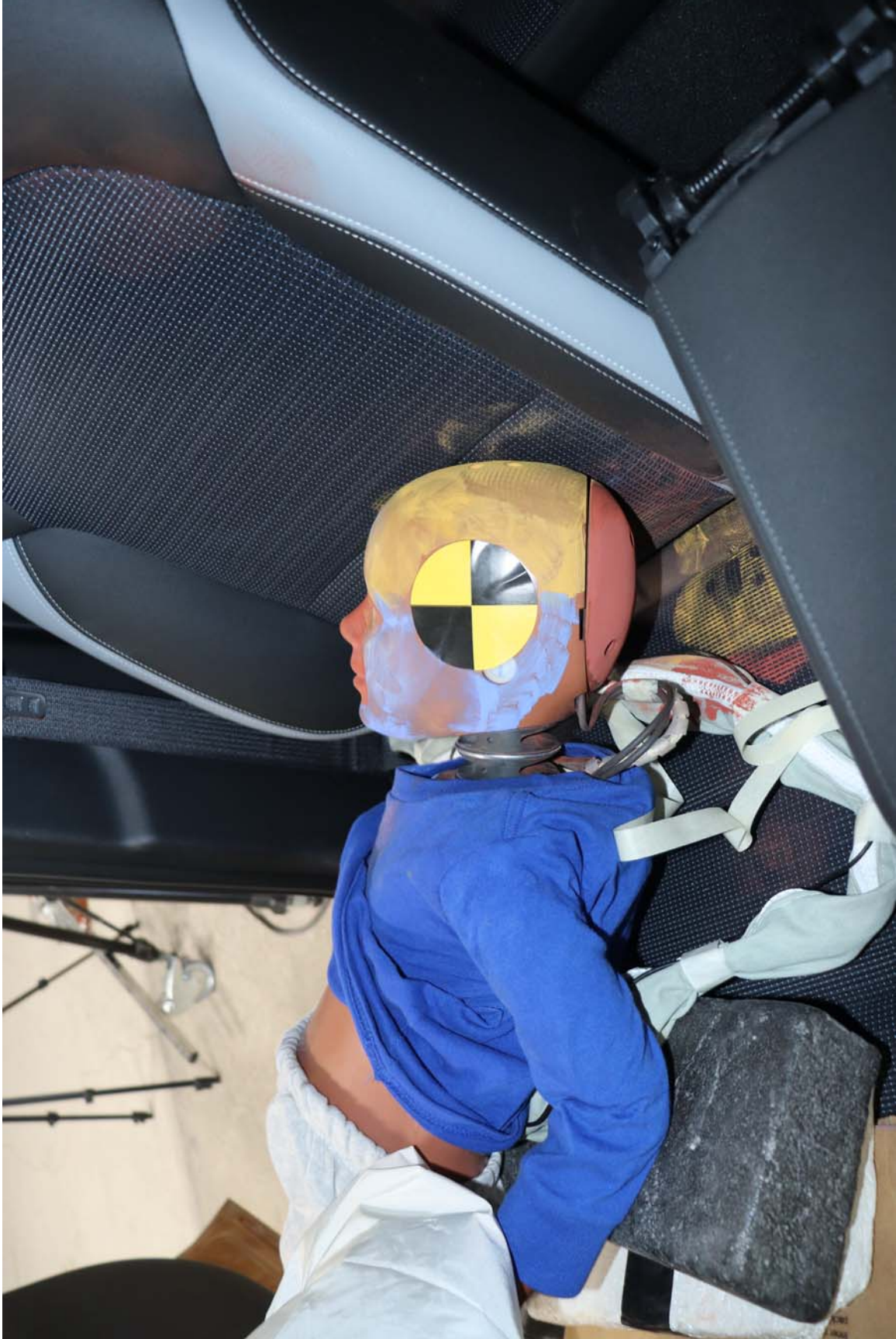
Photo No. 21 - Post-Test 3YO P1 Passenger Dummy Head Contact (seat back)
