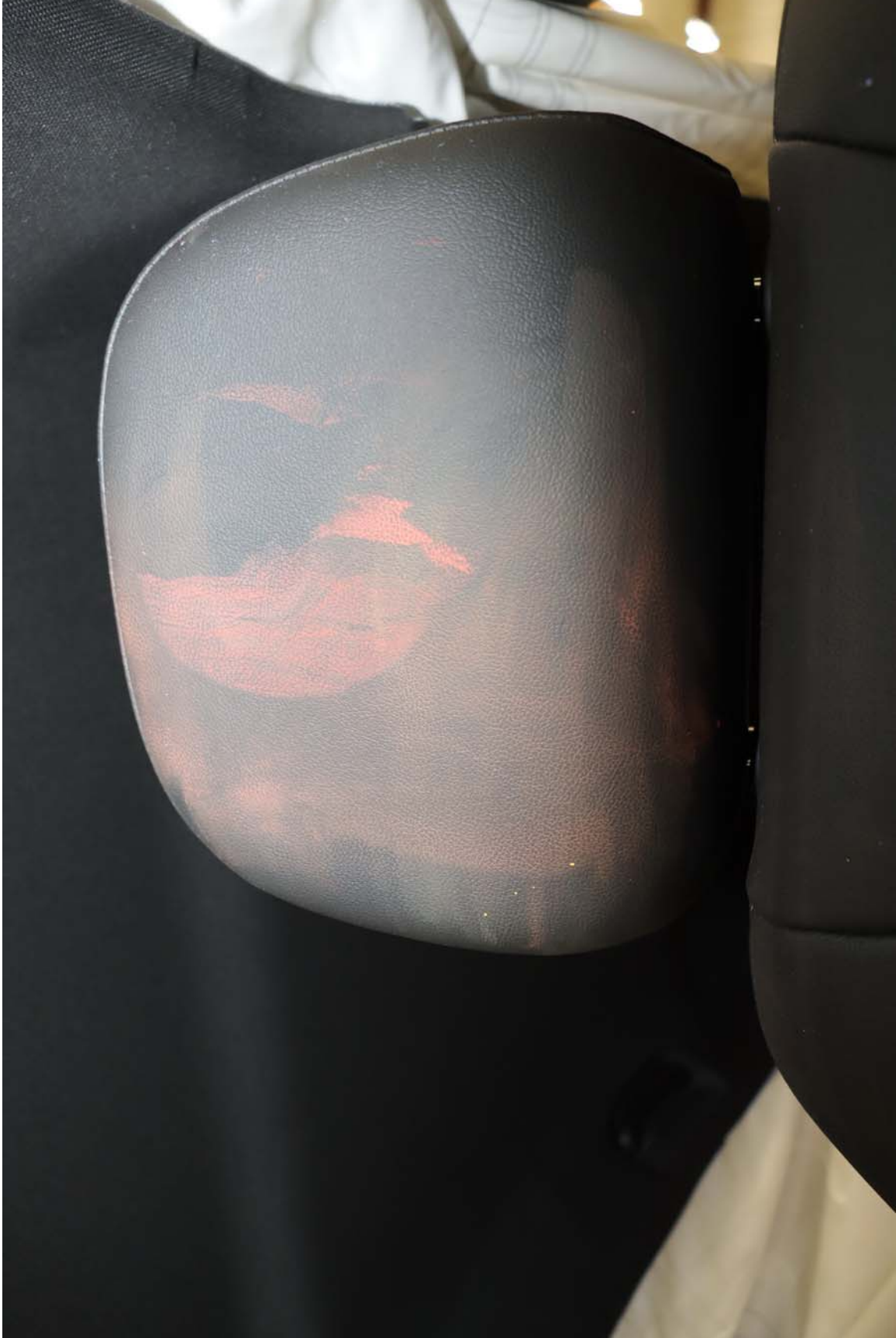
Photo No. 46. Post-Test Driver Dummy Head Contact (headrest)
