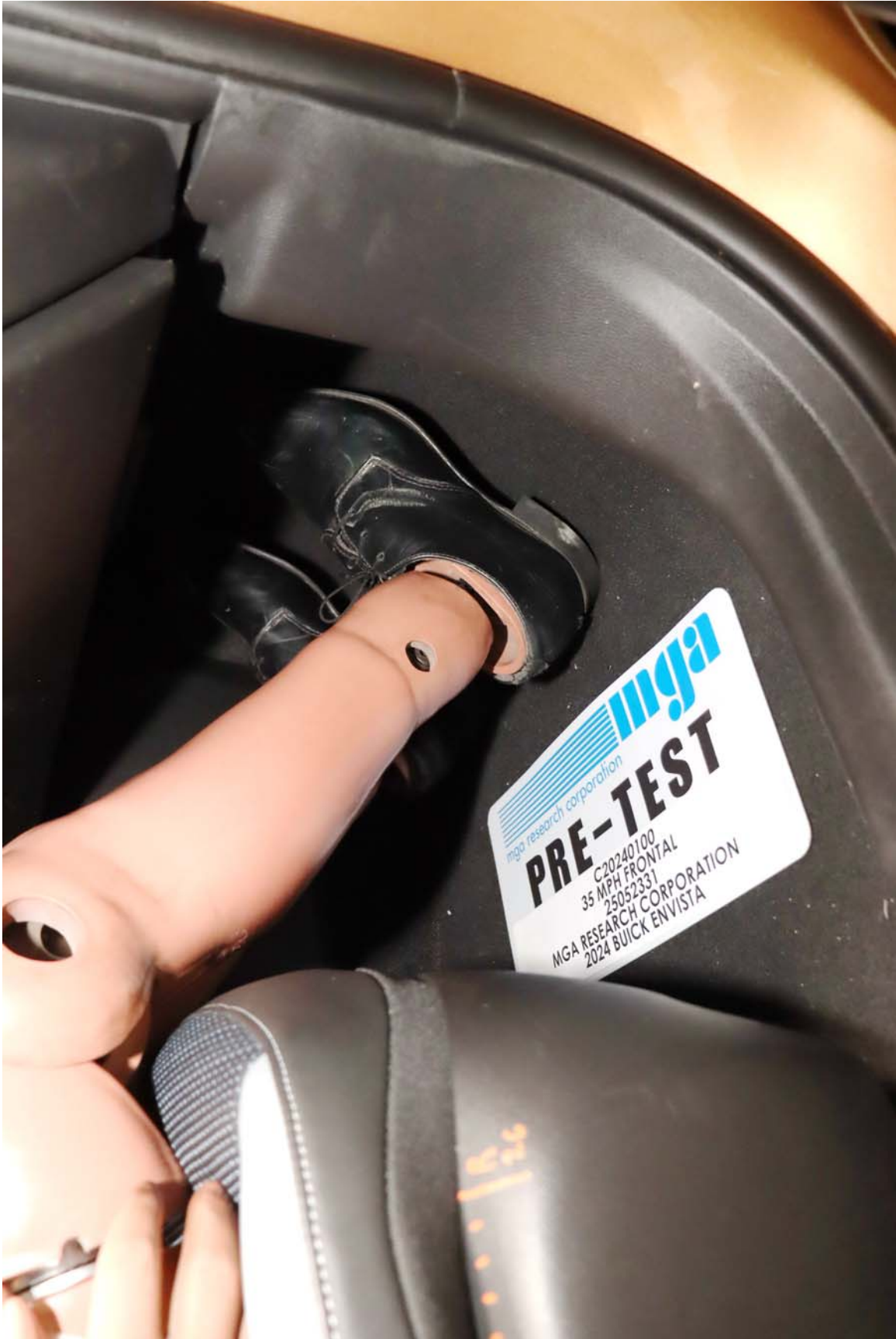
Photo No. 55. Pre-Test Passenger Dummy Feet Position
