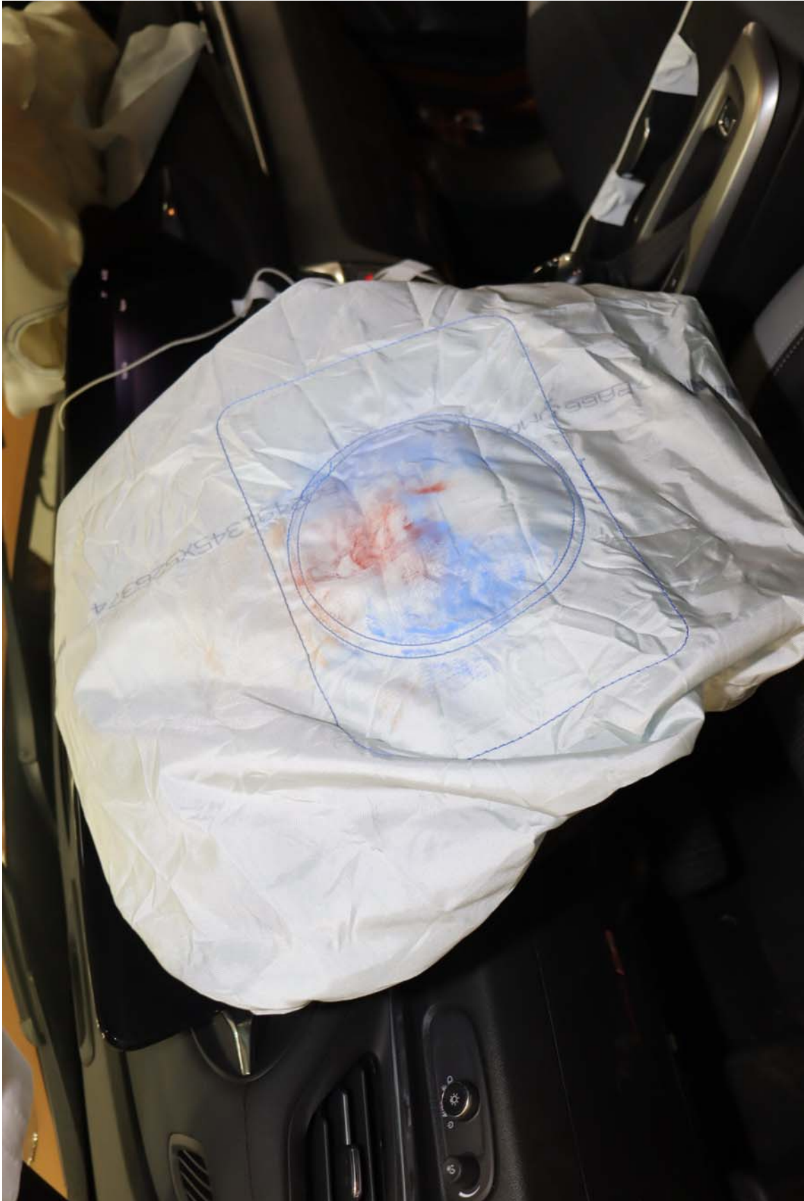
Photo No. 45. Post-Test Driver Dummy Airbag Contact
