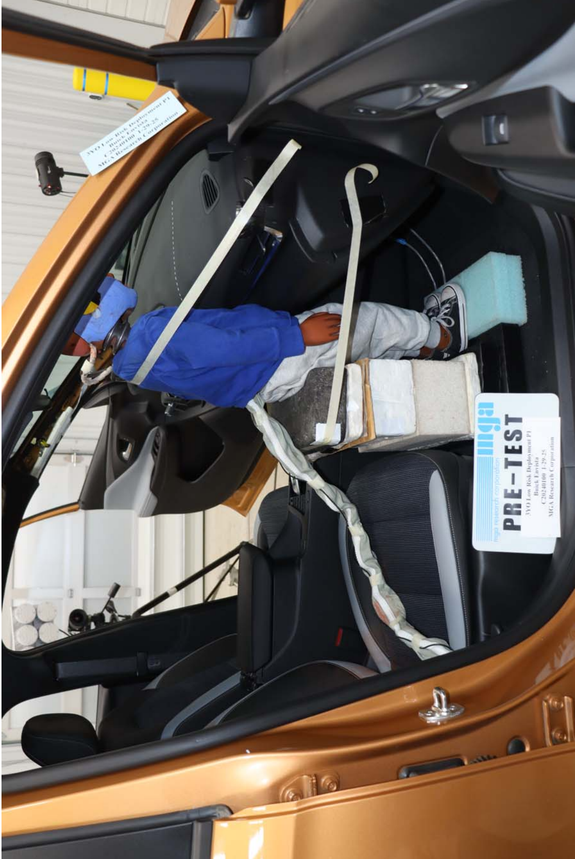
Photo No. 17 - Pre-Test 3YO P1 Passenger Dummy Right Side View
