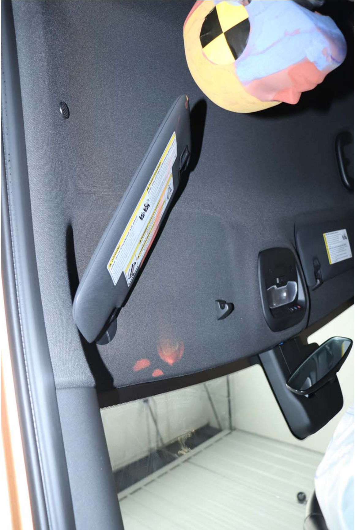
Photo No. 14 - Post-Test 5th Fem. P2 Driver Dummy Head Contact (visor-header)
