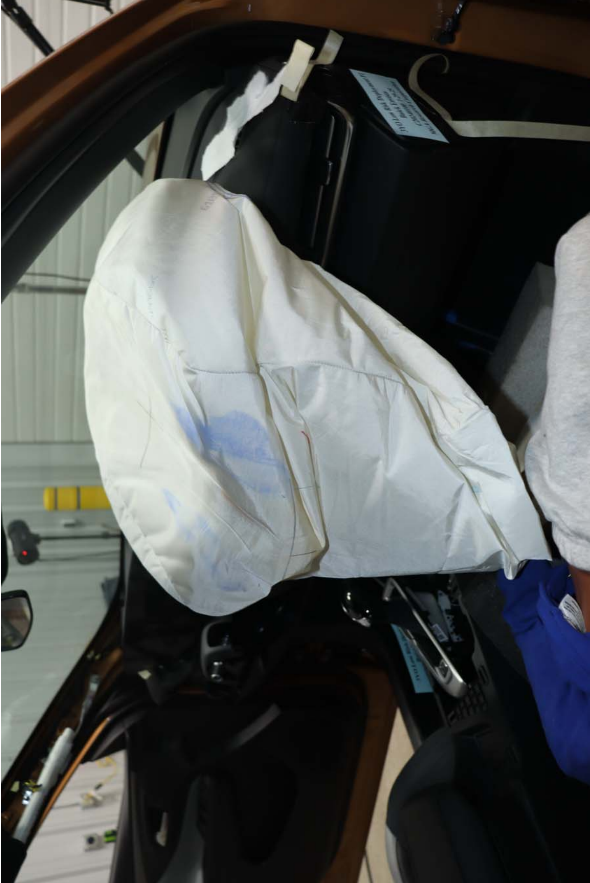
Photo No. 20 - Post-Test 3YO P1 Passenger Dummy Airbag Right Side View
