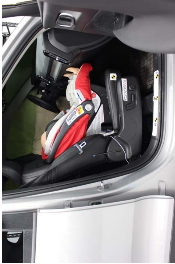
Peg Perego Viaggio WOut Base, Unbelleted, Forward Facing, Forward Seat Track
