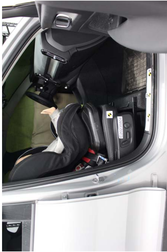
Graco Toddler SafeSeat Step 2 Forward Facing Belted, Rearward Seat Track
