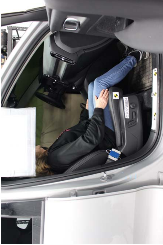
Unbelleted 5th Percentile Female Human Reactivation, Middle Seat Track
