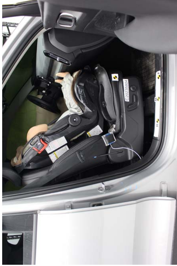
Cosco Summit Deluxe Forward Facing Unbelted, Forward Seat Track
