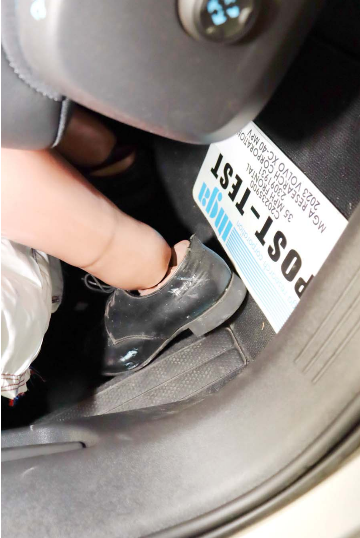
Photo No. 40 - Post-Test Driver Dummy Feet Position
