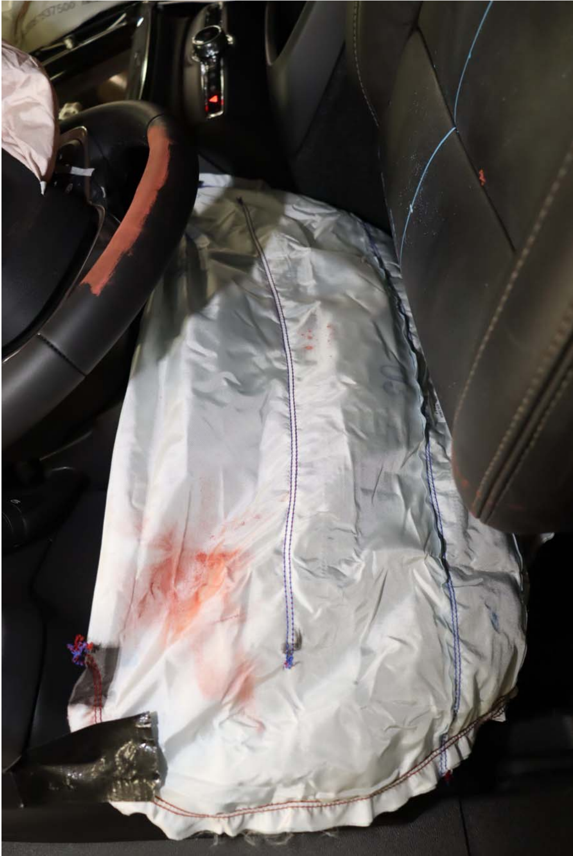
Photo No. 44 - Post-Test Driver Dummy Knee Contact
