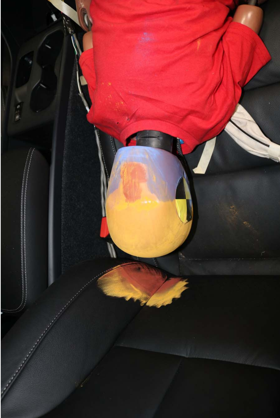
Photo No. 34 - Post-Test 6YO P1 Passenger Dummy Head Contact (seat)
