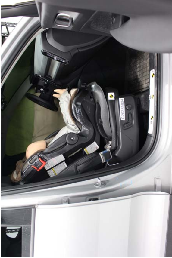
Cosco Summit Deluxe Forward Facing Unbelted, Middle Seat Track
