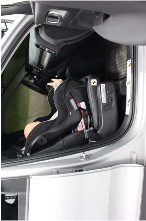
Evenflo Tribute Forward Facing Unbelleted, Middle Seat Track
