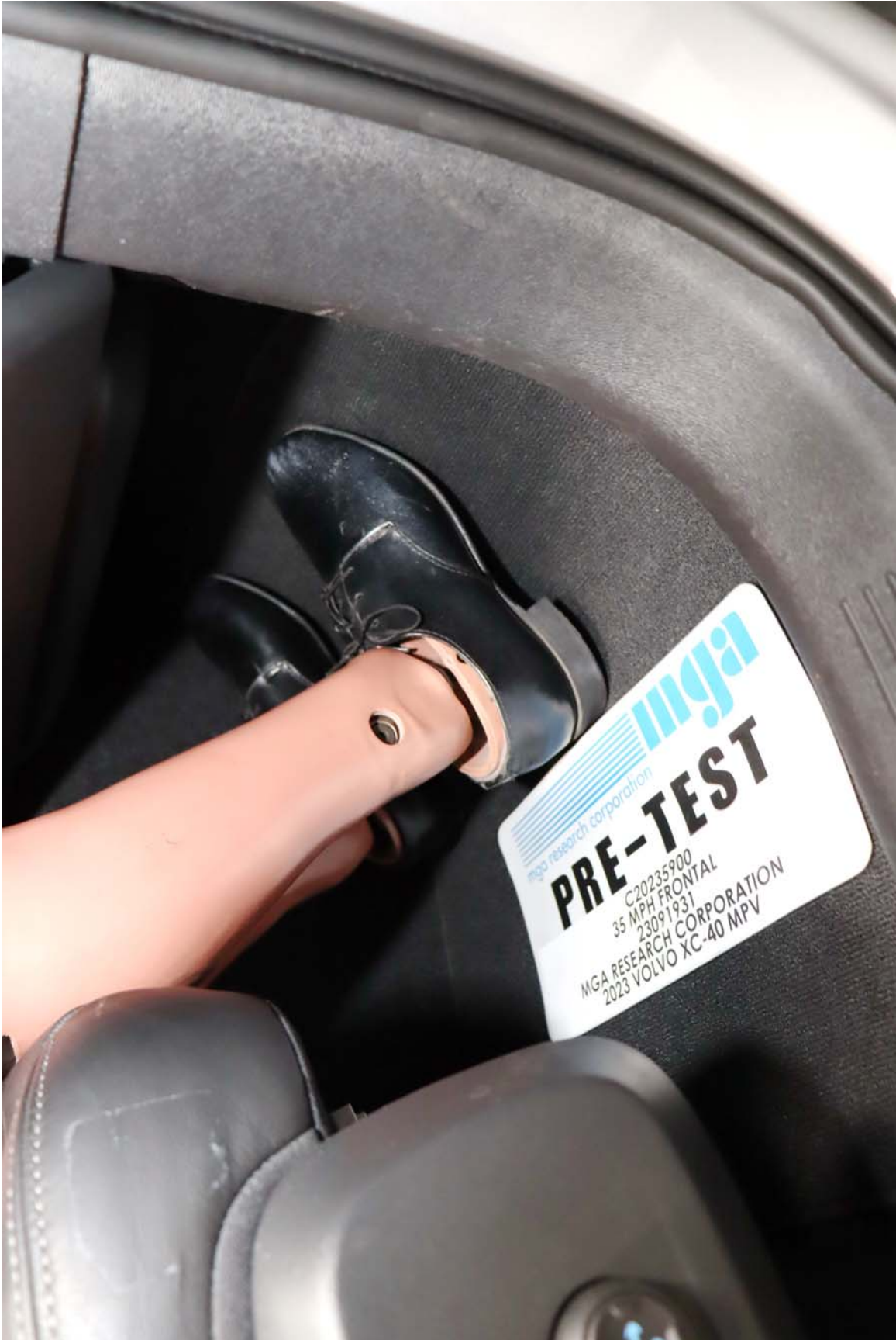
Photo No. 54 - Pre-Test Passenger Dummy Feet Position
