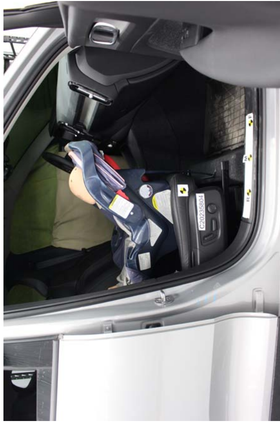
Graco Snugride WOut Base, Unbelted, Rear Facing, Rearward Seat Track
