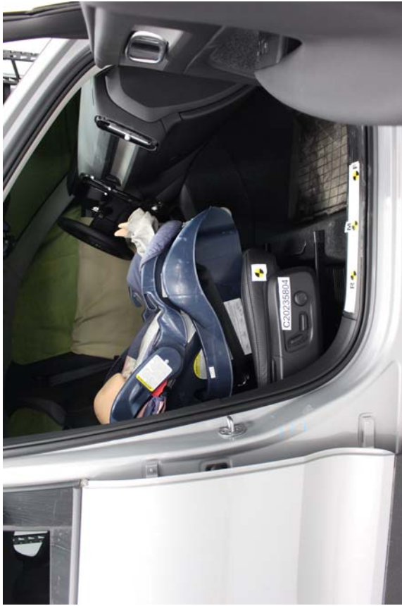
Graco Snugride WB Base, Unbelted, Forward Facing, Rearward Seat Track
