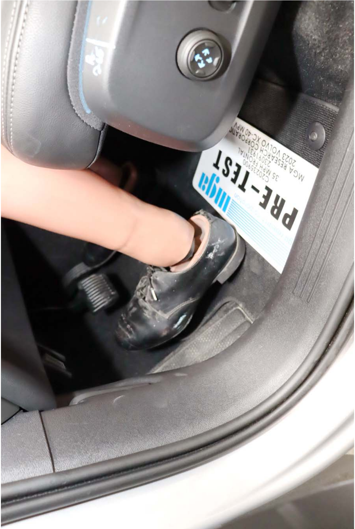
Photo No. 39 - Pre-Test Driver Dummy Feet Position
