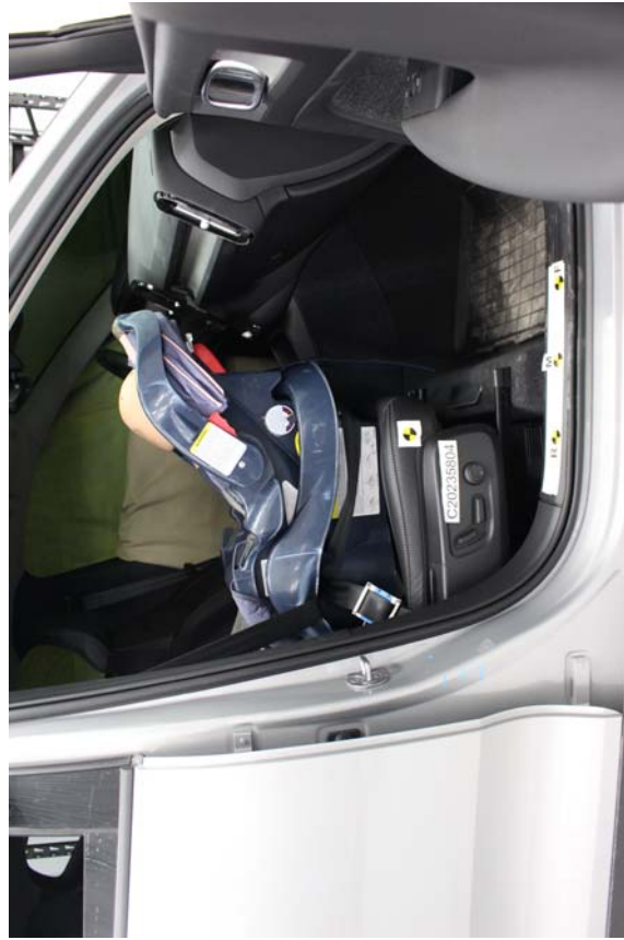
Graco Snugride WBBase, Belted, Rear Facing, Rearward Seat Track
