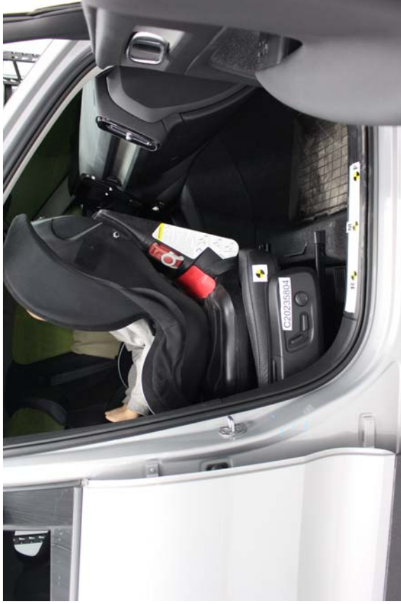
Graco Toddler SafeSeat Step 2 Rear Facing Unbelleted, Rearward Seat Track
