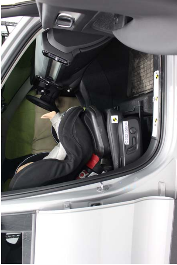
Graco Toddler SafeSeat Step 2 Forward Facing Unbelted, Rearward Seat Track
