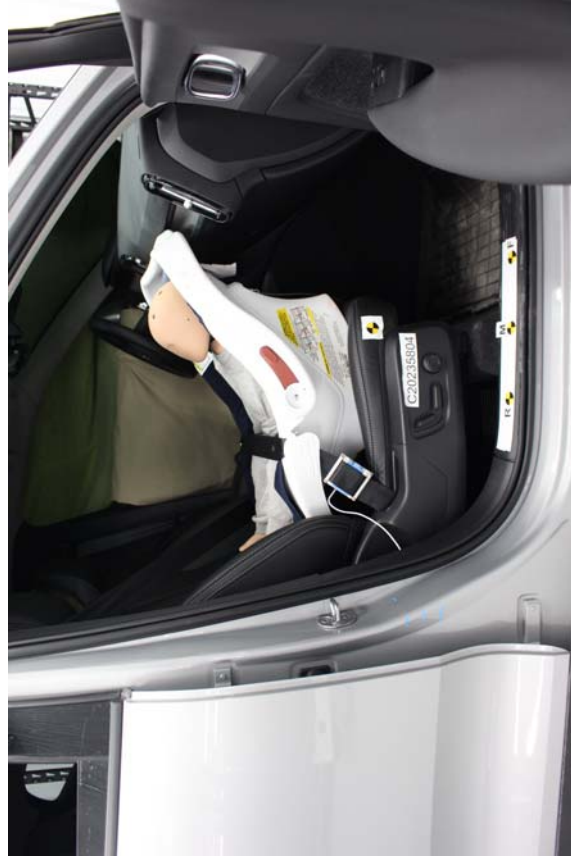
Cosco Arriva WOut Base, Belleted, Rear Facing, Middle Seat Track
