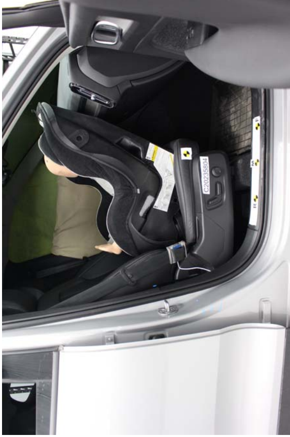
Evenflo Tribute Rear Facing Unbelleted, Forward Seat Track
