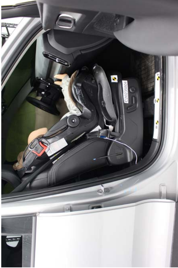
Cosco Summit Deluxe Forward Facing Belted, Forward Seat Track
