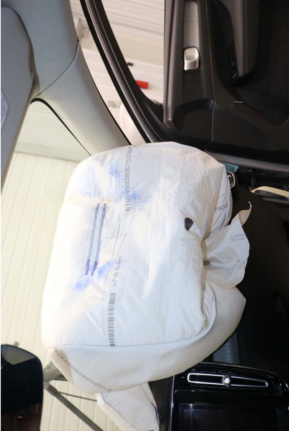
Photo No. 18 - Post-Test 3YO P1 Passenger Dummy Airbag Left Side View
