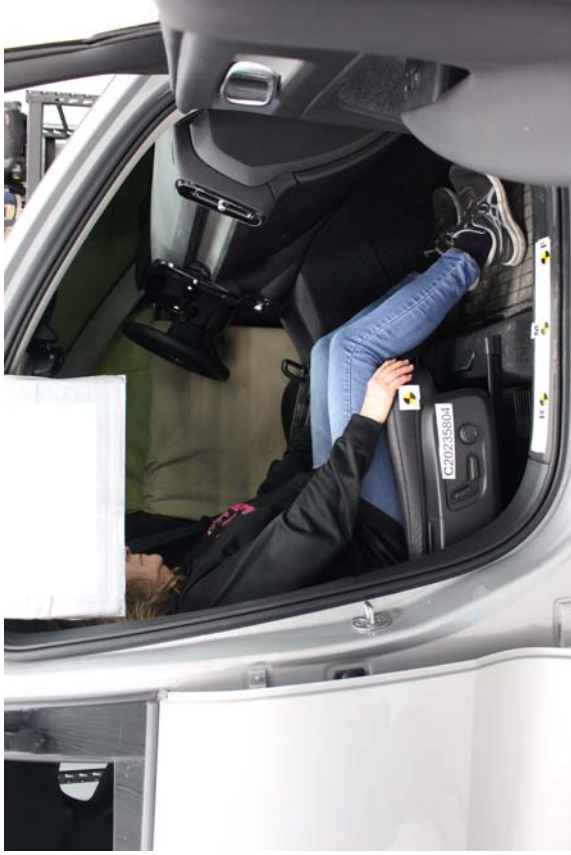
Unbelleted 5th Percentile Female Human Reactivation, Rearward Seat Track
