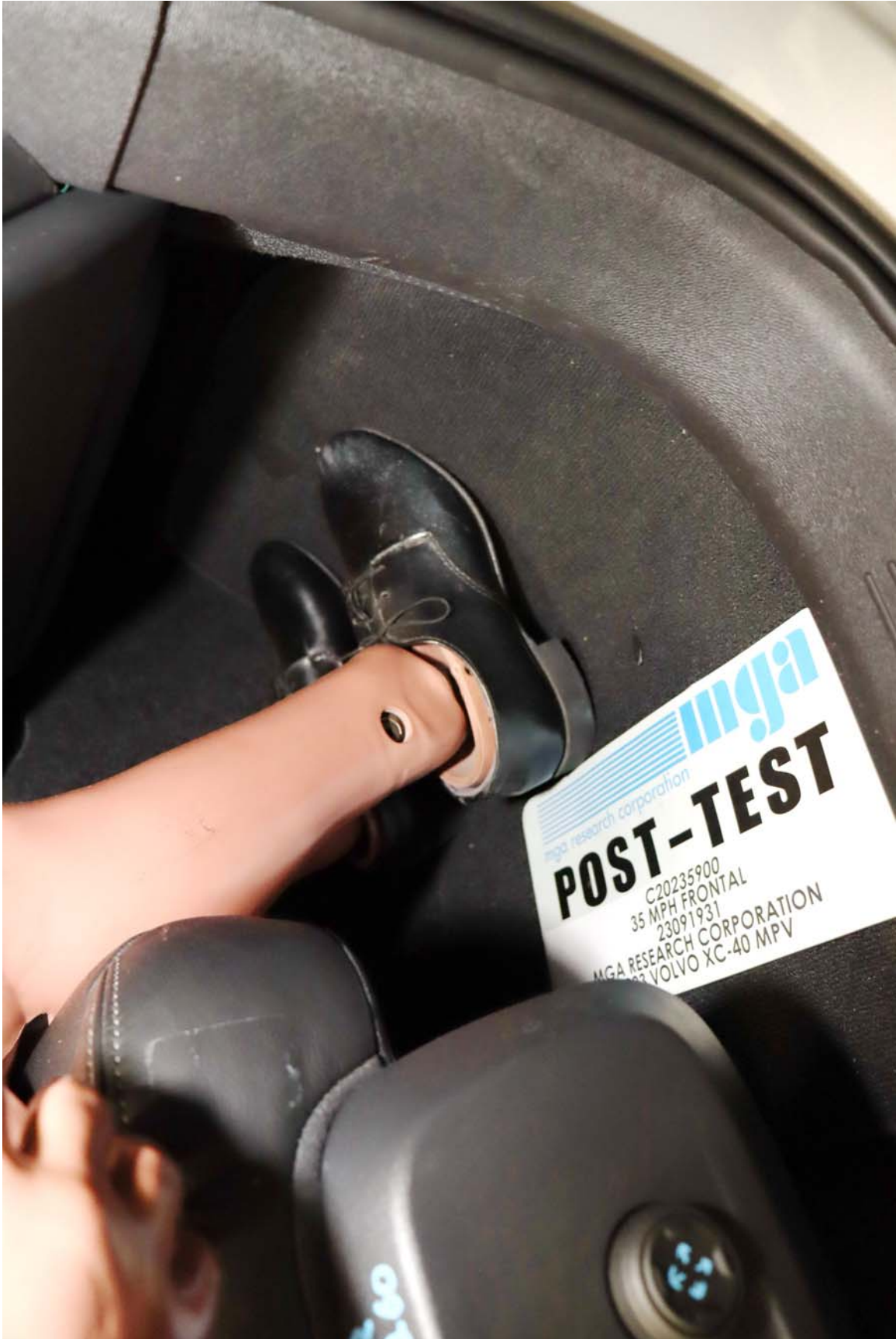
Photo No. 55 - Post-Test Passenger Dummy Feet Position
