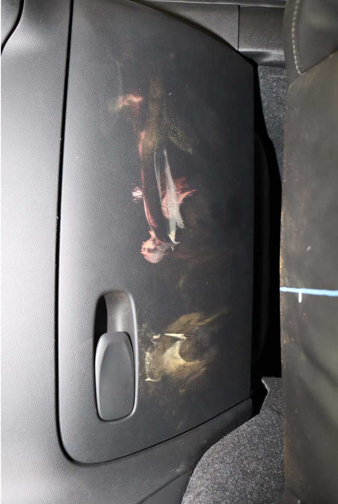
Photo No. 59 - Post-Test Passenger Dummy Knee Contact
