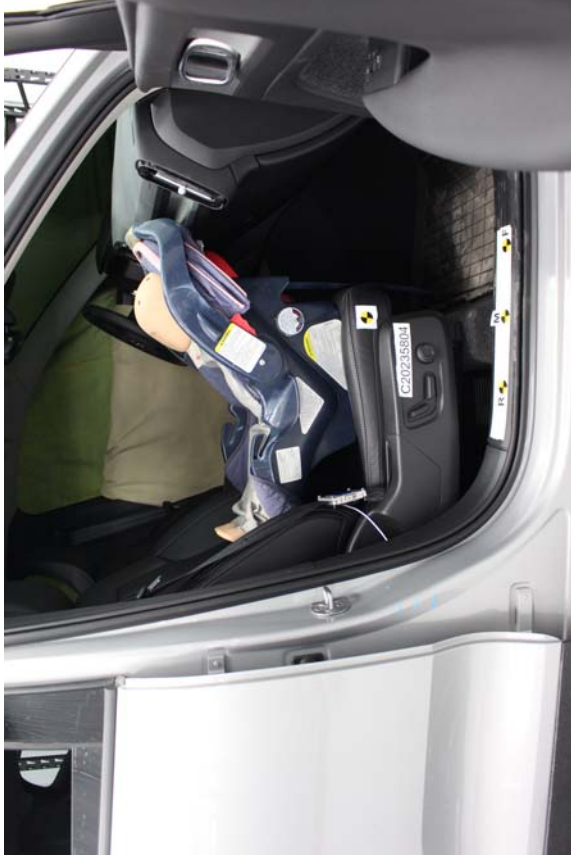
Graco Snugride WOut Base, Unbelted, Rear Facing, Middle Seat Track
