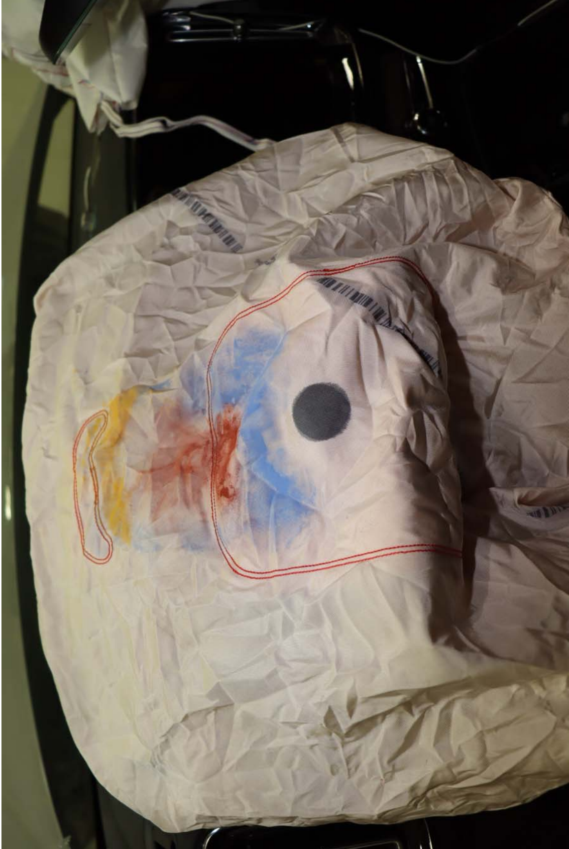
Photo No. 43 - Post-Test Driver Dummy Airbag Contact
