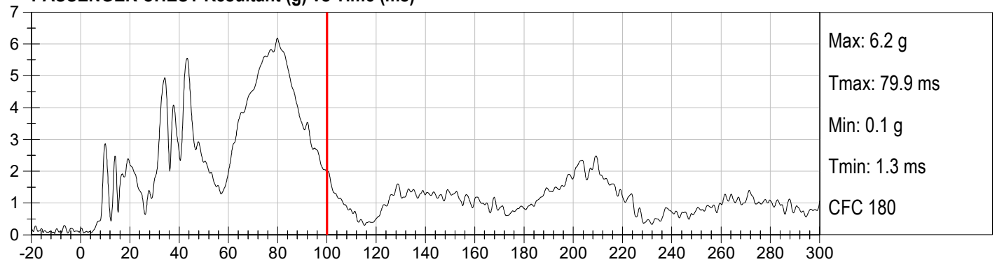
PASSENGER CHEST Resultant (g) vs Time (ms)
