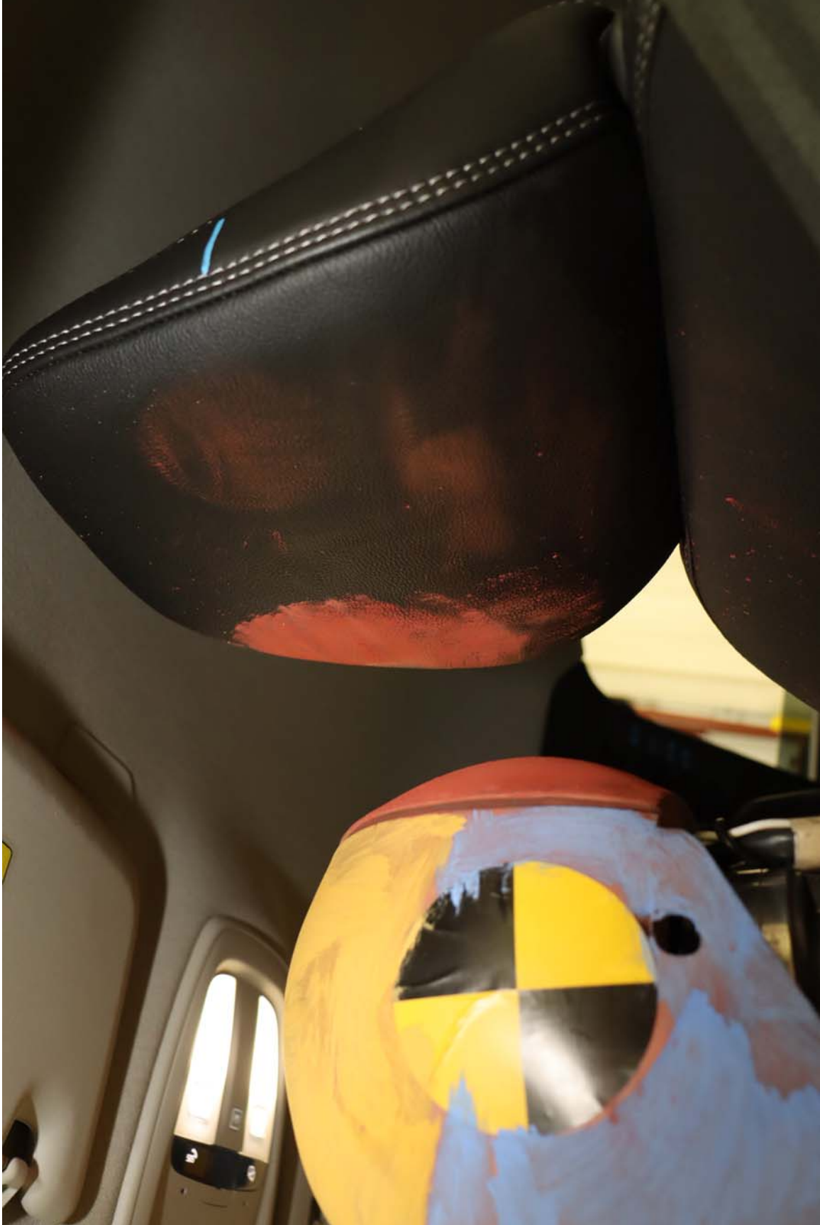
Photo No. 45 - Post-Test Driver Dummy Head Contact (headrest)
