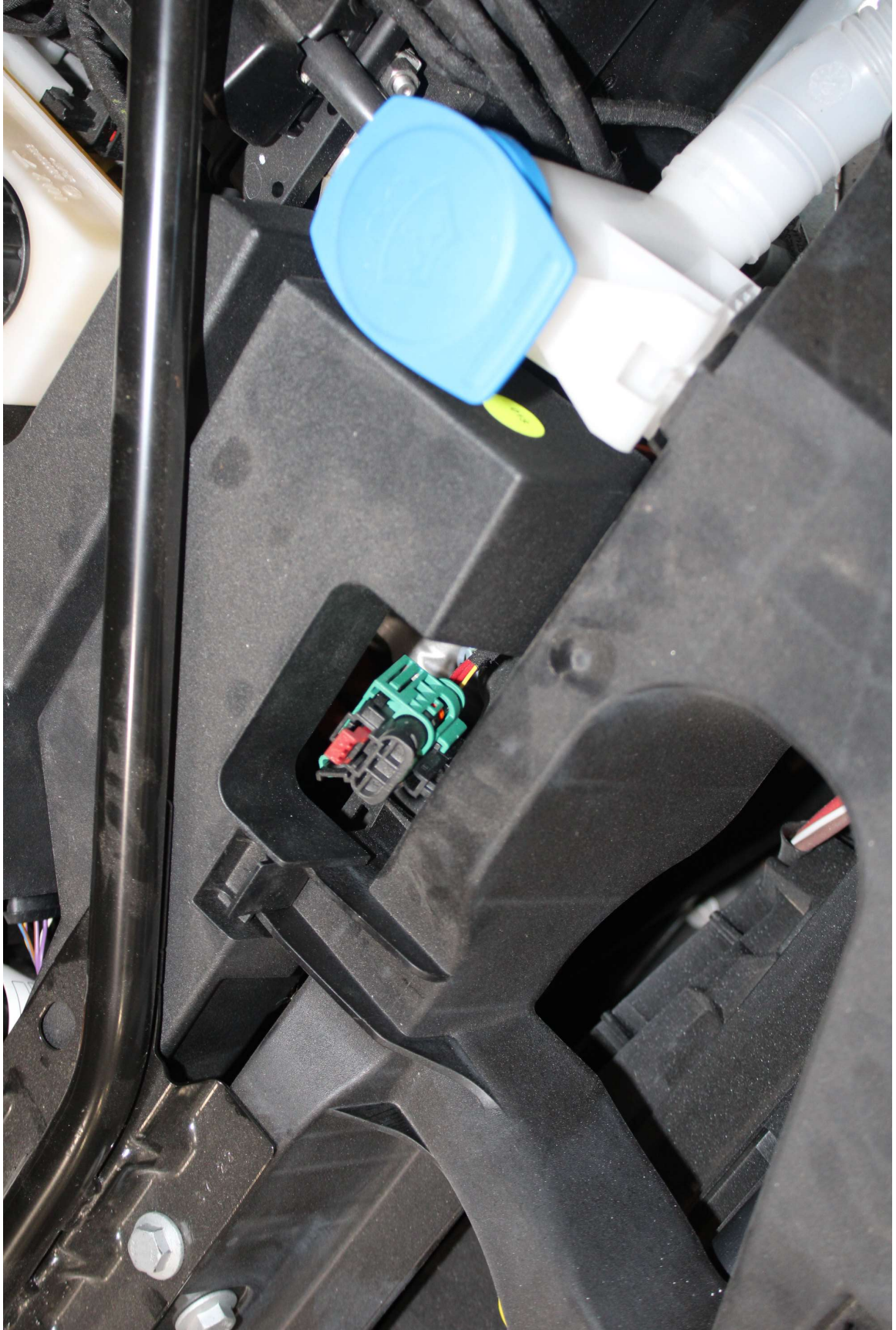
Photo No. 69. Pre-Test Manual Service Disconnect Removed
