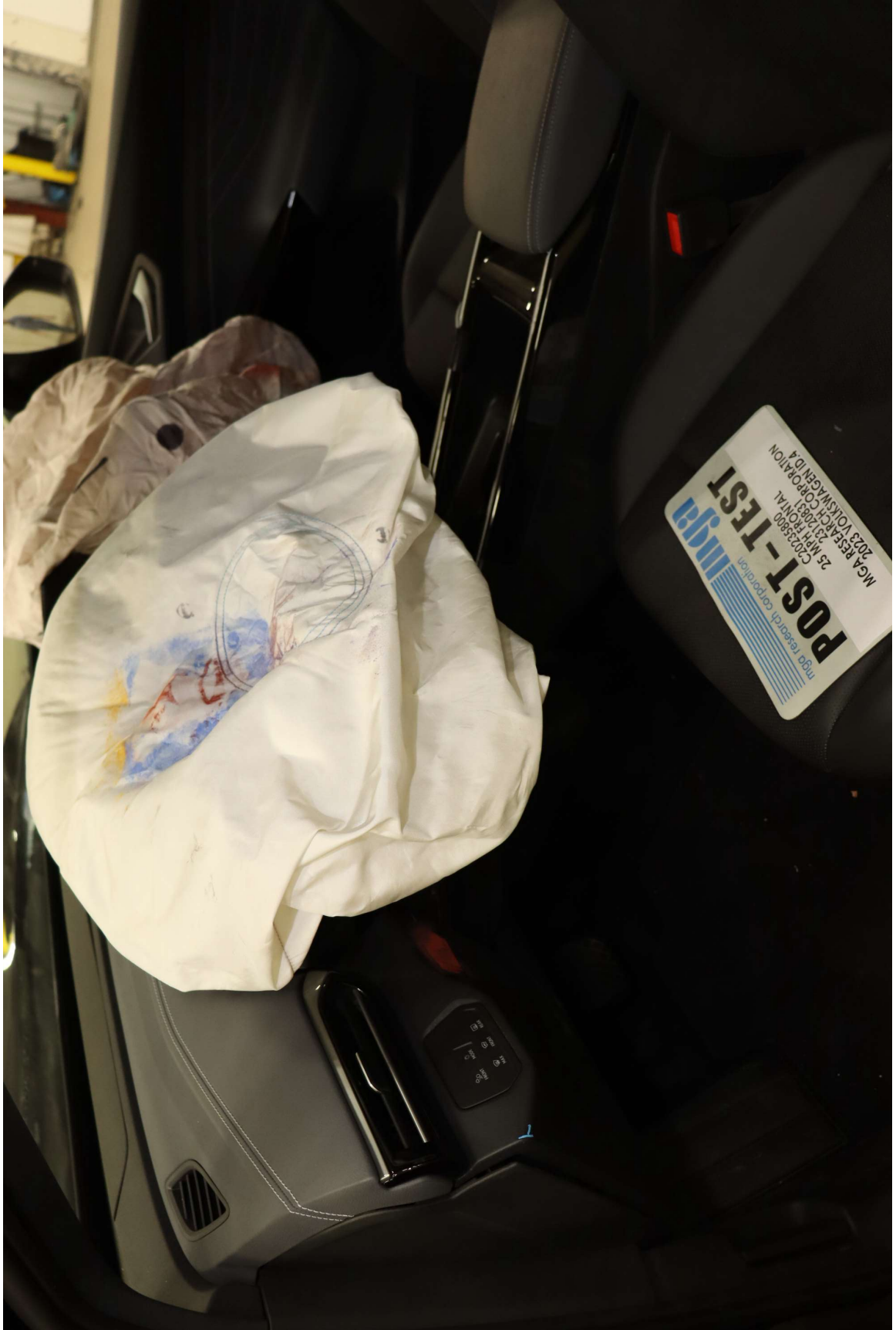
Photo No. 45. Post-Test Driver Dummy Airbag Contact
