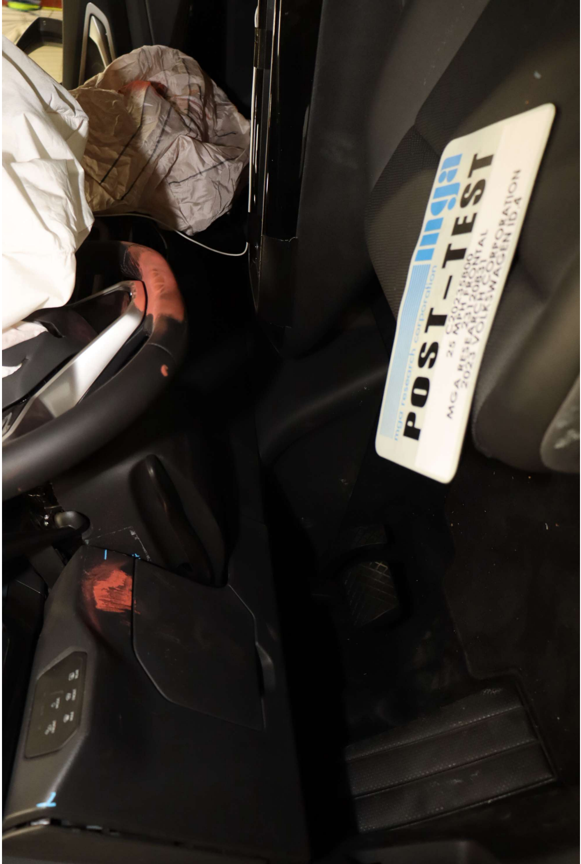
Photo No. 46. Post-Test Driver Dummy Knee Contact
