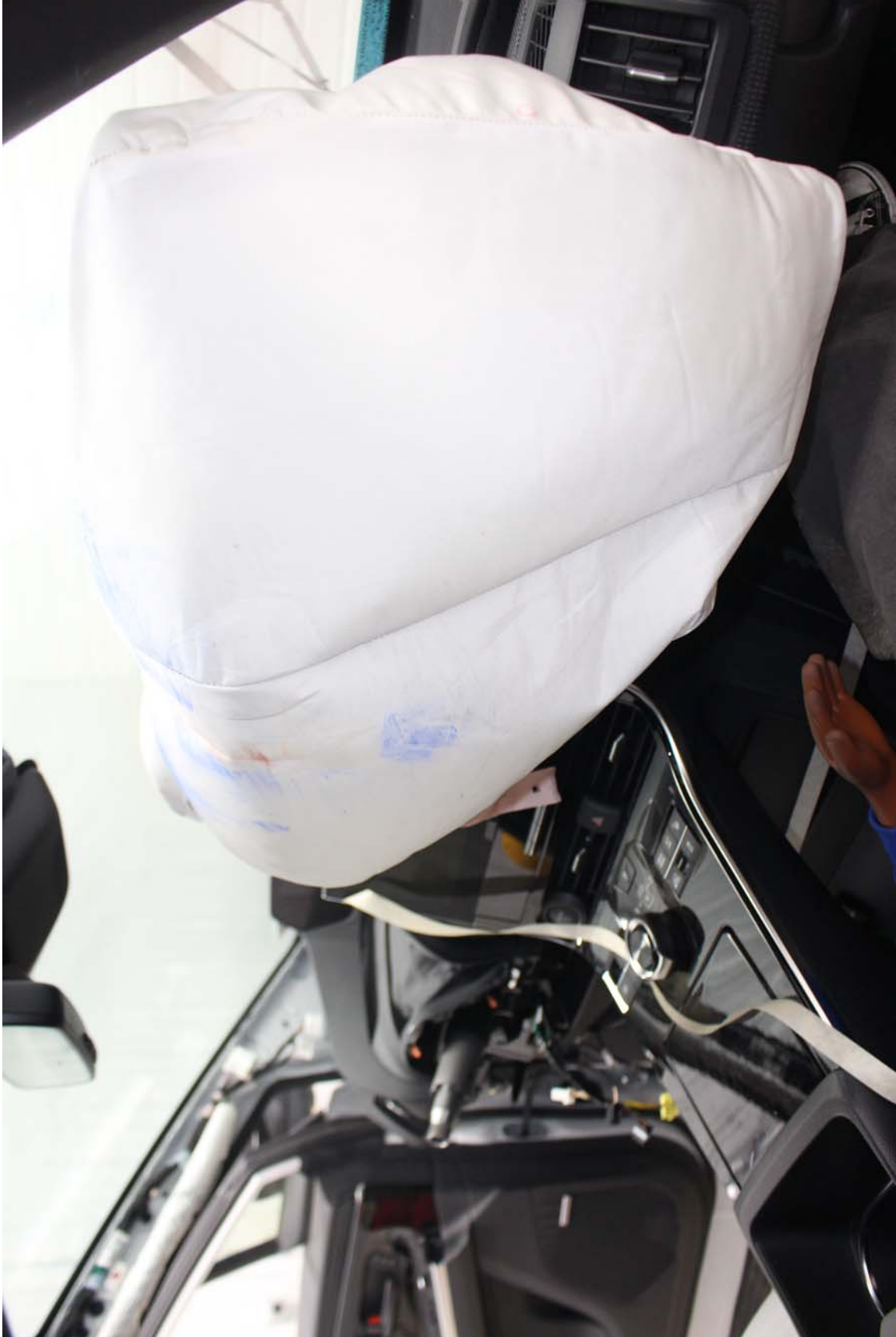
Photo No. 19 - Post-Test 3YO P1 Passenger Dummy Airbag Right Side View
