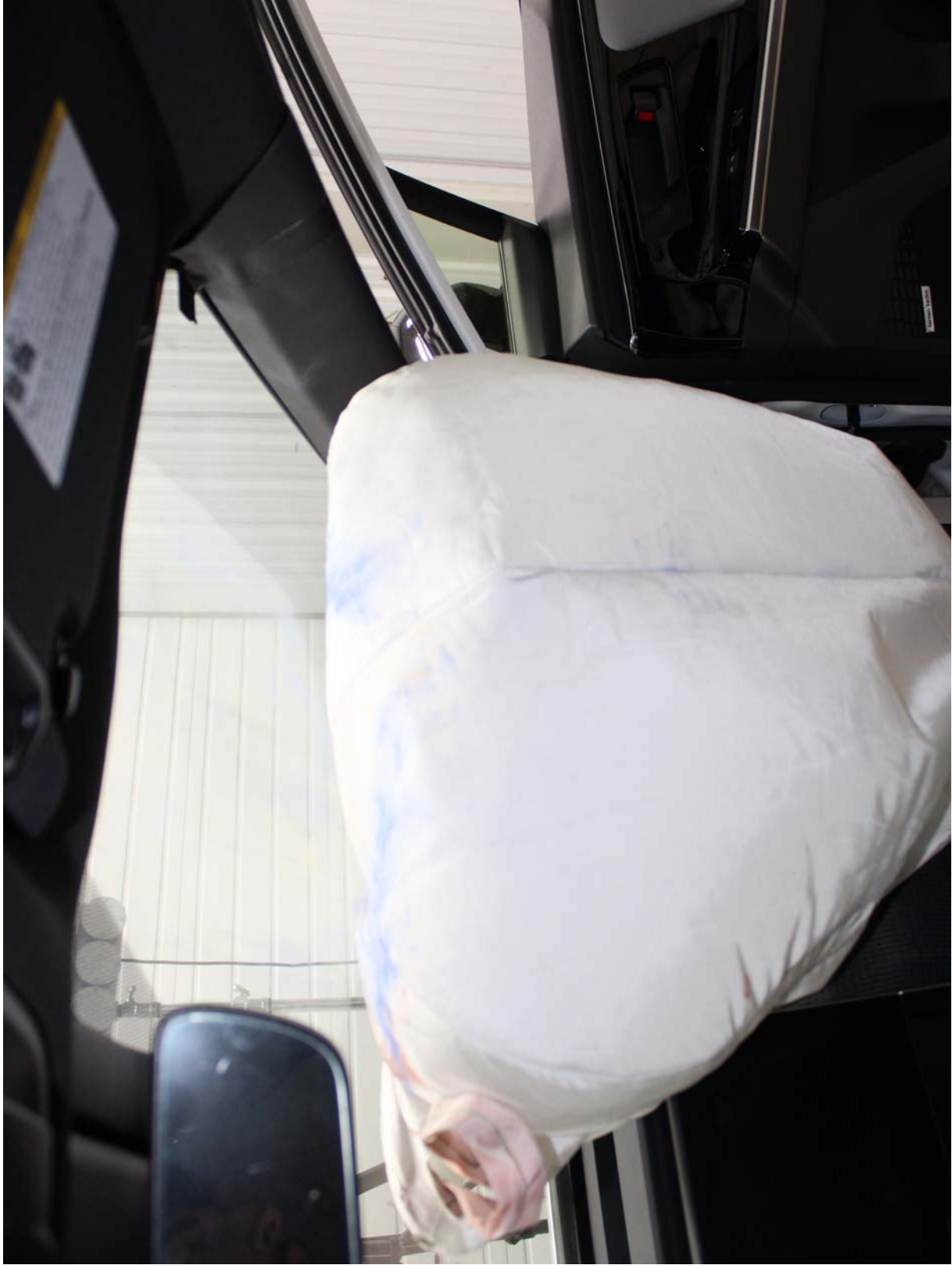
Photo No. 39 - Post-Test 6YO P1 Passenger Dummy Airbag Left Side View
