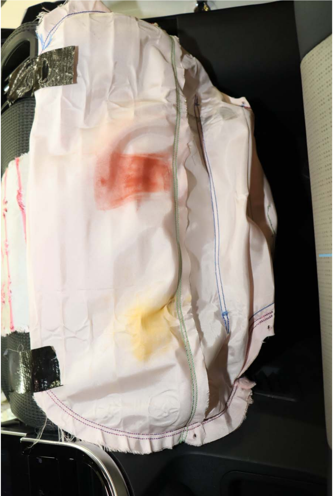
Photo No. 61. Post-Test Passenger Dummy Knee Contact
