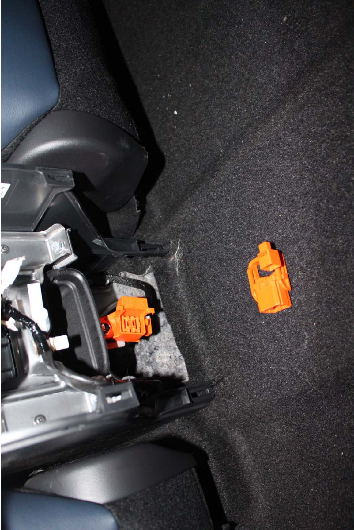
Photo No. 71. Pre-Test Manual Service Disconnect Removed
