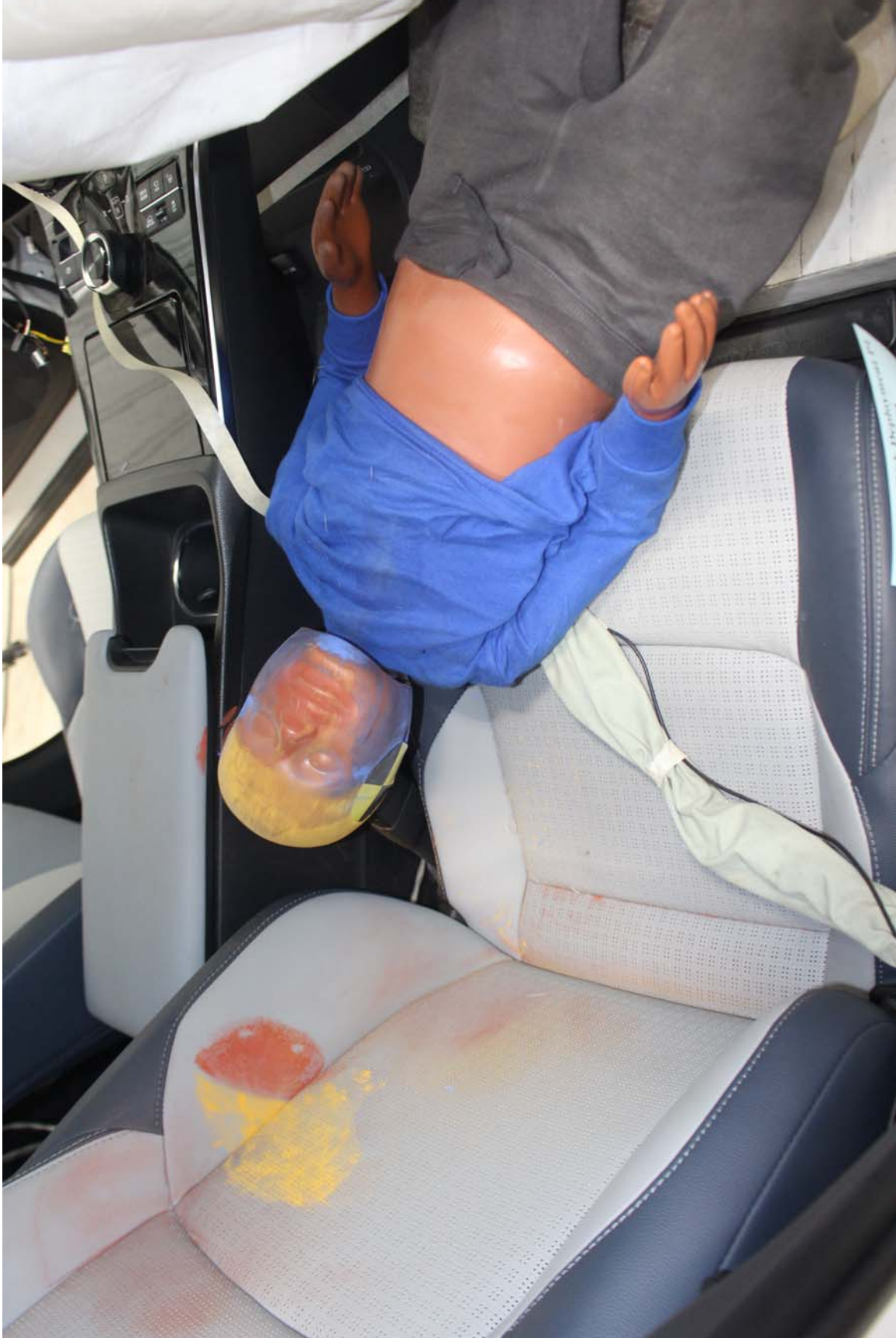
Photo No. 20 - Post-Test 3YO P1 Passenger Dummy Head Contact (seat)
