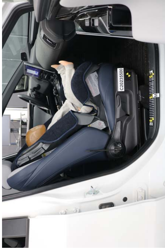
Cosco High Back Booster Forward Facing Unbelted, Forward Seat Track
