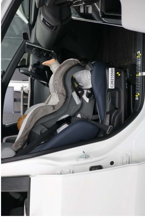
Graco Comfordsport Forward Facing Belted, Middle Seat Track
