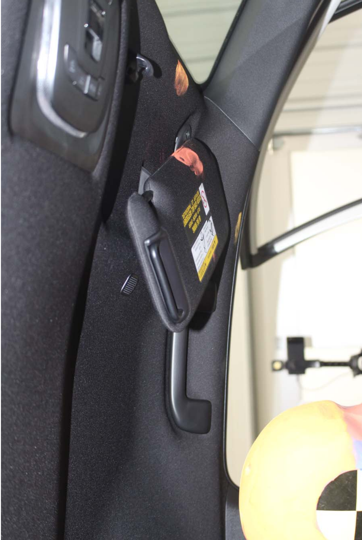
Photo No. 13 - Post-Test 5th Fem. P2 Driver Dummy Head Contact (visor)
