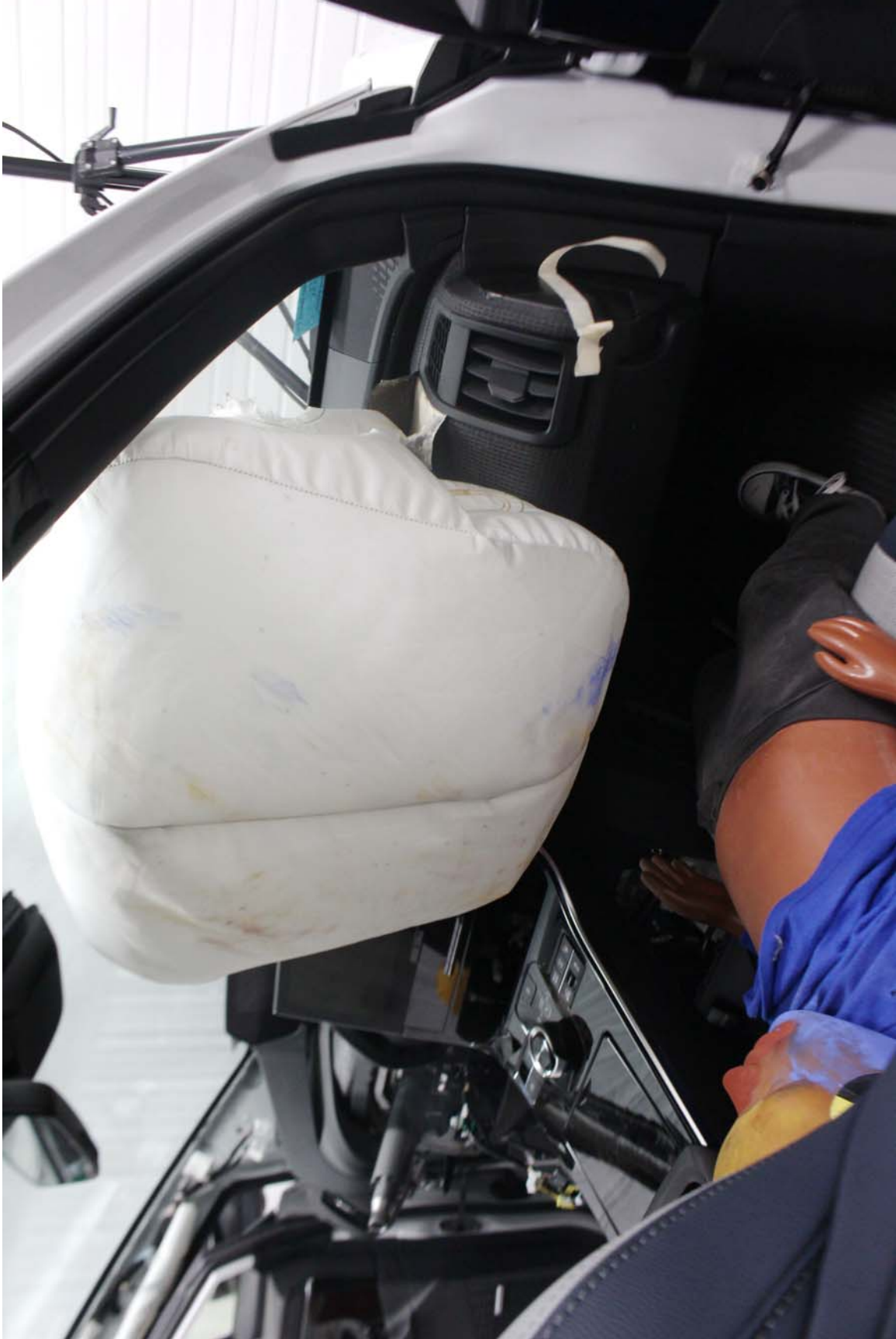
Photo No. 33 - Post-Test 3YO P2 TRIAL 2 Passenger Dummy Airbag Right Side View
