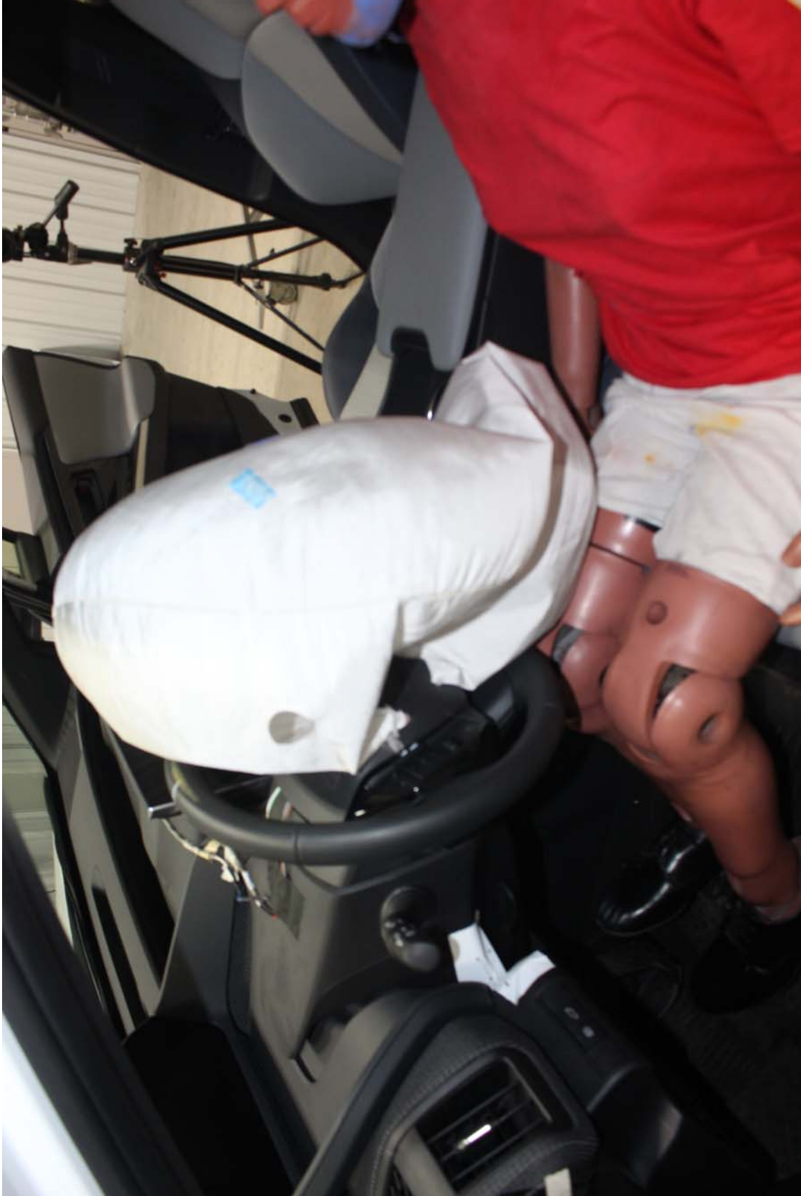
Photo No. 5 - Post-Test 5th Fem. P1 Driver Dummy Airbag Left Side View
