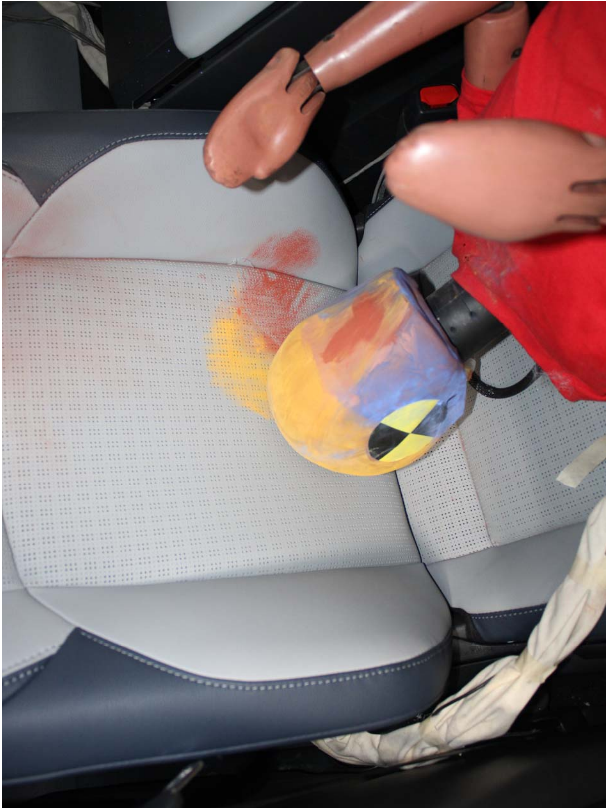
Photo No. 41 - Post-Test 6YO P1 Passenger Dummy Head Contact (seat)
