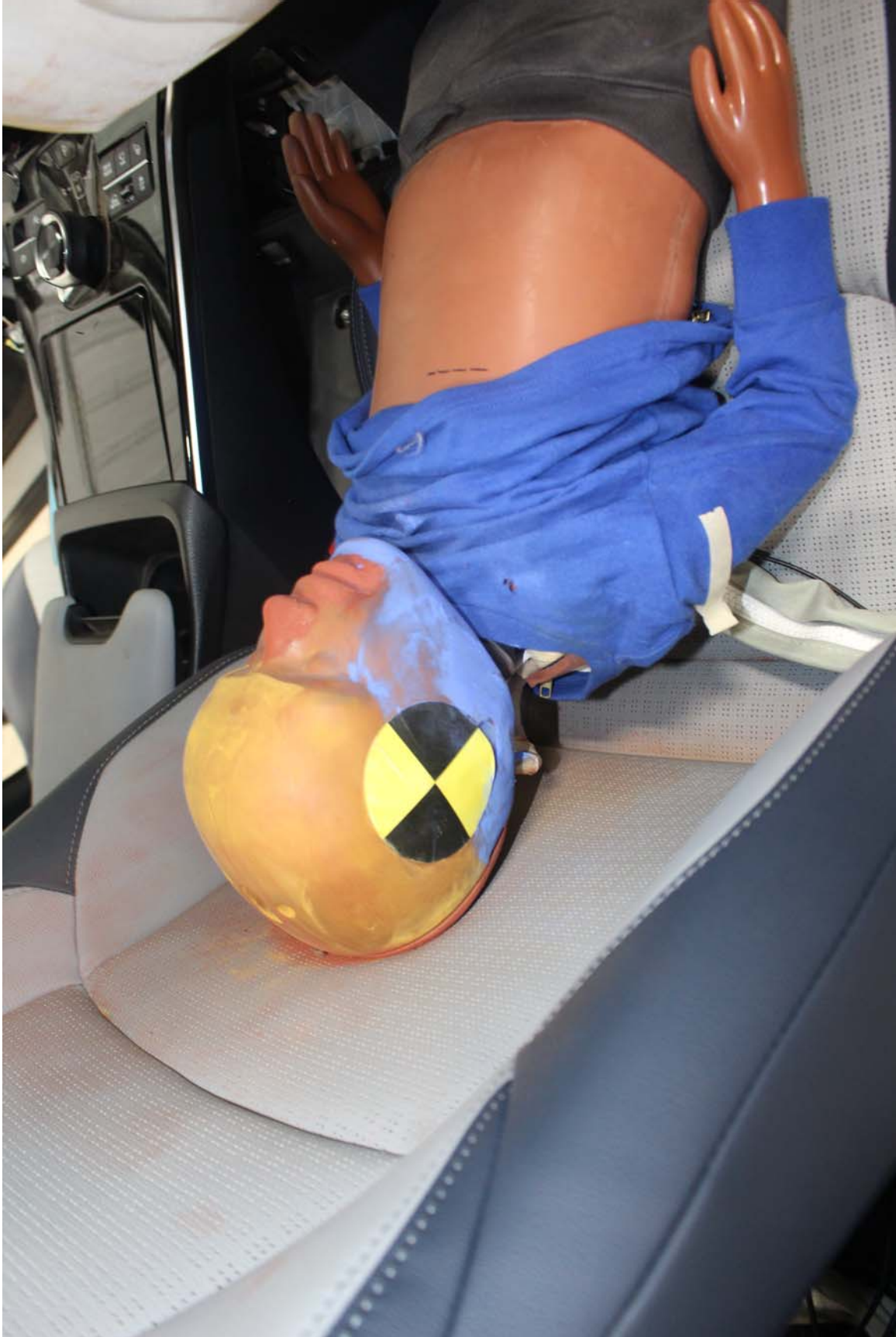
Photo No. 34 - Post-Test 3YO P2 TRIAL 2 Passenger Dummy Head Contact (seat back)
