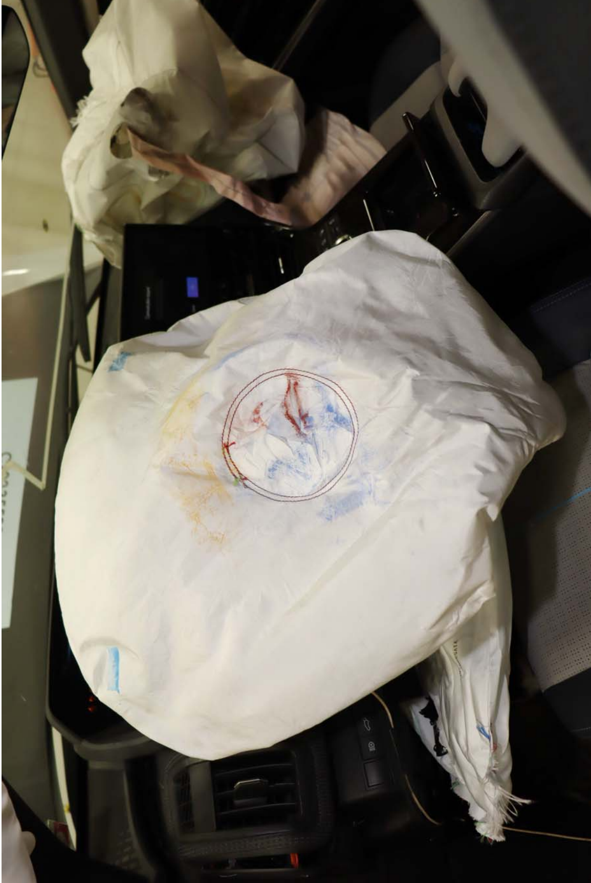
Photo No. 45. Post-Test Driver Dummy Airbag Contact
