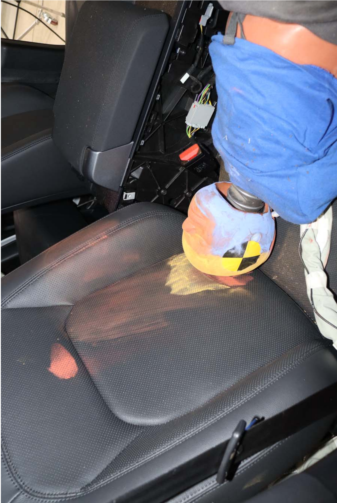
Photo No. 21 - Post-Test 3YO P1 Passenger Dummy Head Contact (seat)
