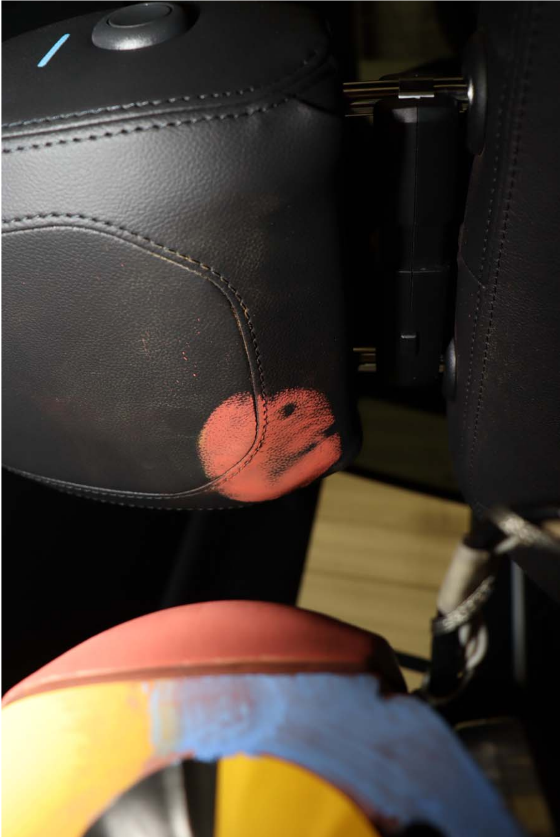
Photo No. 48. Post-Test Driver Dummy Head Contact (headrest)
