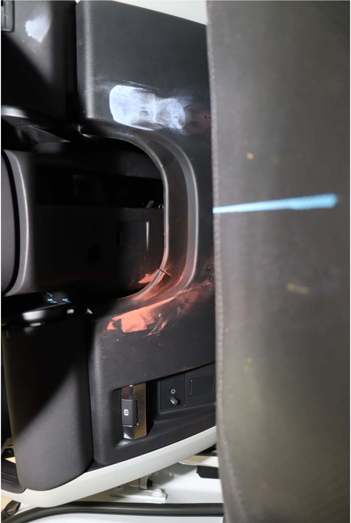
Photo No. 46. Post-Test Driver Dummy Knee Contact
