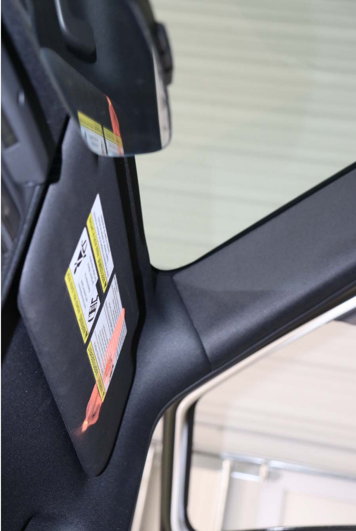
Photo No. 14 - Post-Test 5th Fem. P2 Driver Dummy Head Contact (visor)
