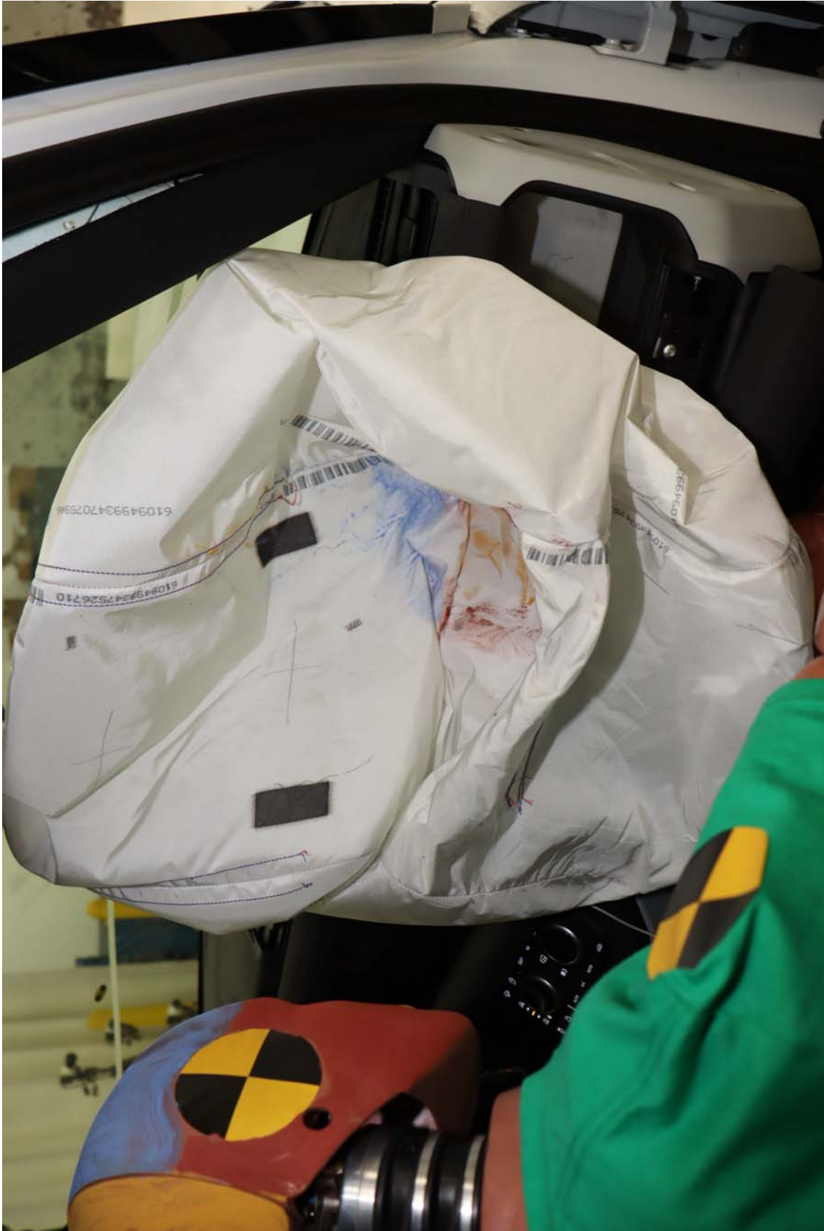
Photo No. 61. Post-Test Passenger Dummy Airbag Contact
