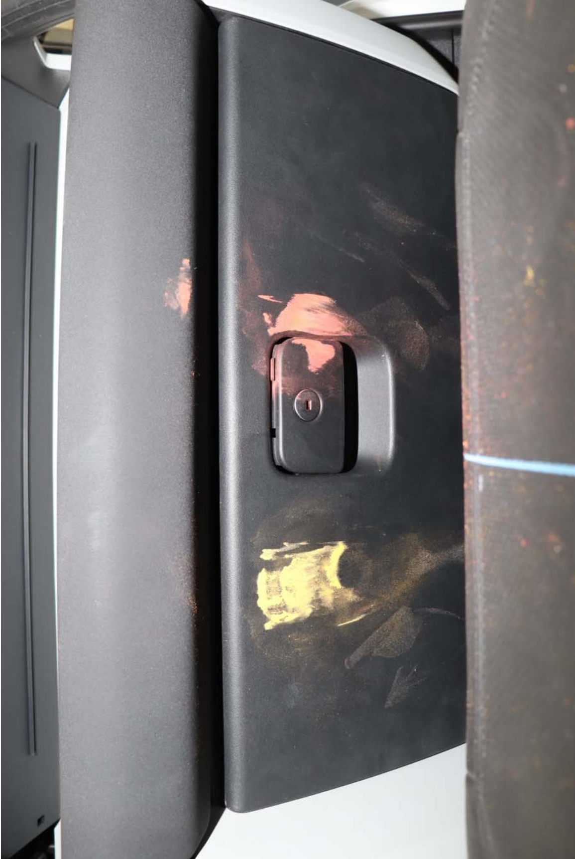
Photo No. 62. Post-Test Passenger Dummy Knee Contact
