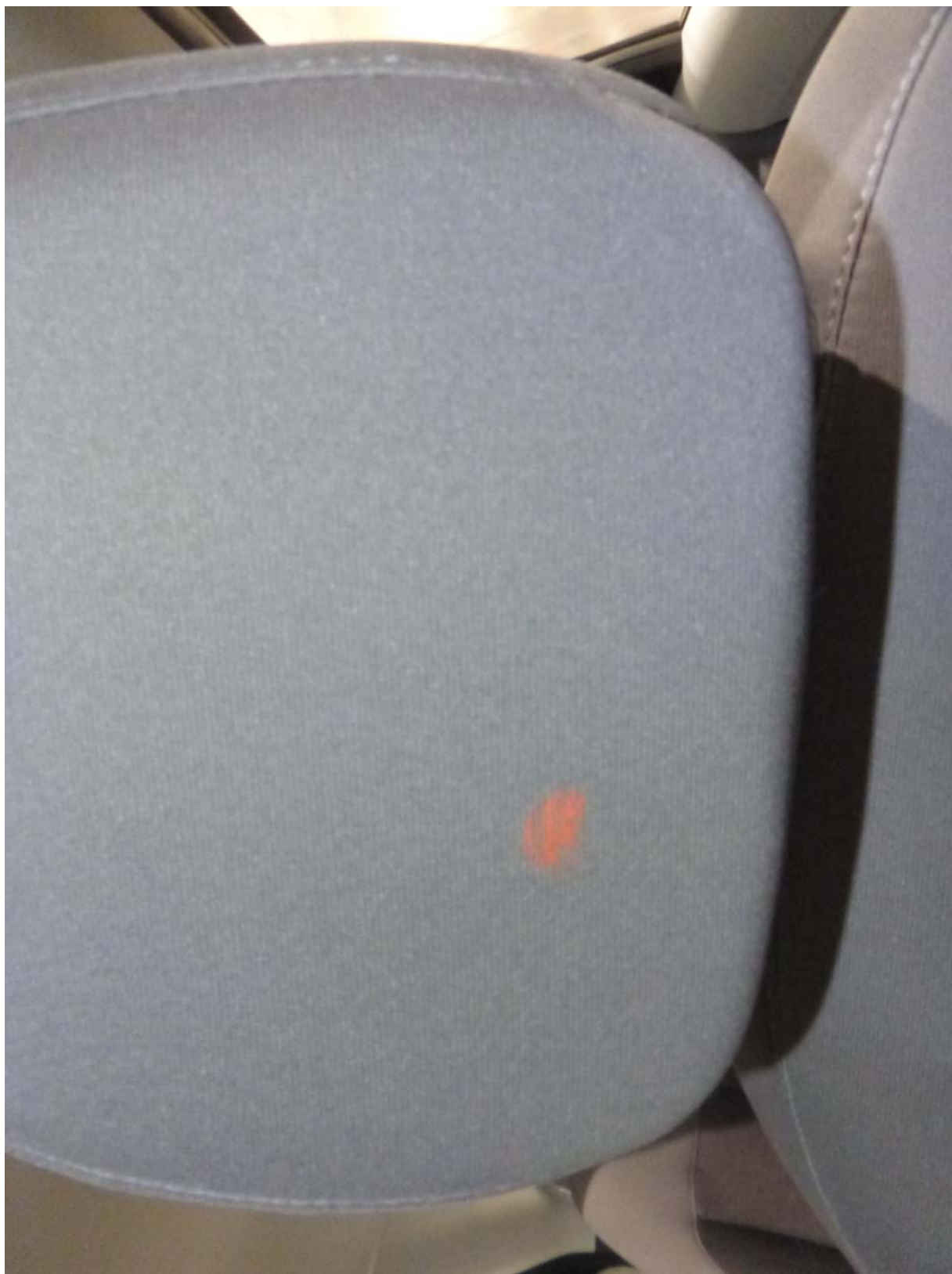
Photo No. 47. Post-Test Driver Dummy Head Contact (headrest)
