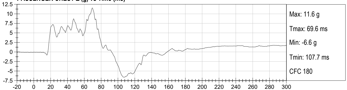
PASSENGER CHEST Resultant (g) vs Time (ms)
