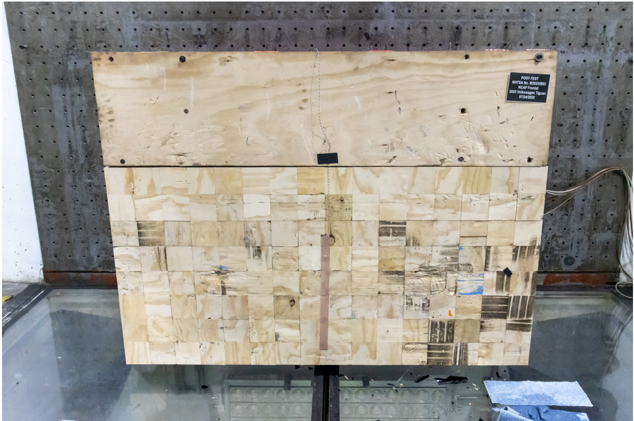
Figure A-3: Post-Test Load Cell Wall
