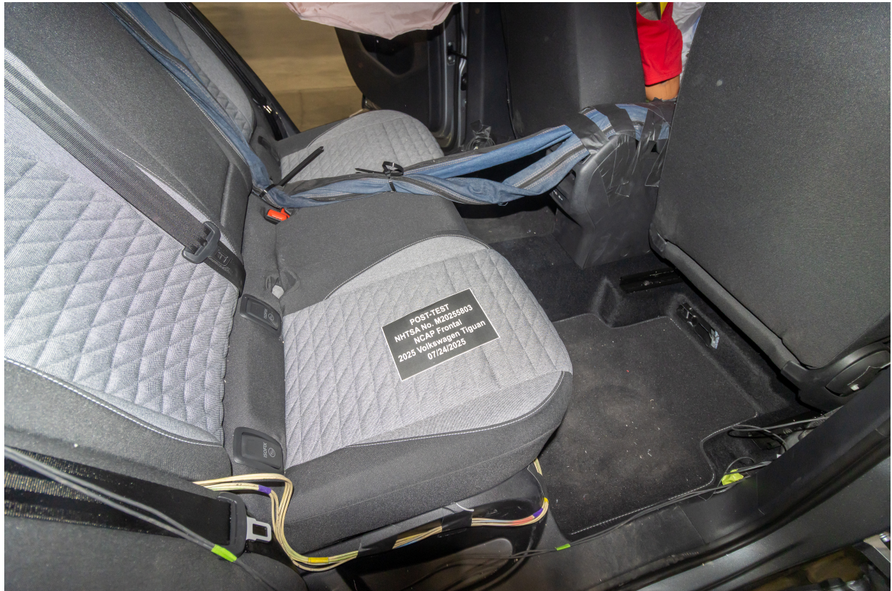
Figure A-29: Post-Test Dummy Cable Routing
