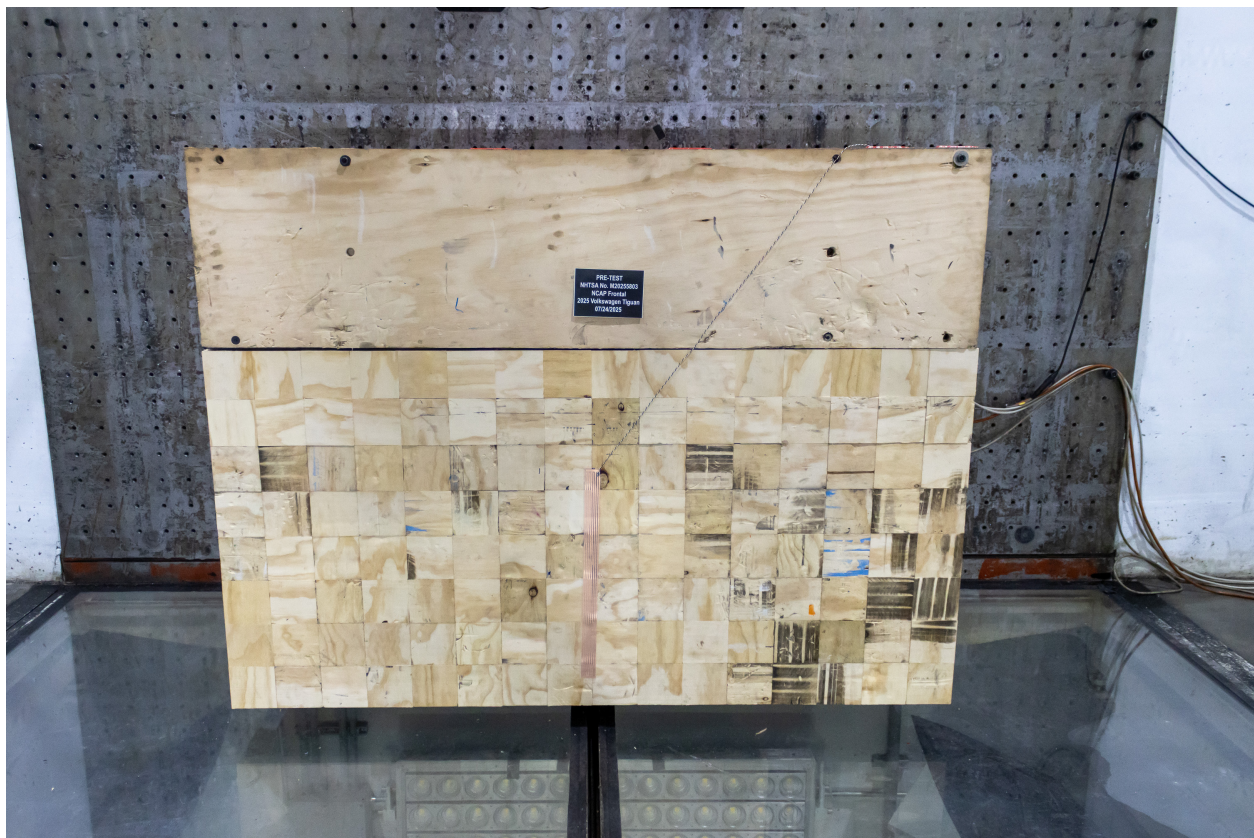
Figure A-2: Pre-Test Load Cell Wall
