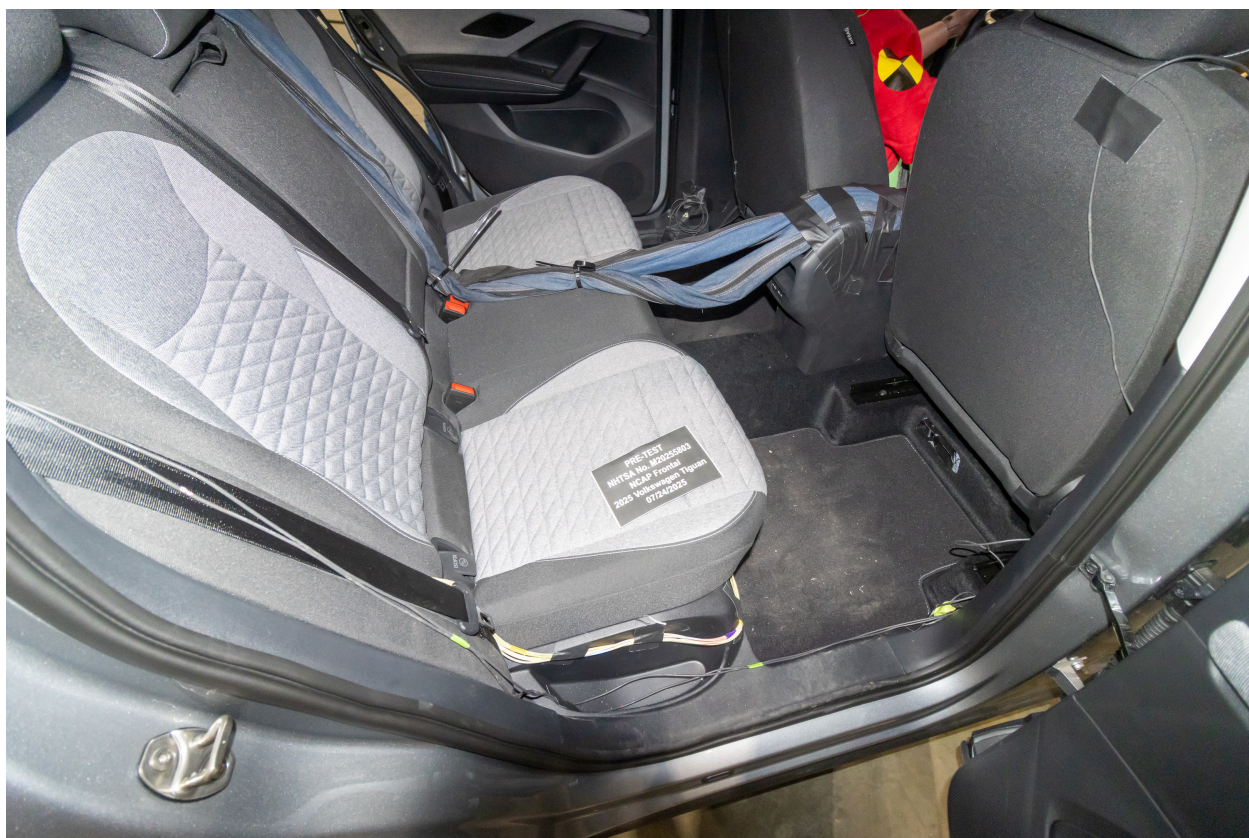
Figure A-28: Pre-Test Dummy Cable Routing
