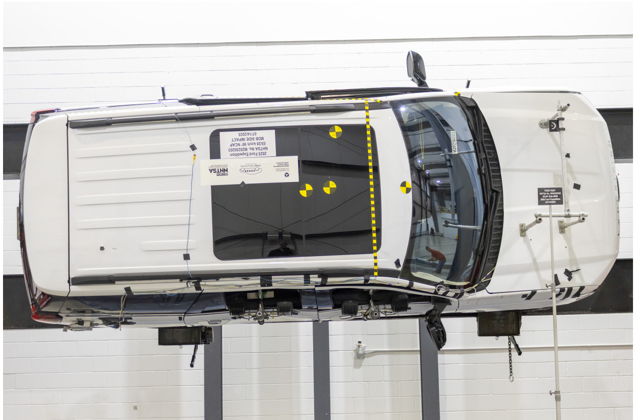
Figure A-99: FMVSS No. 301 Static Rollover 270 Degrees
