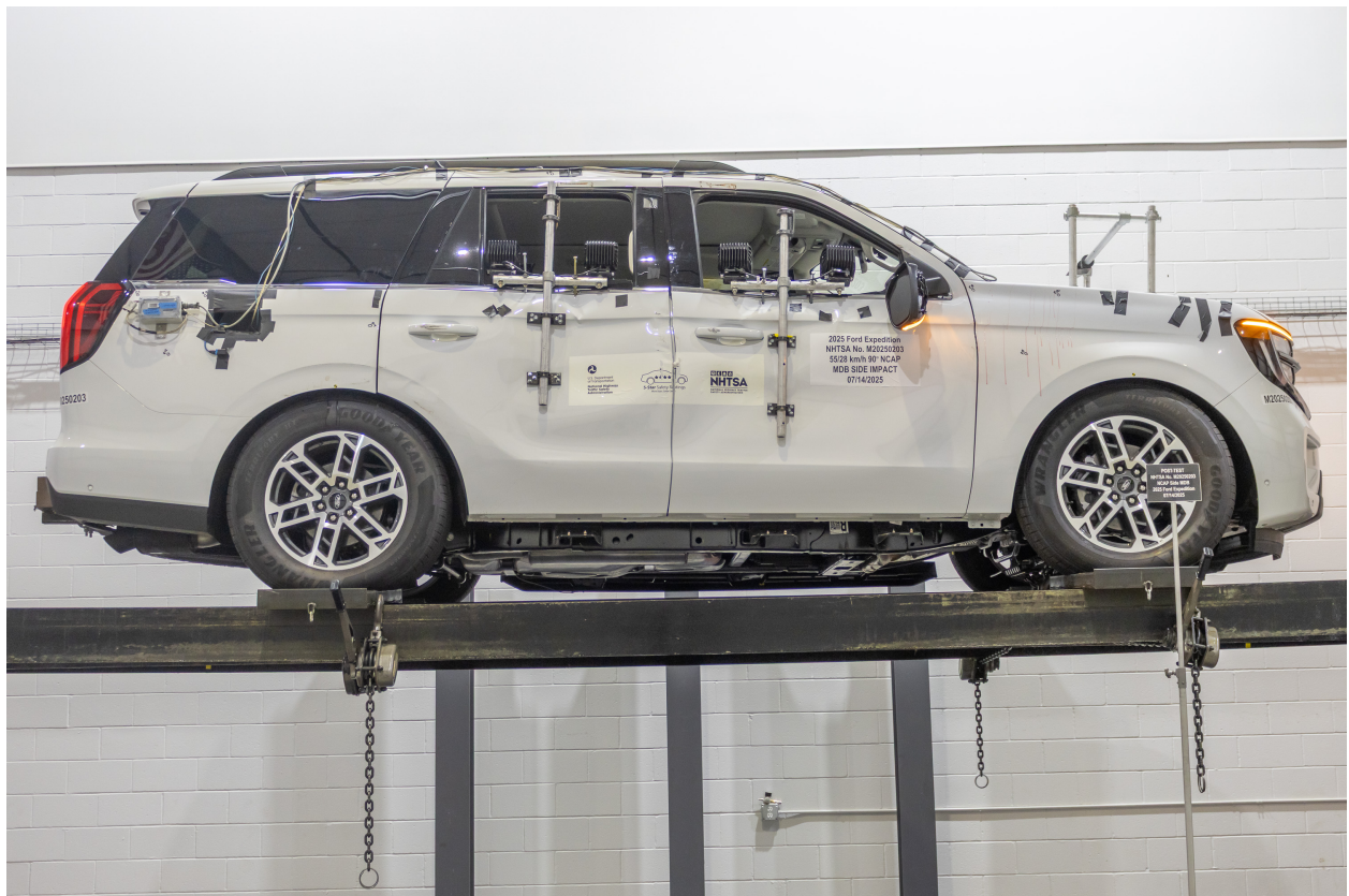
Figure A-100: FMVSS No. 301 Static Rollover 360 Degrees
