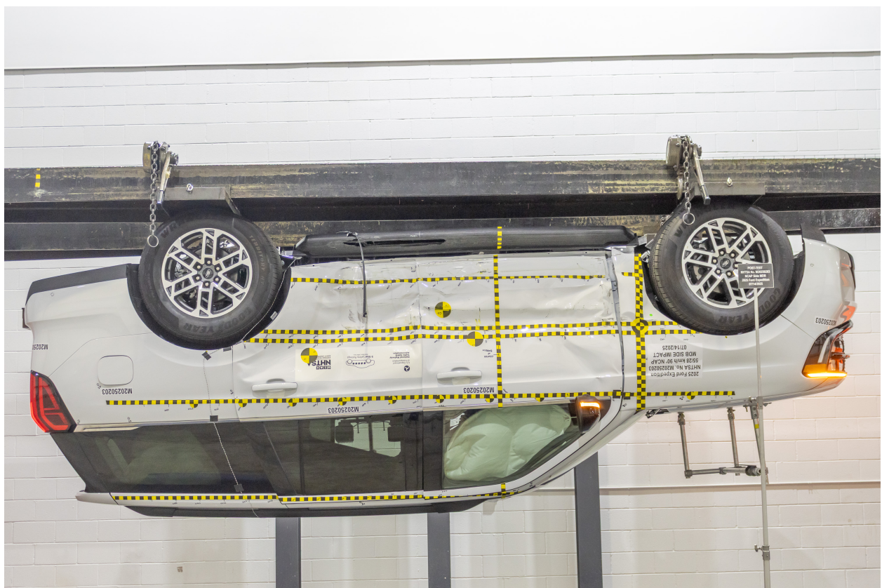
Figure A-98: FMVSS No. 301 Static Rollover 180 Degrees
