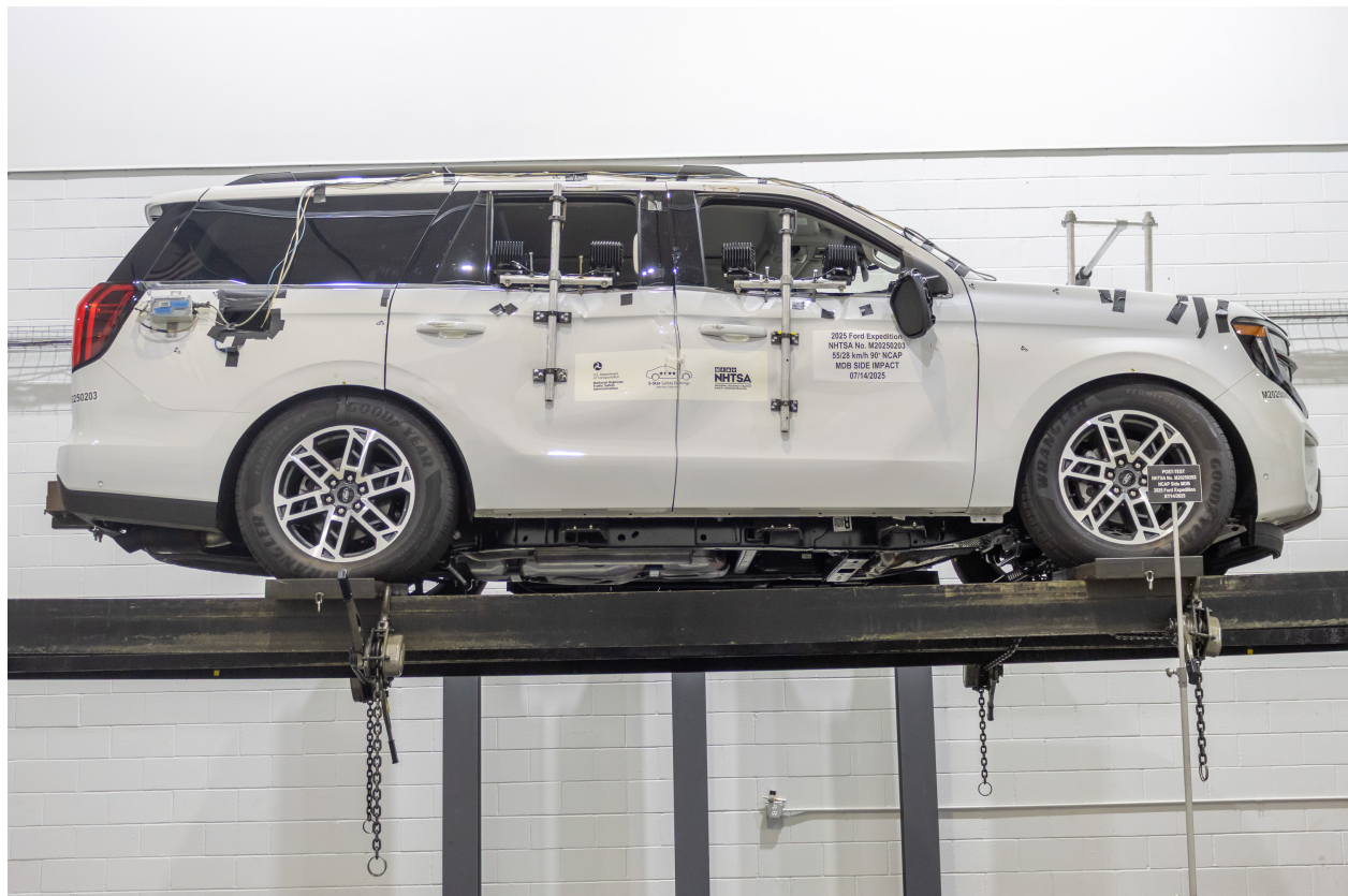
Figure A-96: FMVSS No. 301 Static Rollover 0 Degrees
