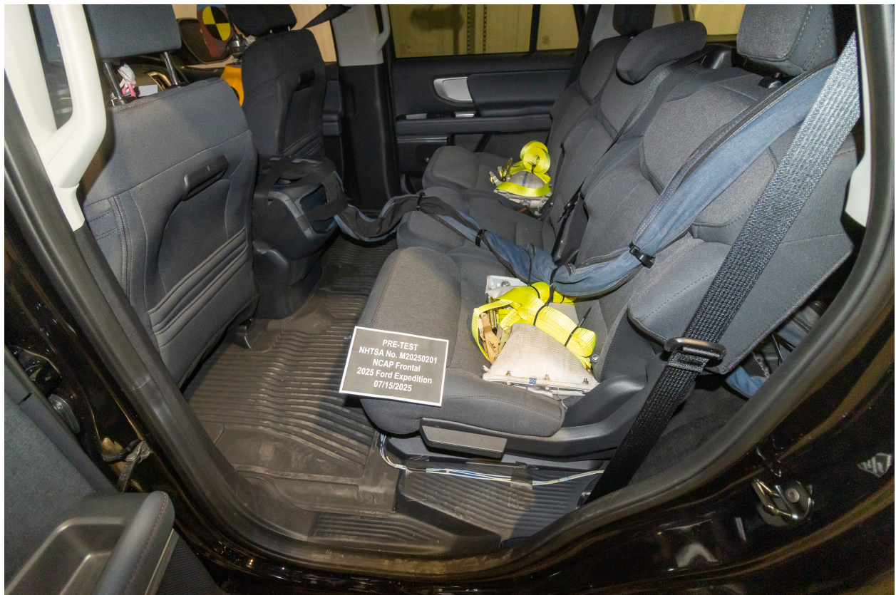
Figure A-28: Pre-Test Dummy Cable Routing
