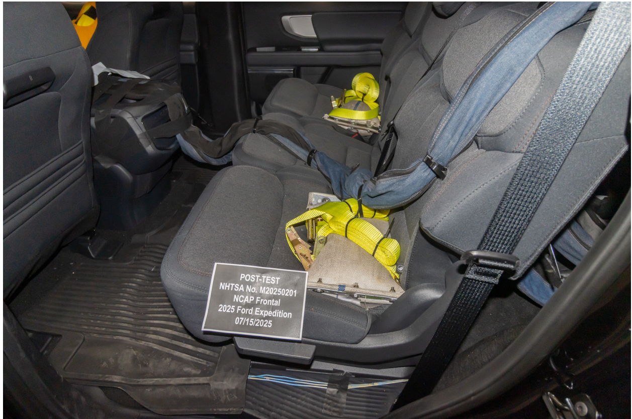
Figure A-29: Post-Test Dummy Cable Routing
