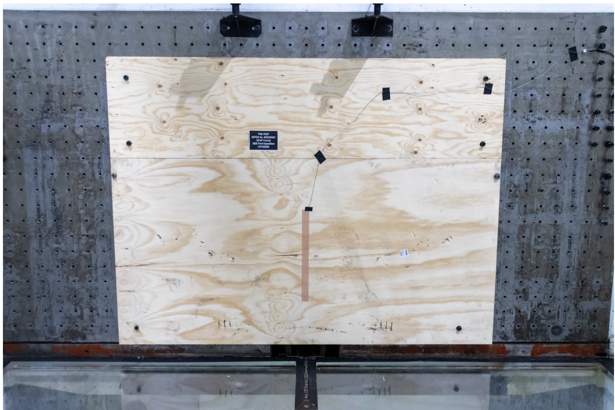
Figure A-2: Pre-Test Load Cell Wall
