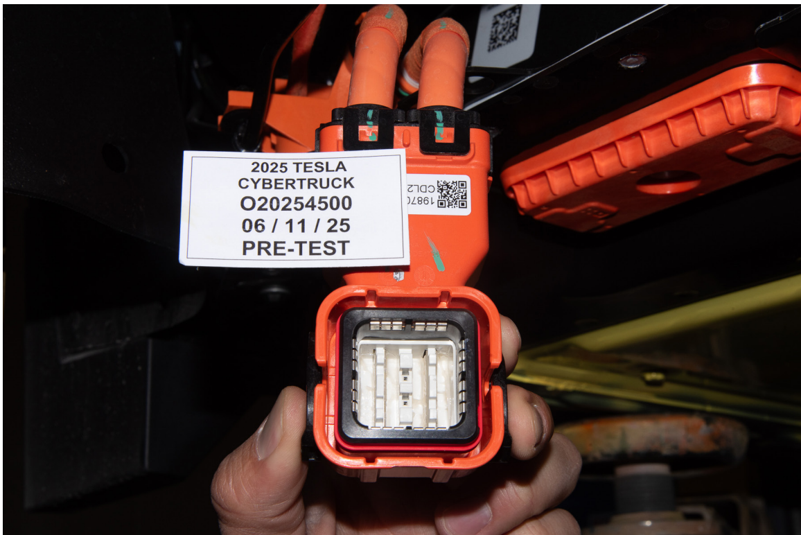
FIGURE 305-07a Manual High Voltage Service Disconnect Removed
