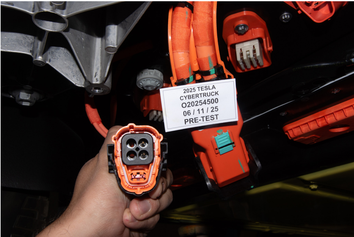
FIGURE 305-07c Manual High Voltage Service Disconnect Removed
