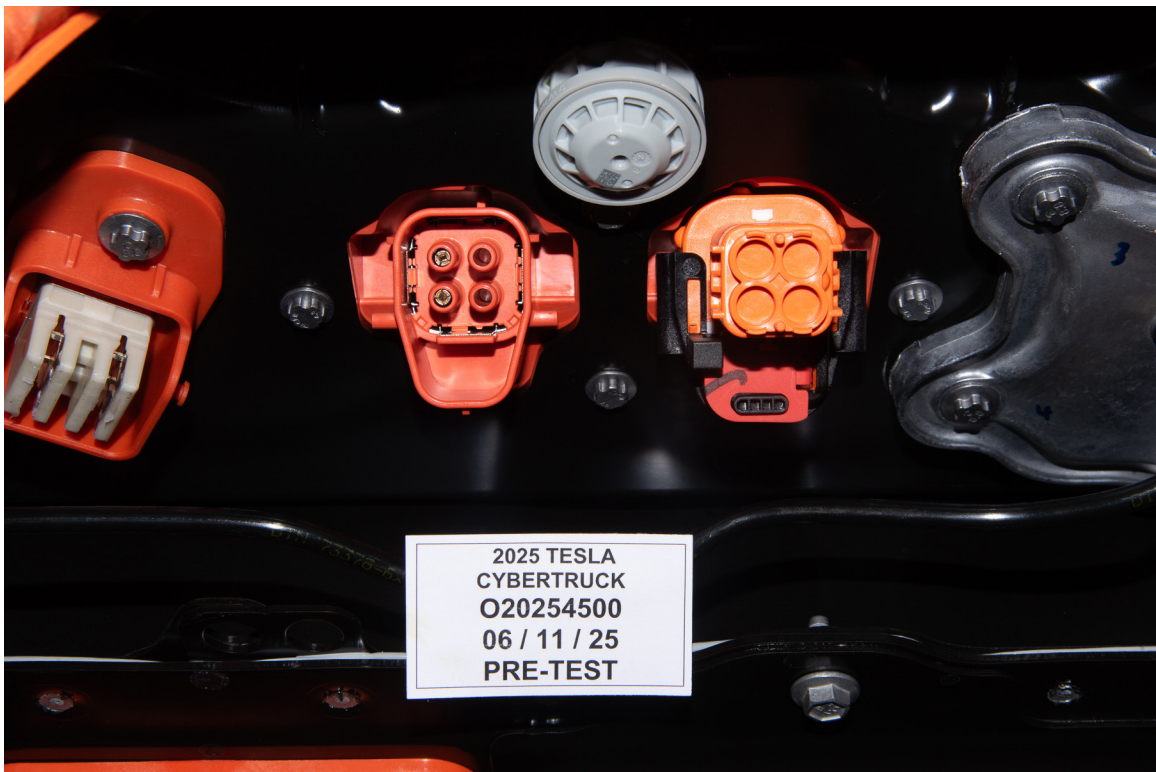
FIGURE 305-08a Manual High Voltage Service Disconnect Removed
