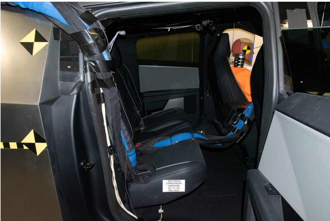
FIGURE 28. Pre-Test Dummy Cable Routing
