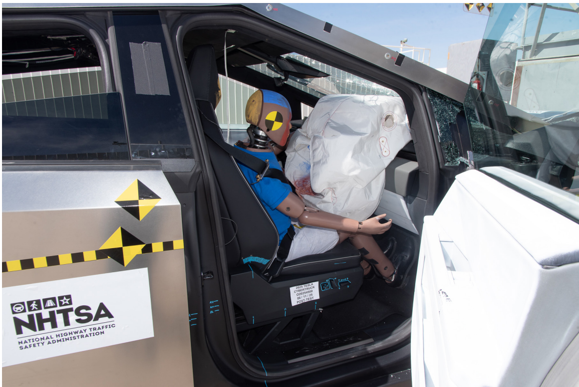
FIGURE 58. Post-Test Passenger Dummy and Vehicle Interior View
