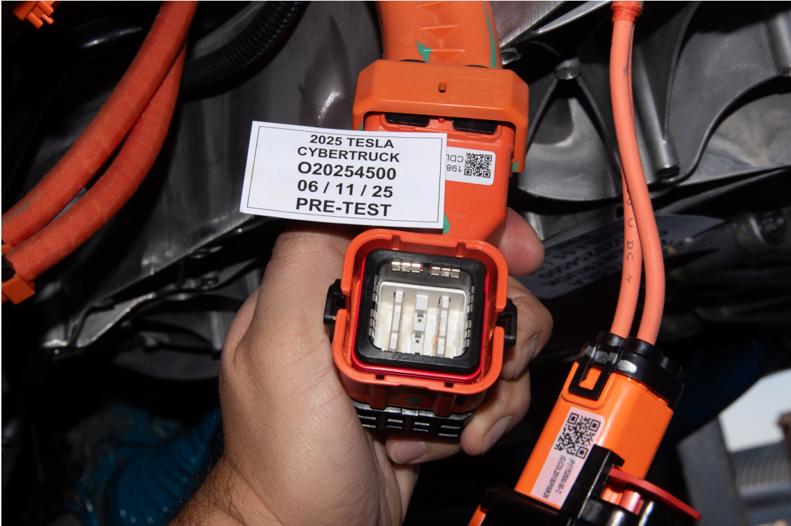
FIGURE 305-07b Manual High Voltage Service Disconnect Removed
