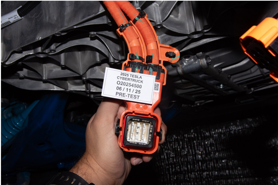
FIGURE 305-07d Manual High Voltage Service Disconnect Removed
