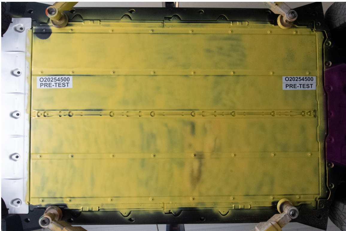
FIGURE 305-09. Pre-Impact View of Propulsion Battery
