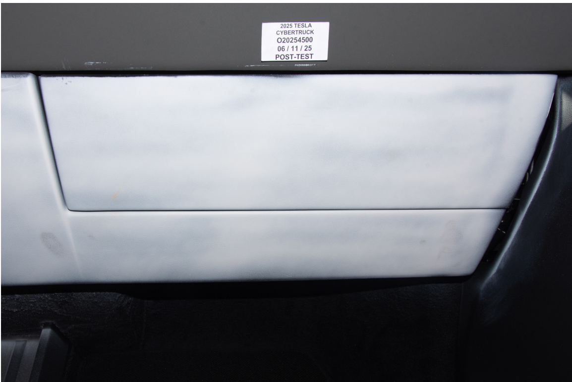
FIGURE 68. Post-Test Passenger's Side Knee Bolster
