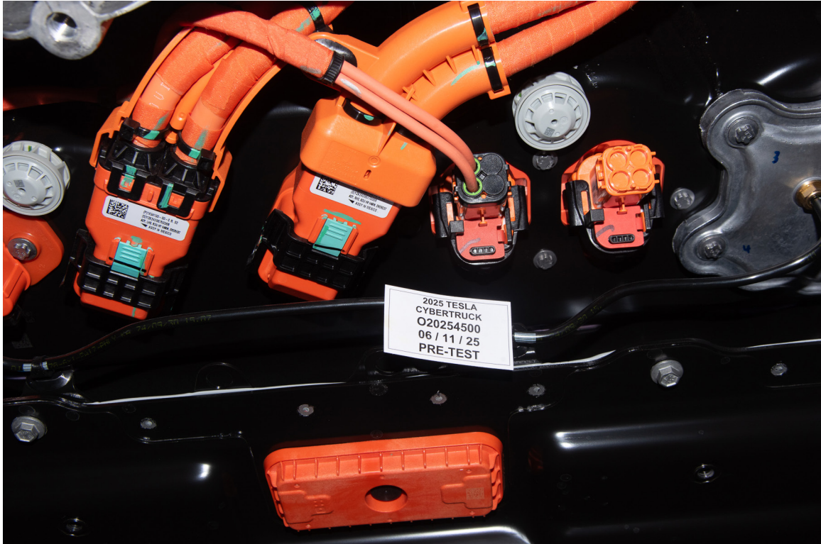
FIGURE 305-06e Manual High Voltage Service Disconnect in Place
