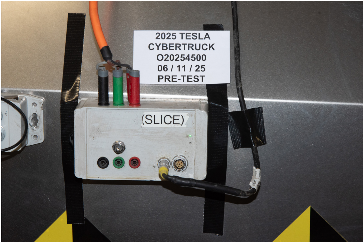
FIGURE 305-024. Pre-Impact View of Installed Test Interface Port
