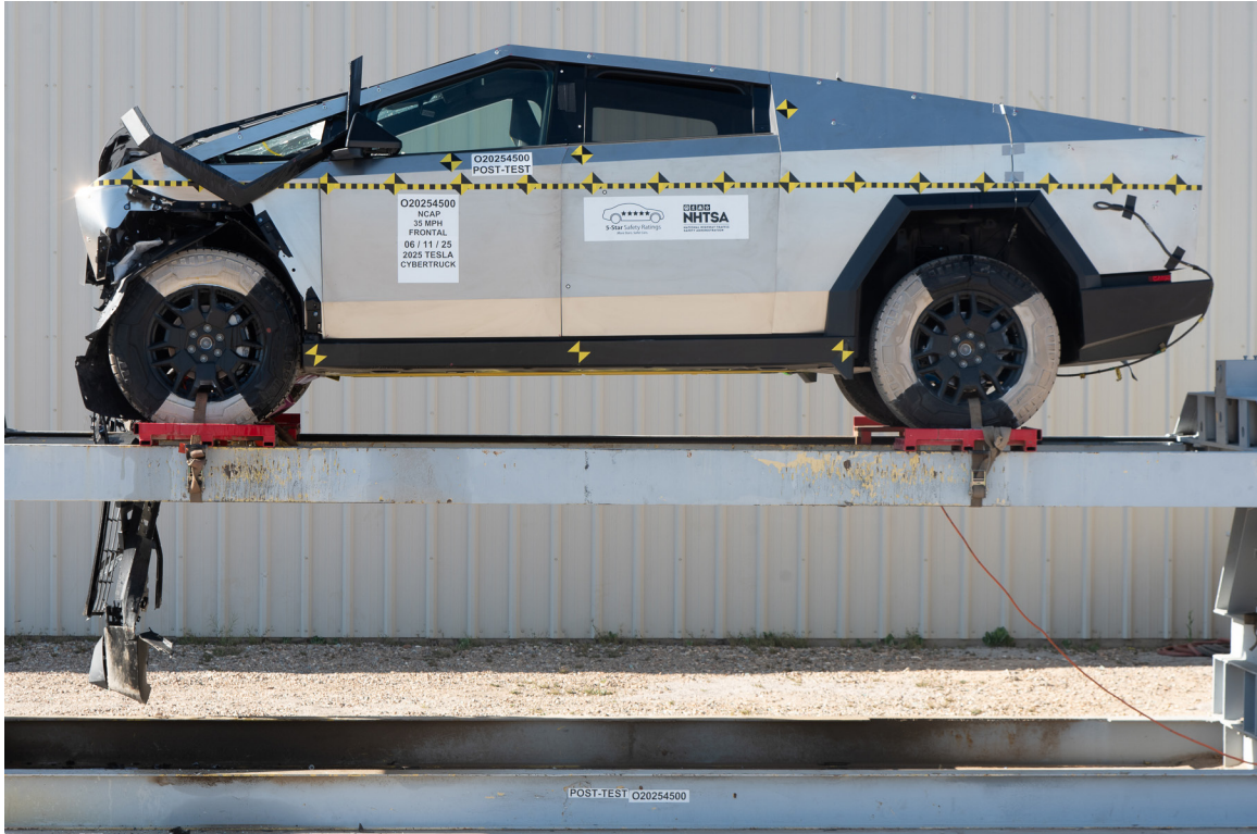
FIGURE 81. Vehicle at 360° on Static Rollover Device
