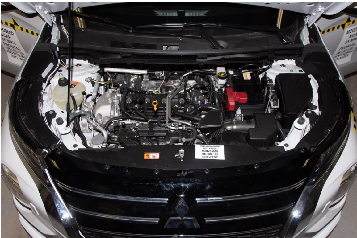
FIGURE 20. Pre-Test Engine Compartment View
