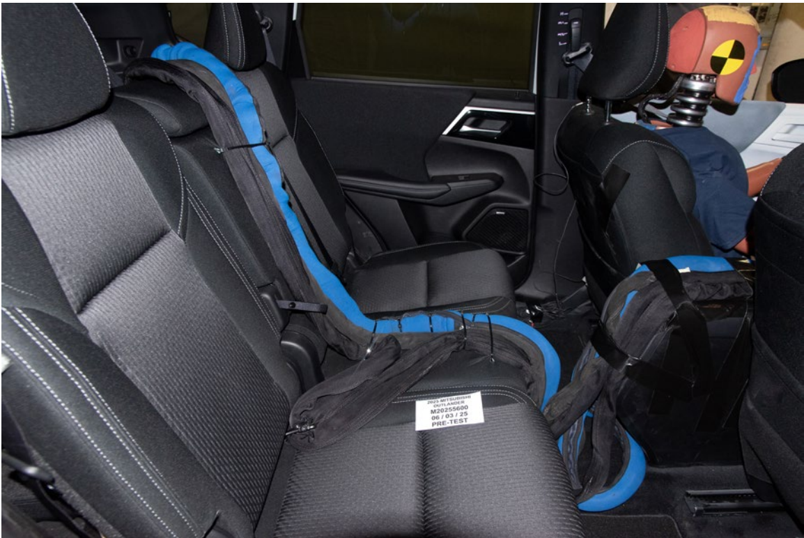
FIGURE 28. Pre-Test Dummy Cable Routing
