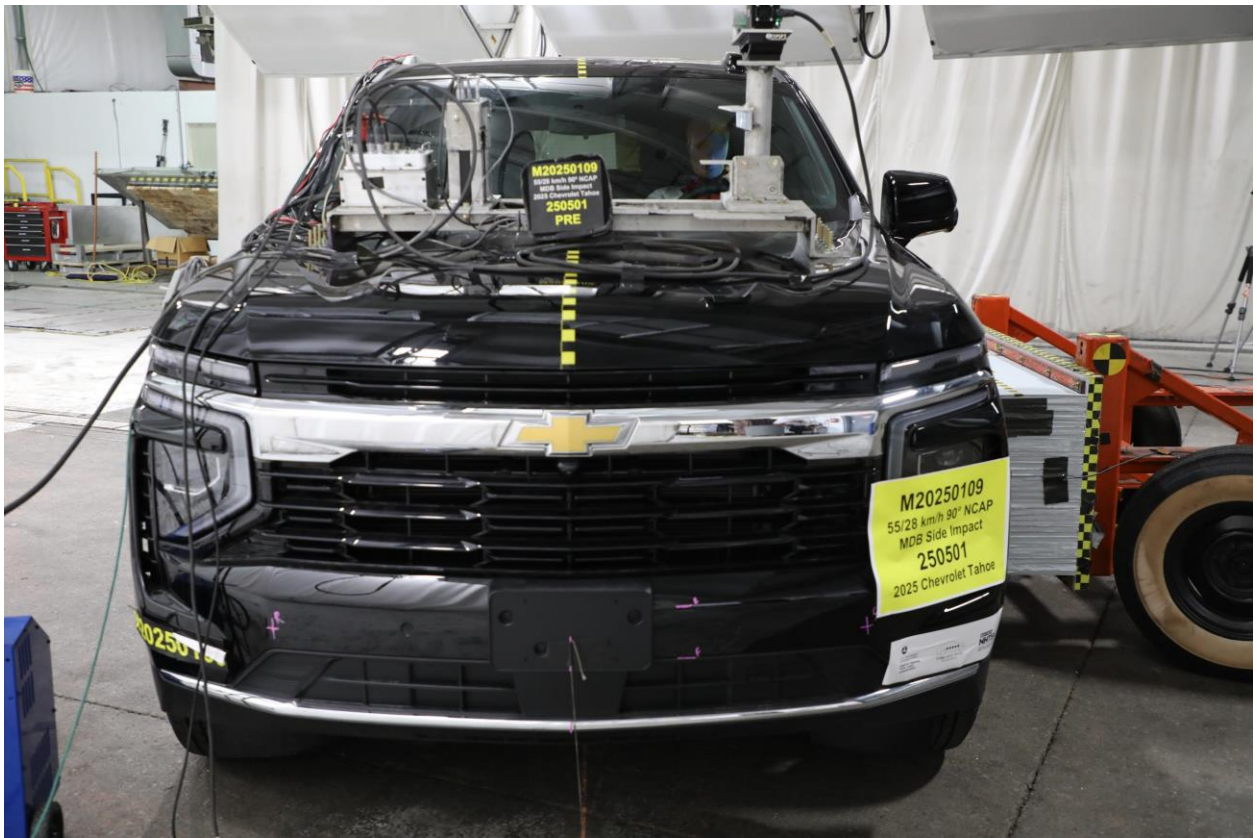
003 Pre-Test Frontal View of Test Vehicle
