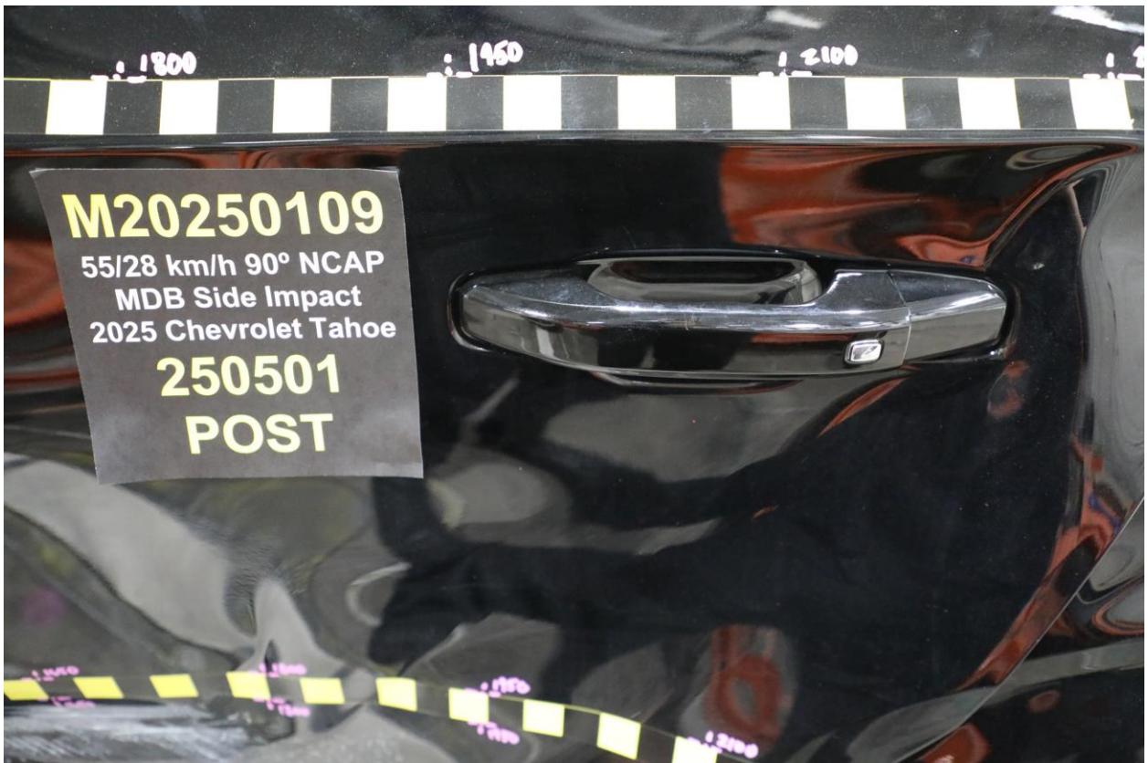
024 Post-Test Left Rear Door Latch Close-Up
