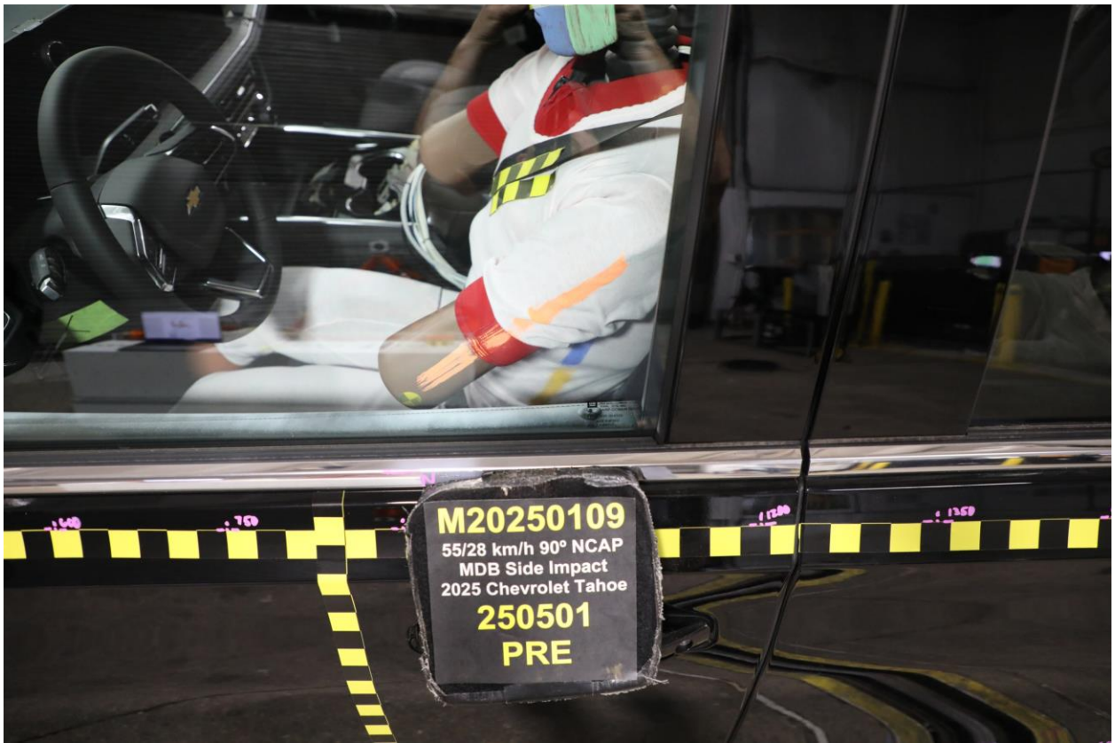
042 Pre-Test Driver Dummy and Door Clearance View
