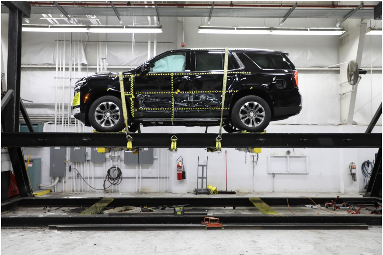
100 FMVSS No. 301 Static Rollover 360 Degrees
