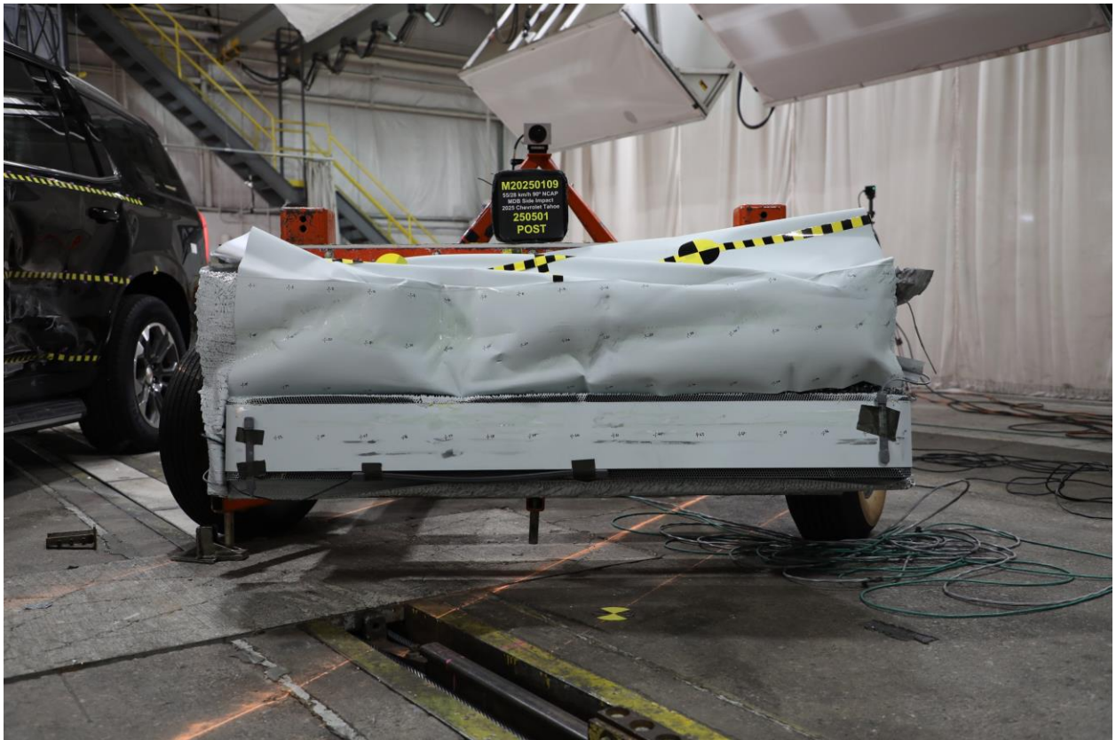
085 Post-Test Front View of MDB Impactor Face
