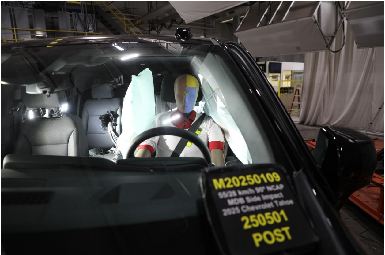
026 Post-Test Front Close-Up View of Driver Dummy
