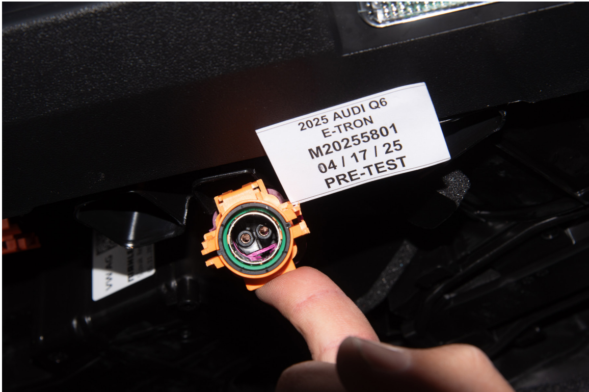
FIGURE 305-07. Manual High Voltage Service Disconnect Removed
