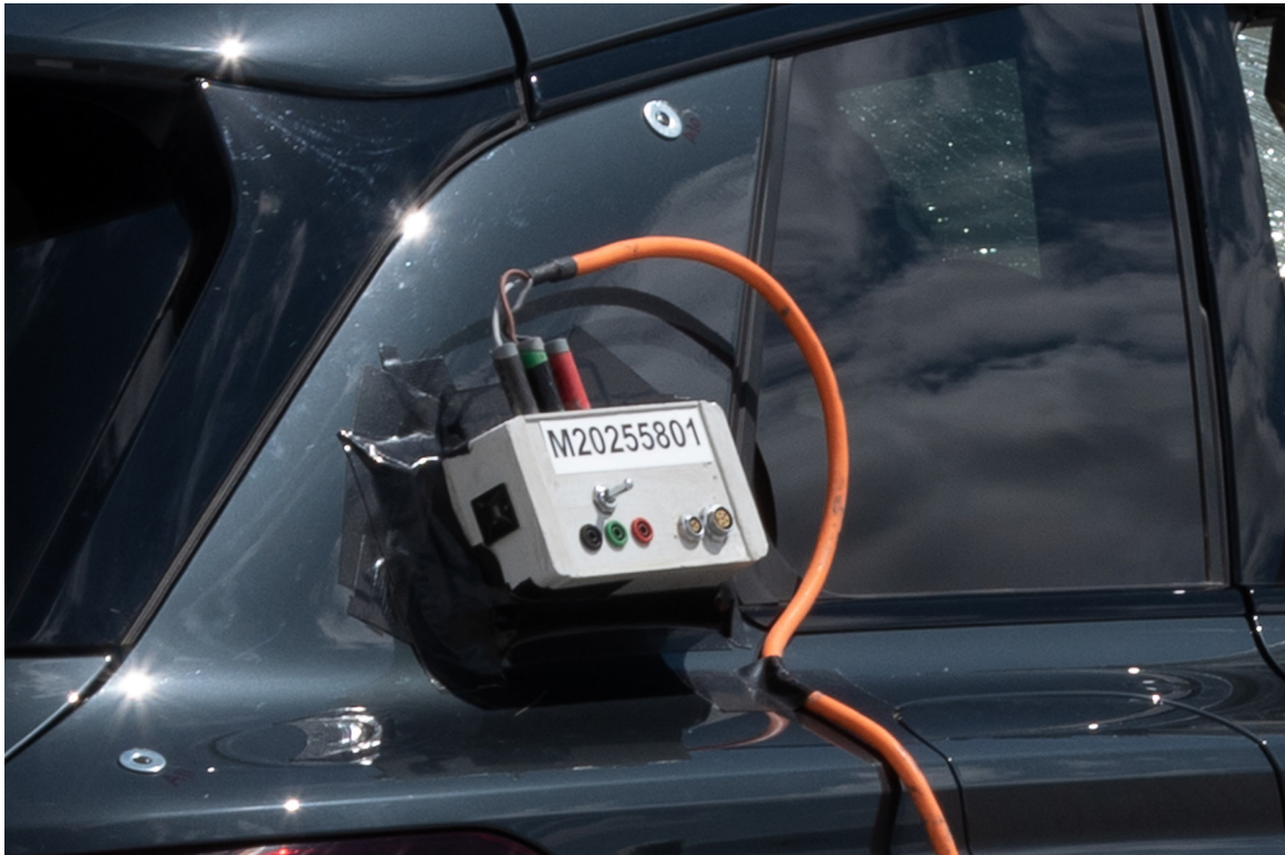
FIGURE 305-025. Post-Impact View of Installed Test Interface Port
