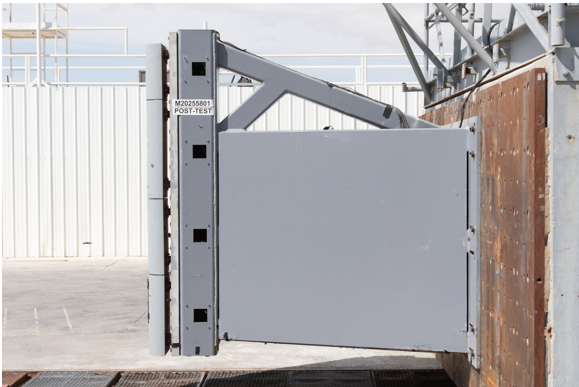
FIGURE 62. Post-Test Pole Barrier Side View
