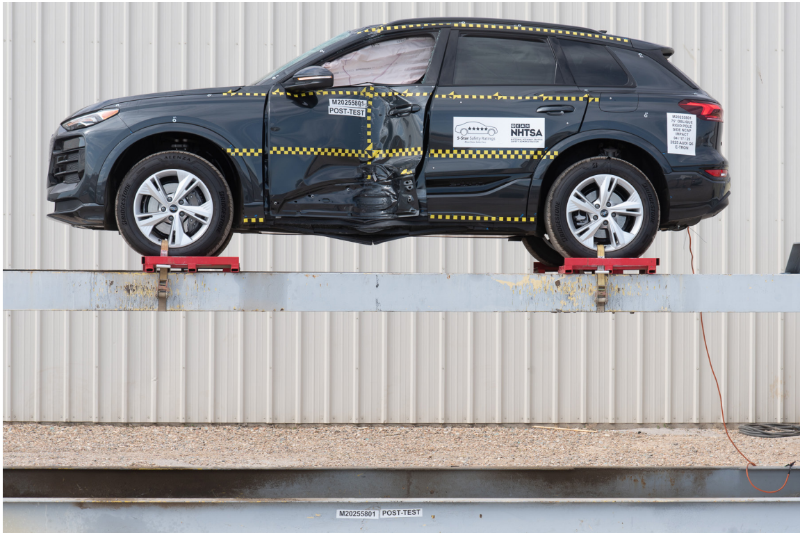
FIGURE 69. FMVSS No. 301 Static Rollover 360 Degrees
