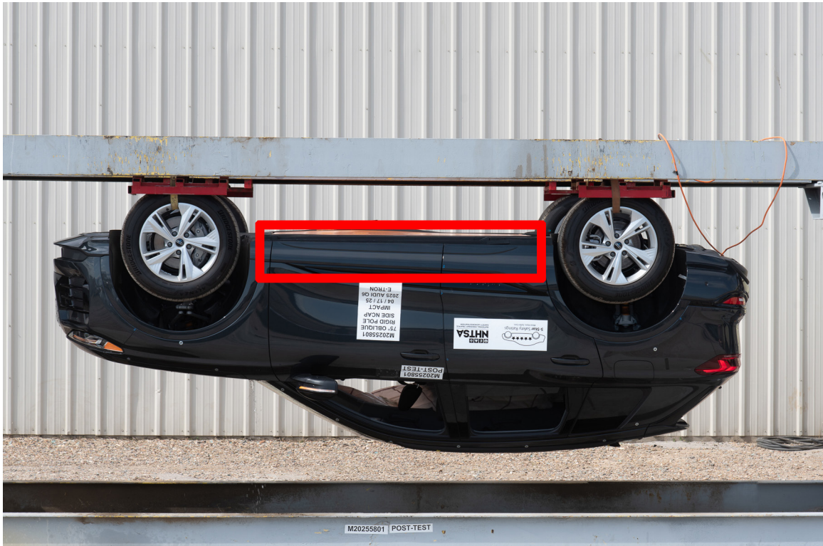
FIGURE 305-029. FMVSS No. 305 Static Rollover at 180°
