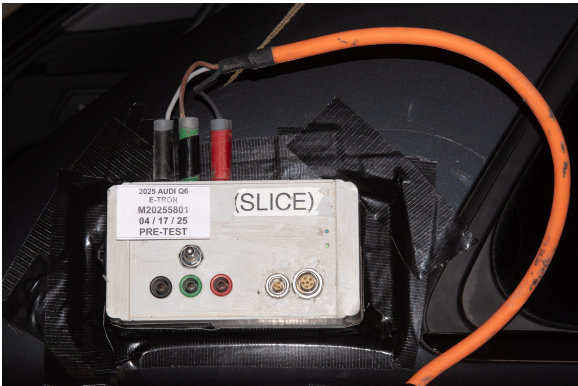
FIGURE 305-024. Pre-Impact View of Installed Test Interface Port
