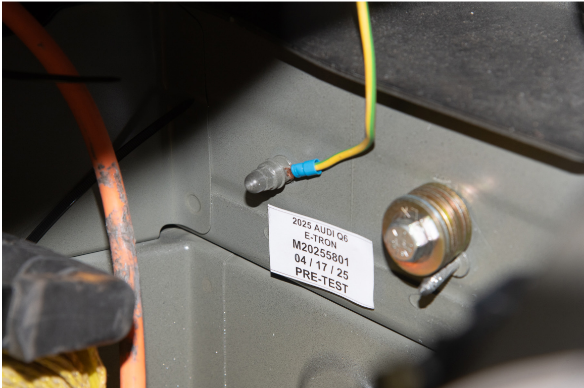
FIGURE 305-021. Pre-Impact View of Ground Lead Attached
