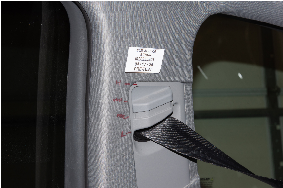
FIGURE 33. Pre-Test View of Belt Anchorage for Dummy
