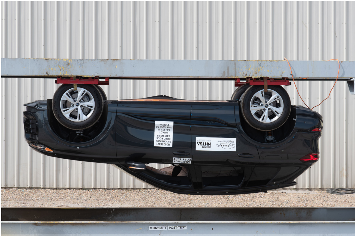
FIGURE 67. FMVSS No. 301 Static Rollover 180 Degrees
