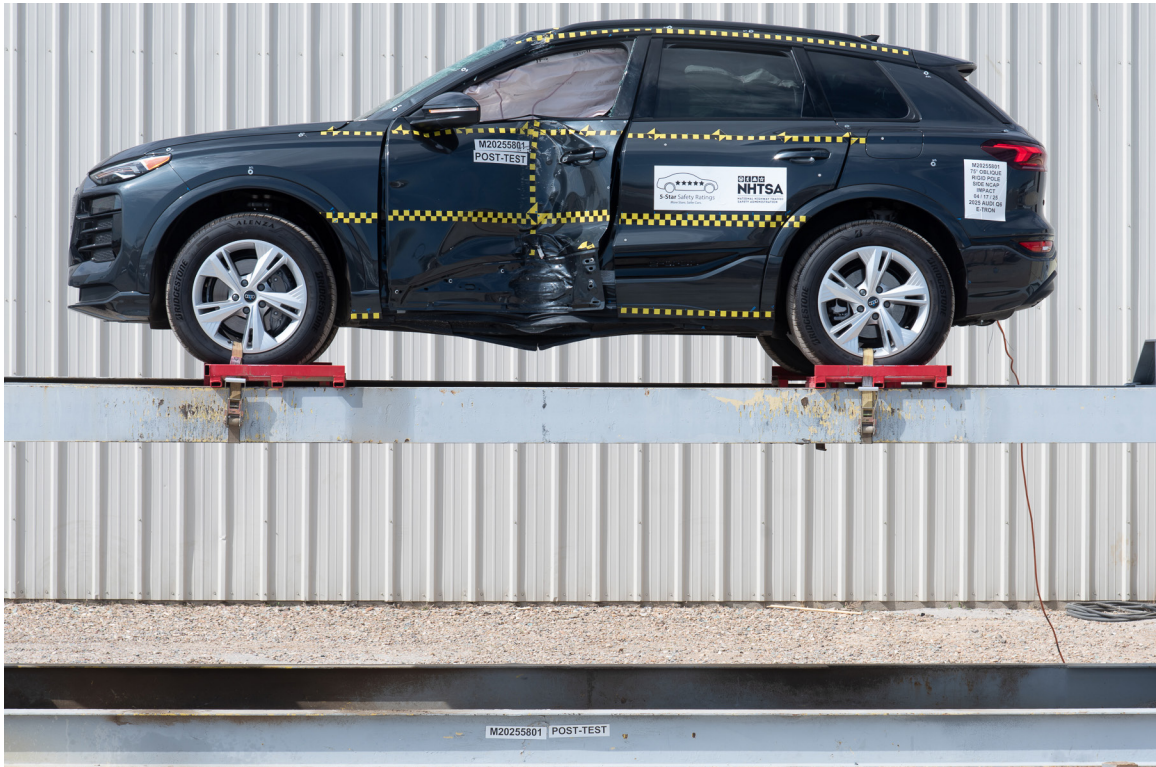
FIGURE 65. FMVSS No. 301 Static Rollover 0 Degrees
