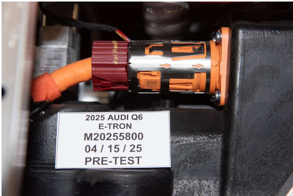
FIGURE 305-018. Pre-Impact View of High Voltage Interconnect(s)
