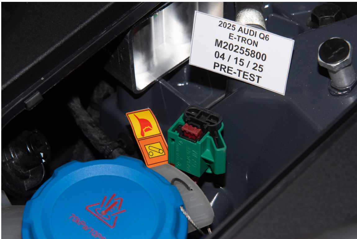
FIGURE 305-03. First Responder Warning Label
