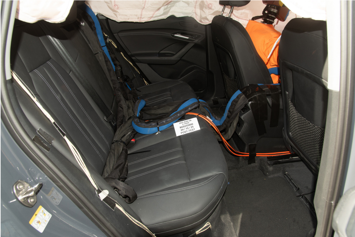
FIGURE 29. Post-Test Dummy Cable Routing
