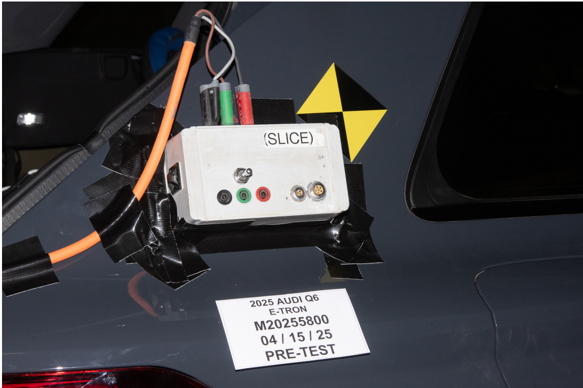
FIGURE 305-024. Pre-Impact View of Installed Test Interface Port
