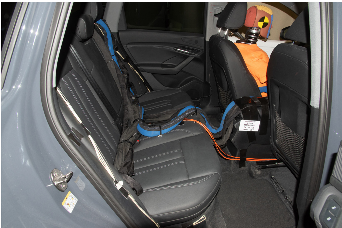
FIGURE 28. Pre-Test Dummy Cable Routing
