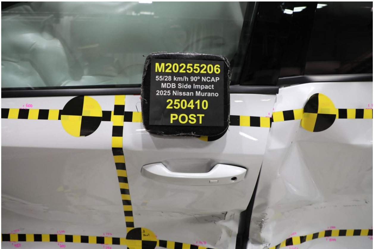
022 Post-Test Left Front Door Latch Close-Up
