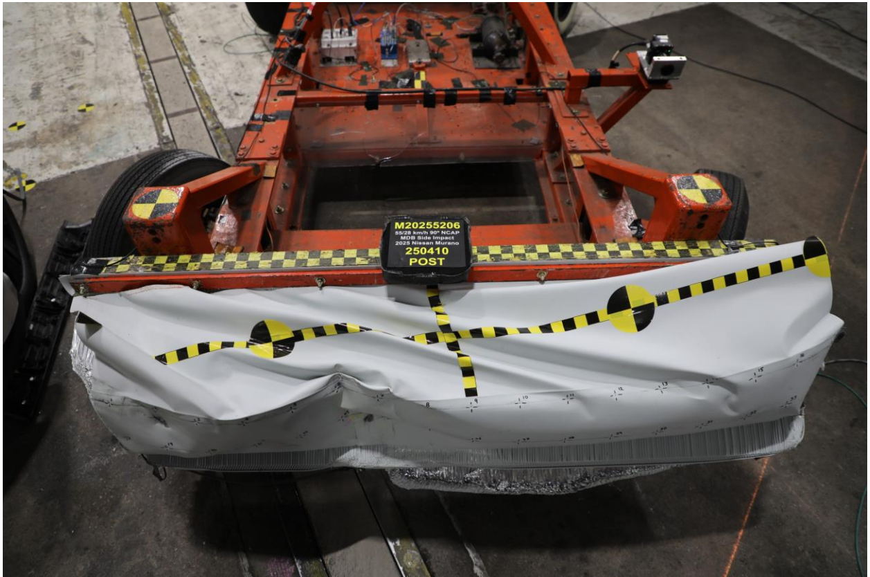
087 Post-Test Top View of MDB Impactor Face
