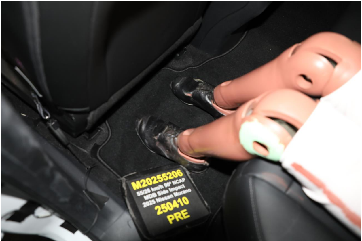
064 Pre-Test Placement of Rear Passenger Dummy's Feet
