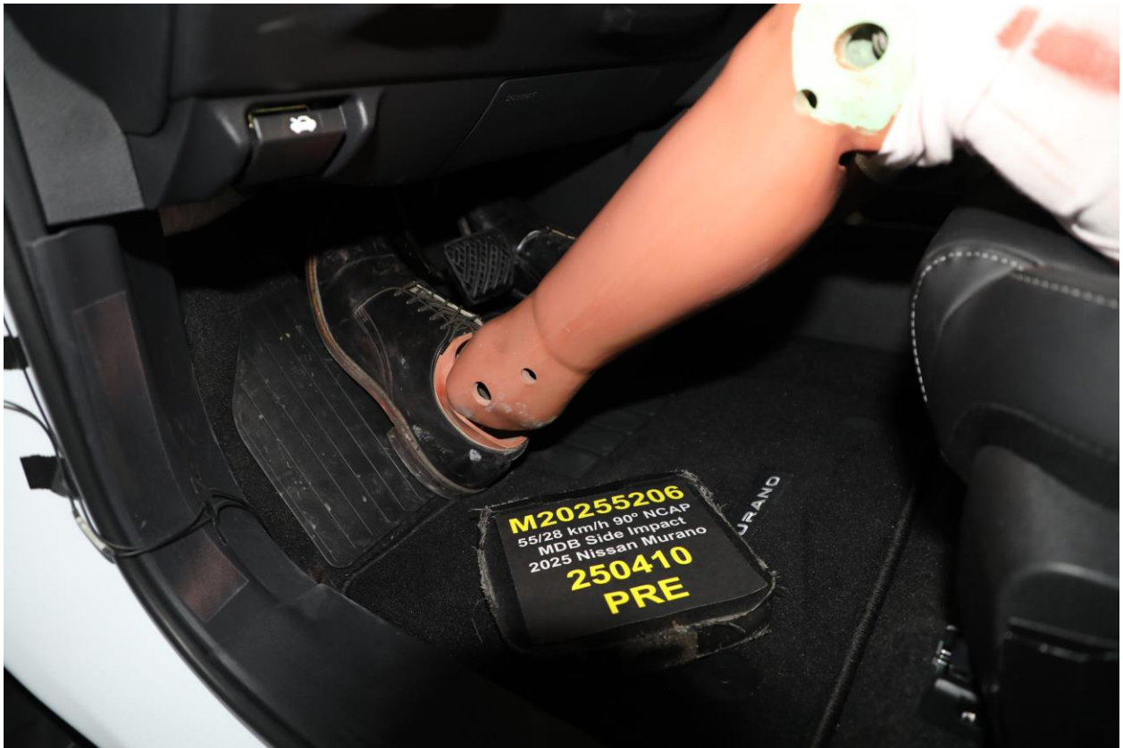
034 Pre-Test Placement of Driver's Dummy Feet
