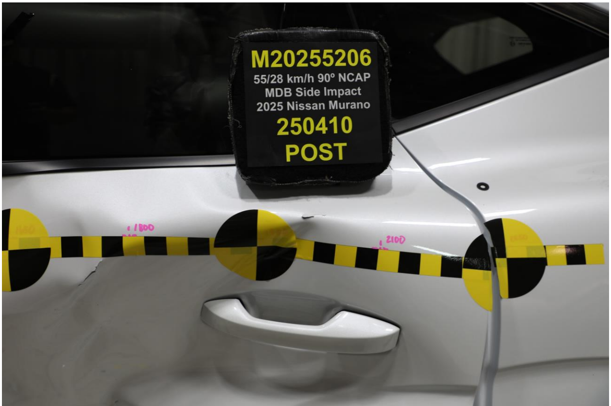
024 Post-Test Left Rear Door Latch Close-Up
