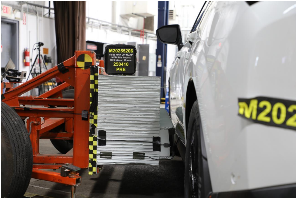
018 Pre-Test Right Side View of MDB Positioned Against Side of Test Vehicle
