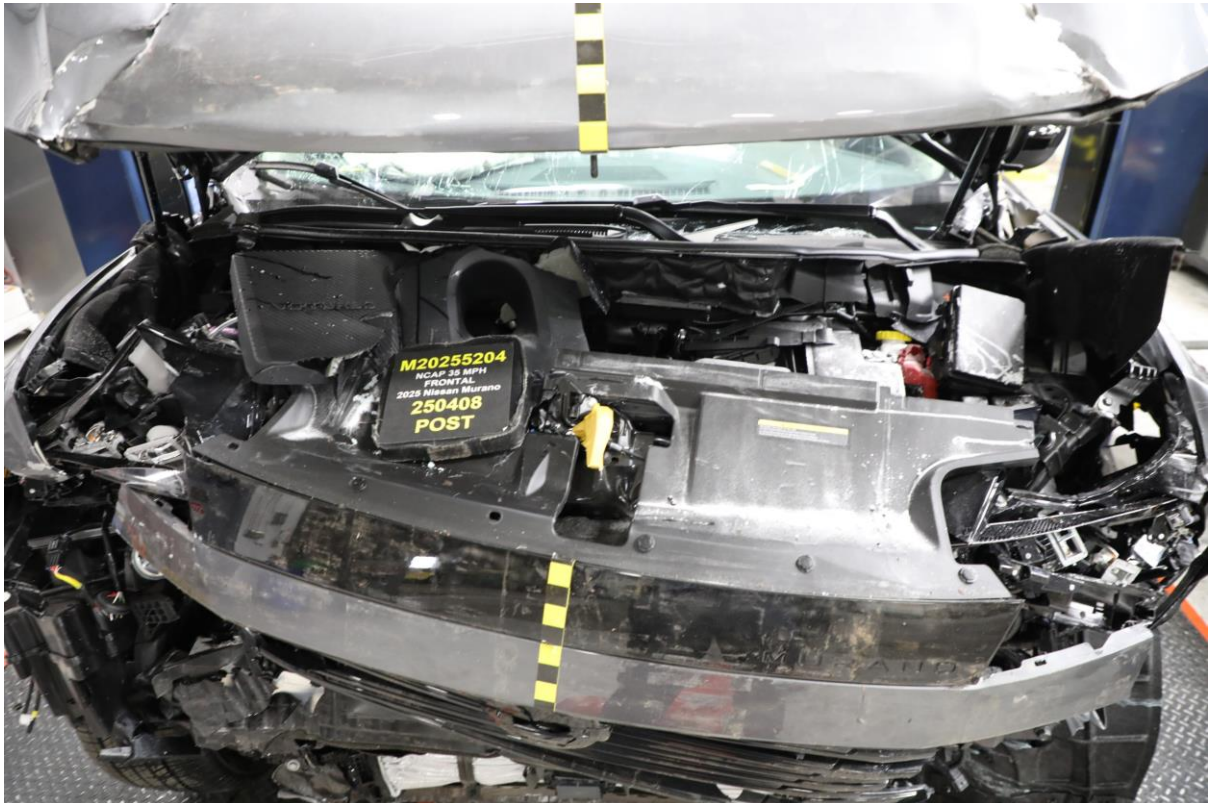
021 Post-Test Engine Compartment View
