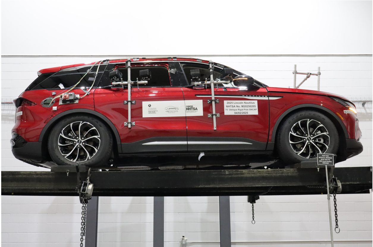
Figure A-65: FMVSS No. 301 Static Rollover 0 Degrees
