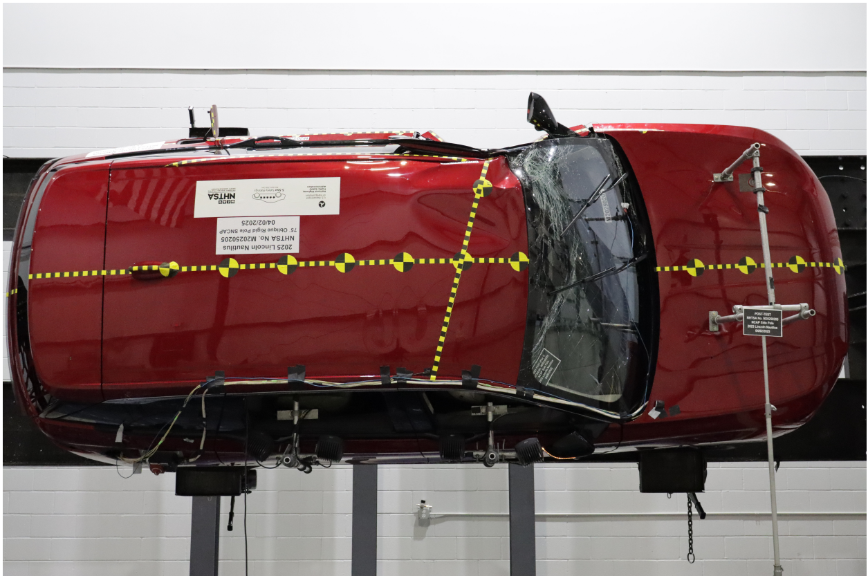
Figure A-68: FMVSS No. 301 Static Rollover 270 Degrees
