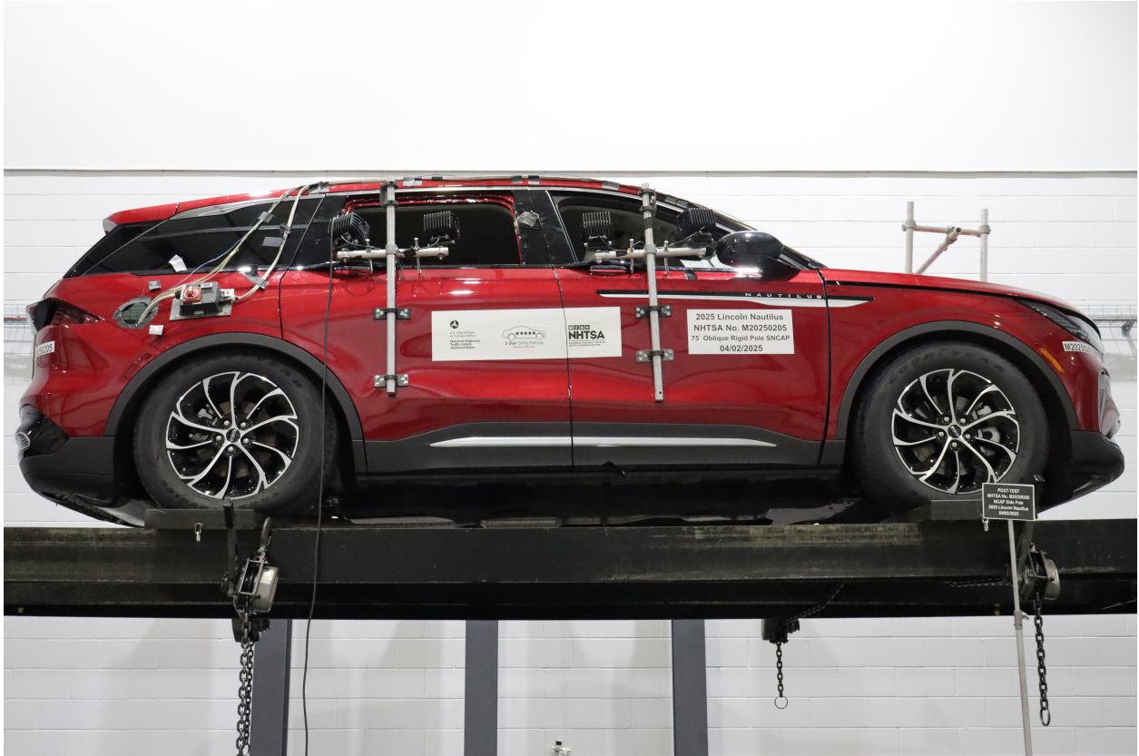
Figure A-69: FMVSS No. 301 Static Rollover 360 Degrees
