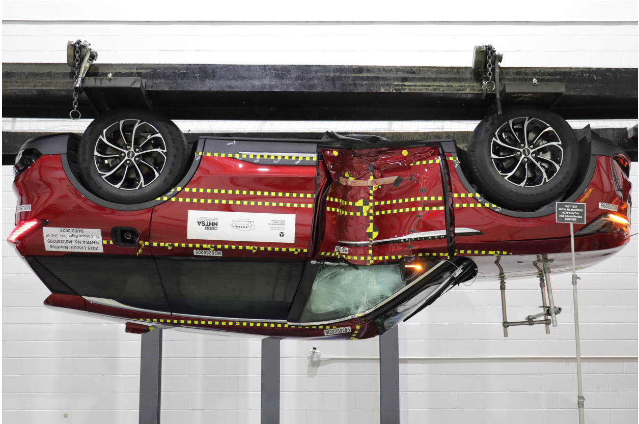
Figure A-67: FMVSS No. 301 Static Rollover 180 Degrees
