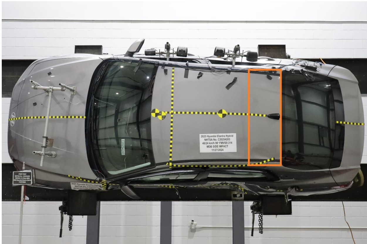
Figure 305-28: FMVSS No. 305 Static Rollover 90 Degrees
