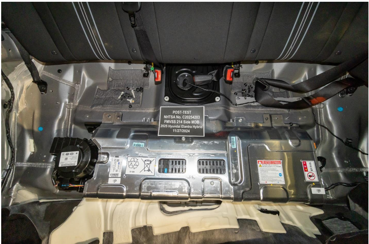
Figure 305-10: Post-Impact Front View of Propulsion Battery
