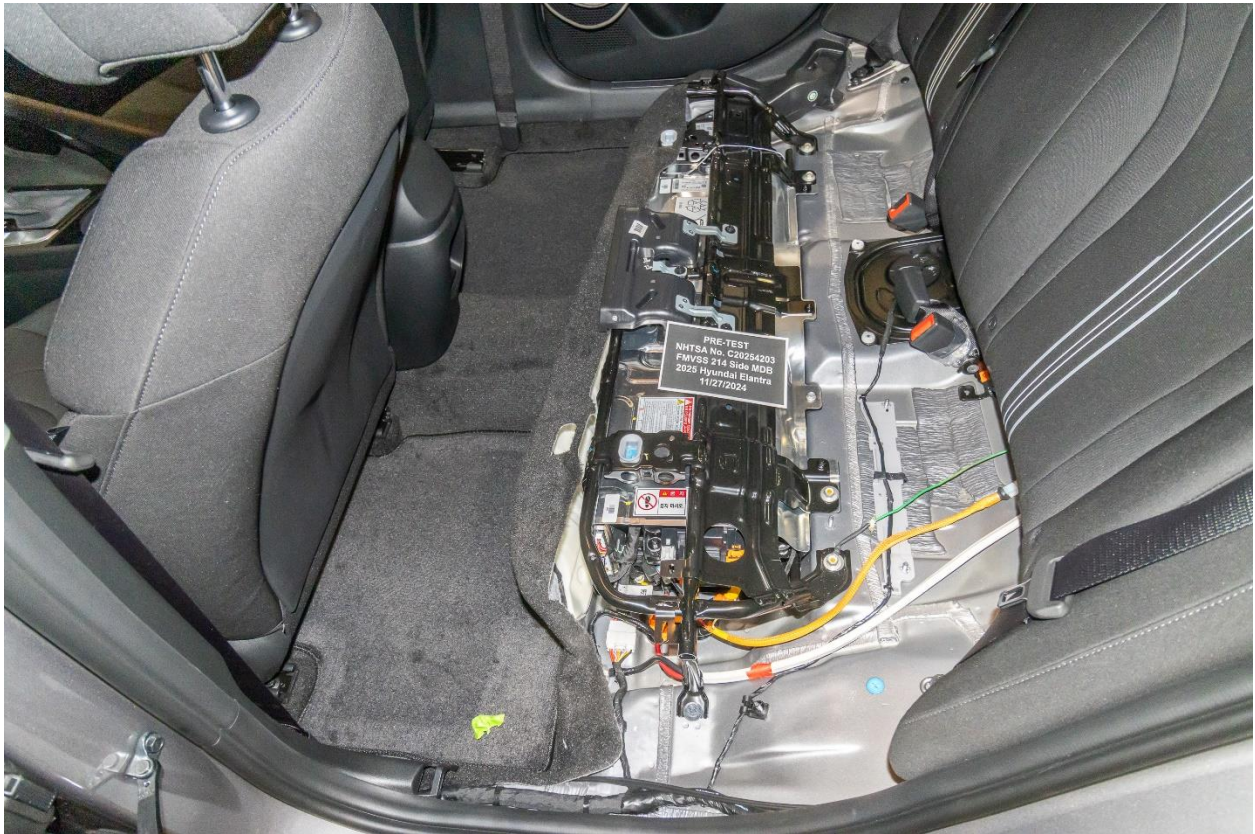
Figure 305-9: Pre-Impact View of Propulsion Battery
