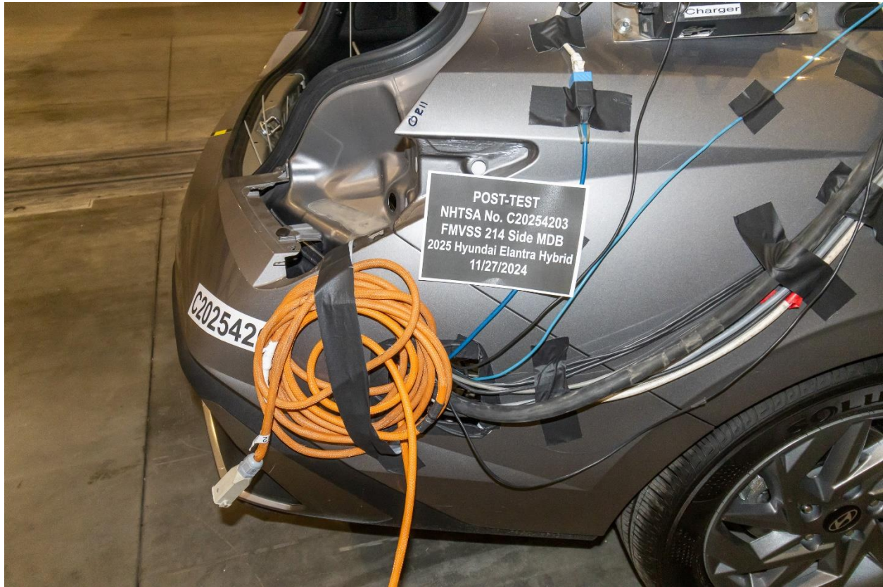
Figure 305-25: Post-Impact View of Installed Test Interface Port
