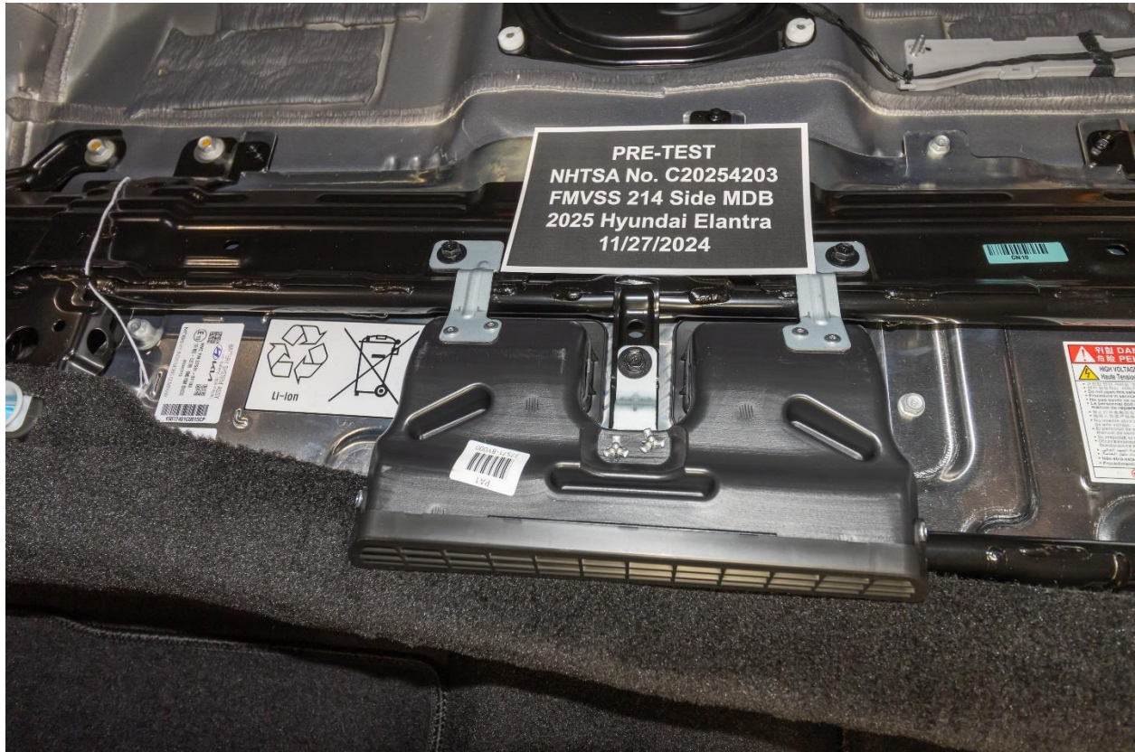
Figure 305-19: Pre-Impact View of Propulsion Battery Venting System
