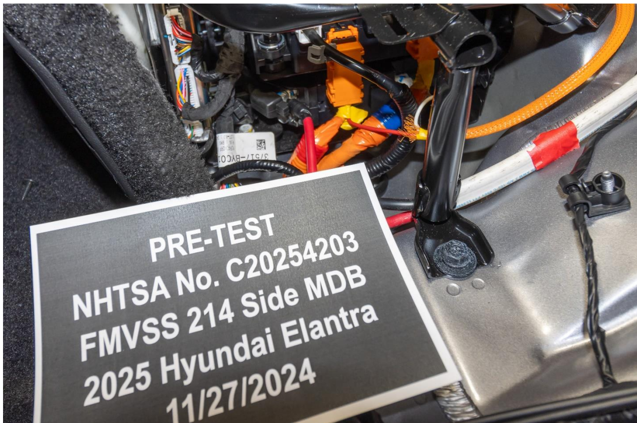
Figure 305-22: Pre-Impact View of High Voltage Leads Attached
