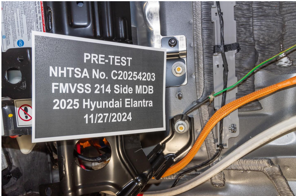
Figure 305-21: Pre-Impact View of Ground Lead Attached
