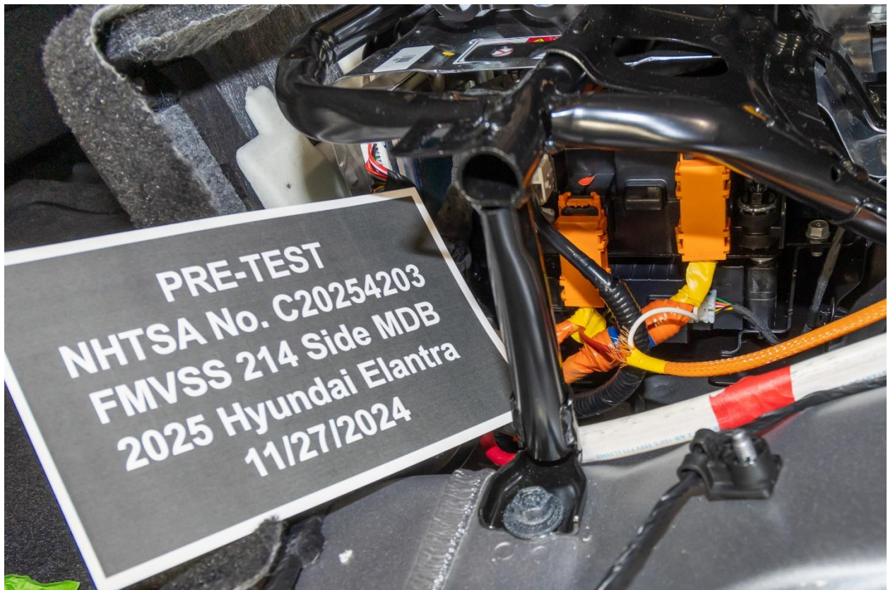
Figure 305-18: Pre-Impact View of High Voltage Interconnects
