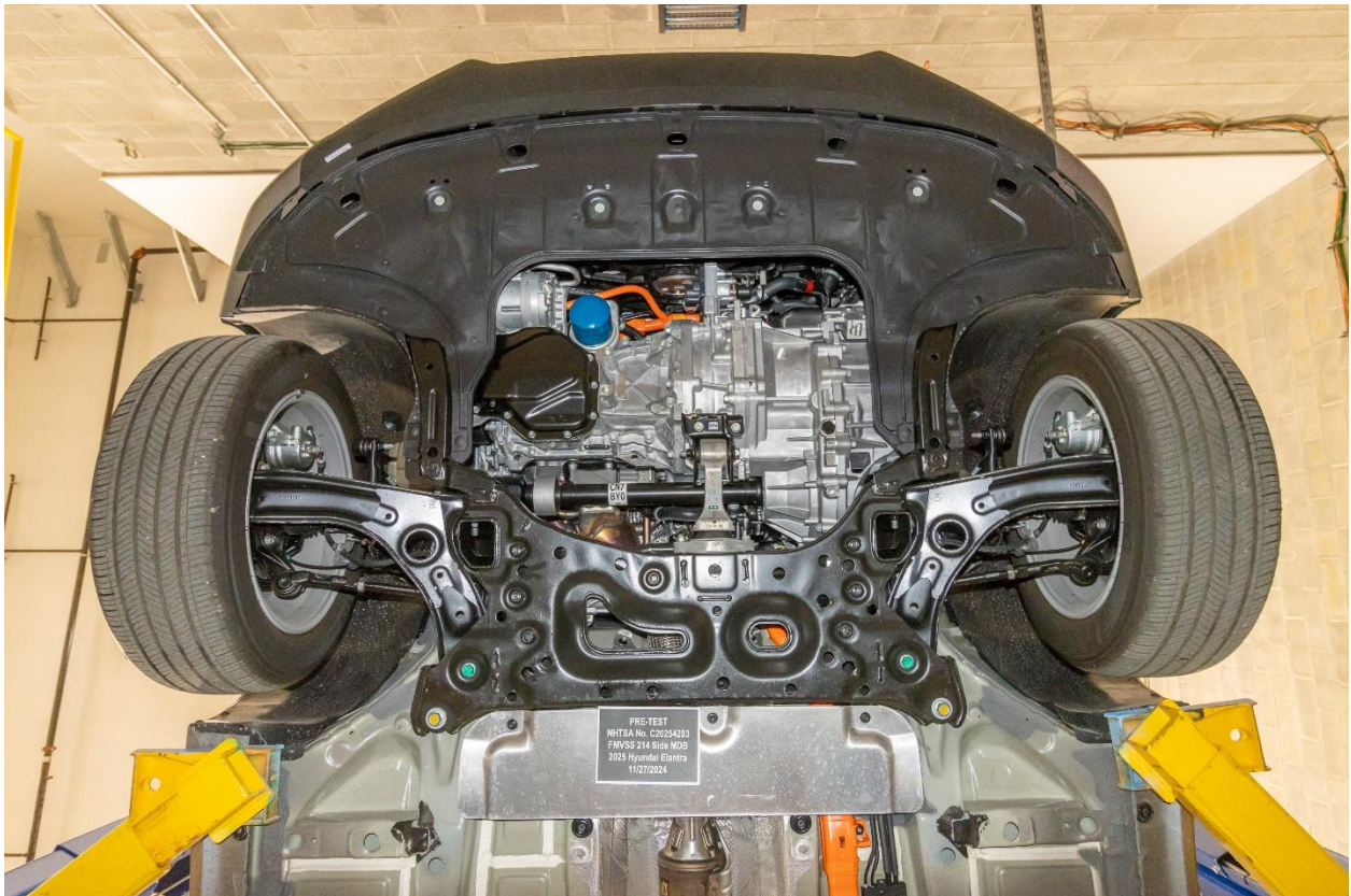
Figure 305-16: Pre-Impact View of Electric Propulsion Drive
