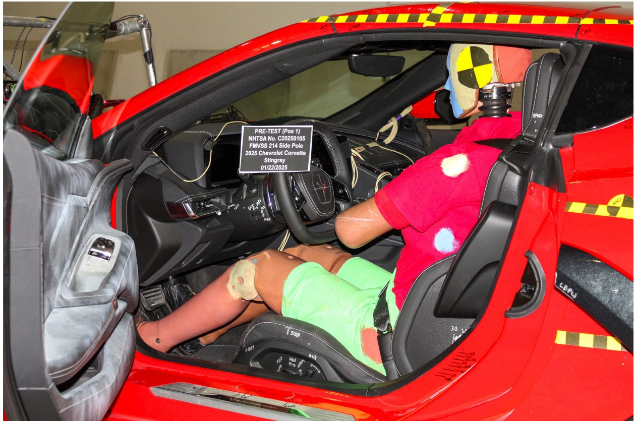
Figure A-15: Pre-Test Dummy with Door Open
