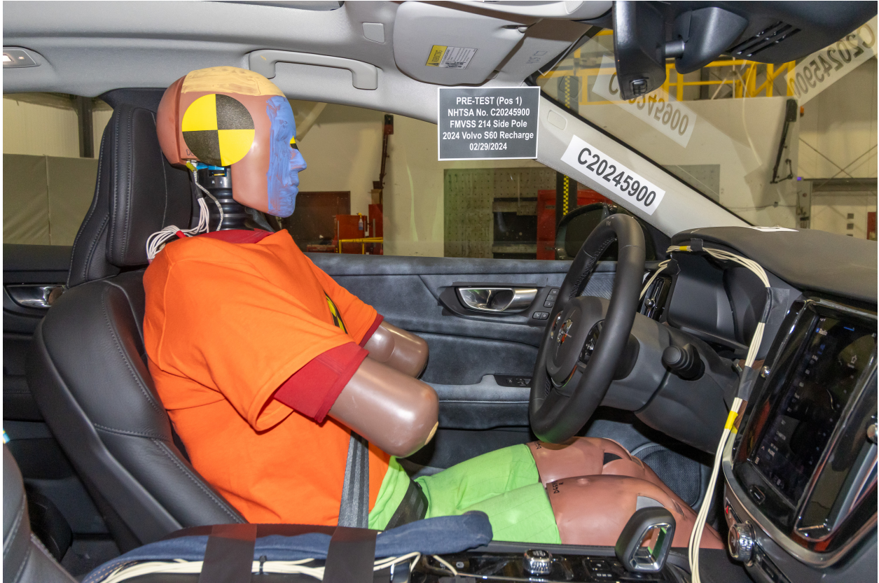
Figure A-11: Pre-Test Dummy Through Opposite Window
