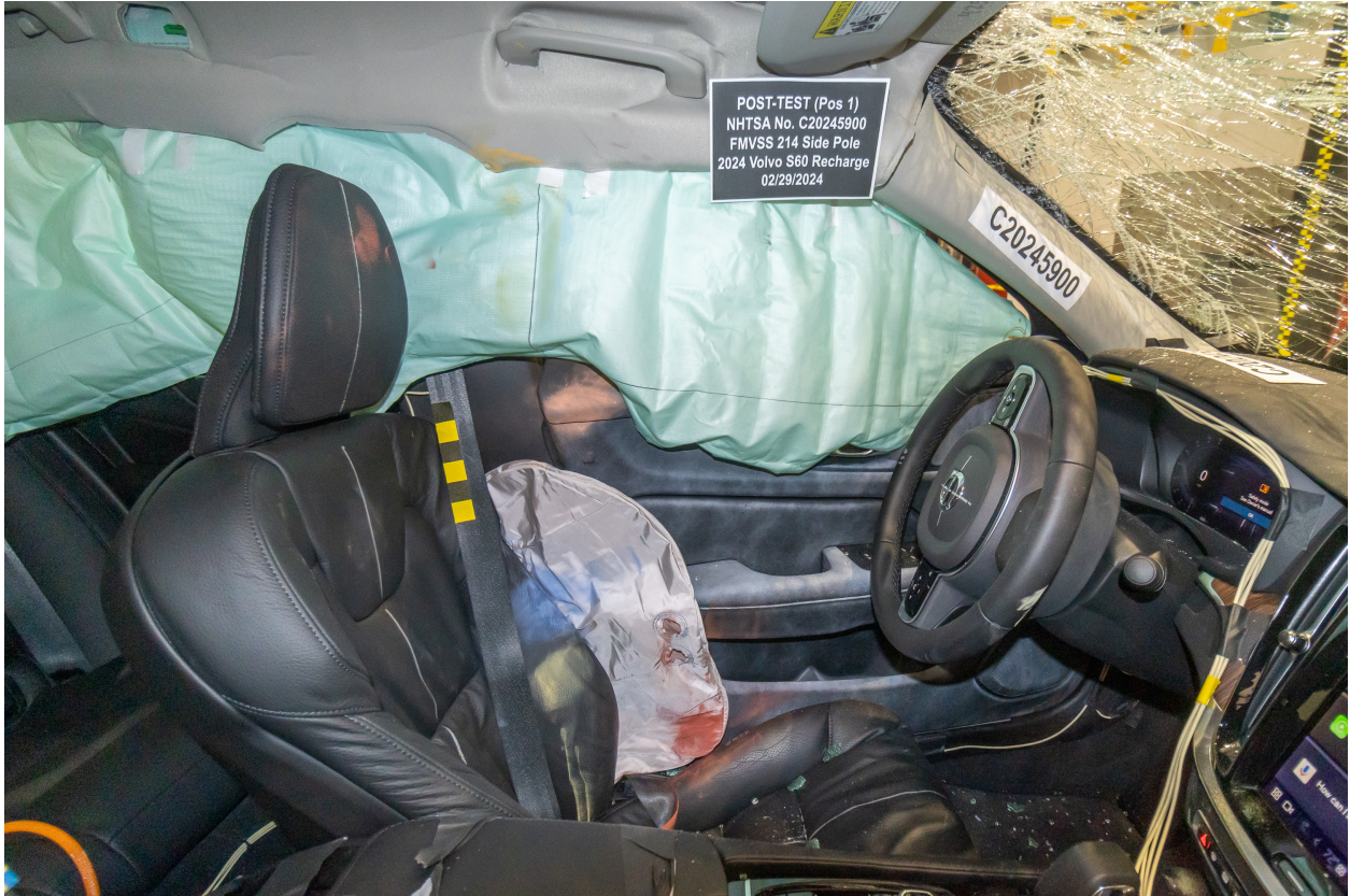
Figure A-19: Post-Test Interior of Front Door Showing Dummy Impact Locations
