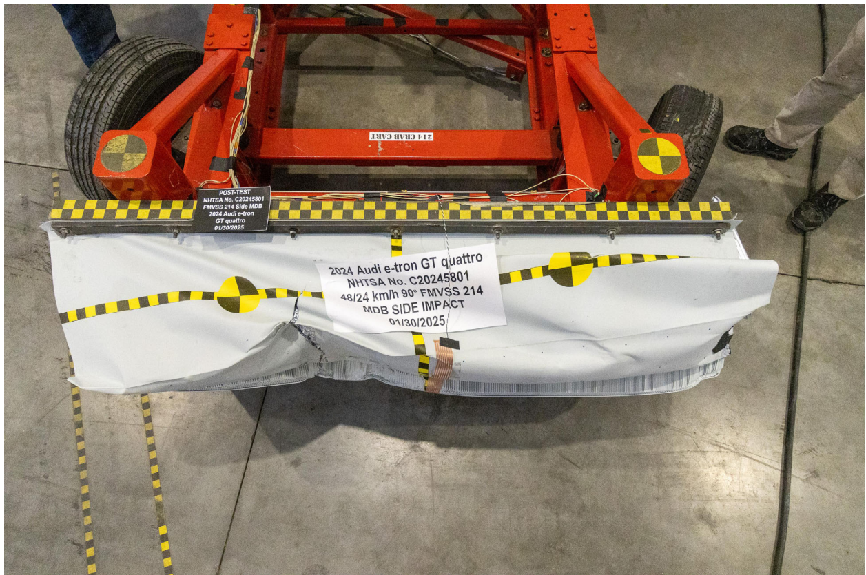
Figure A-14: Post-Test Top View of Impactor Face
