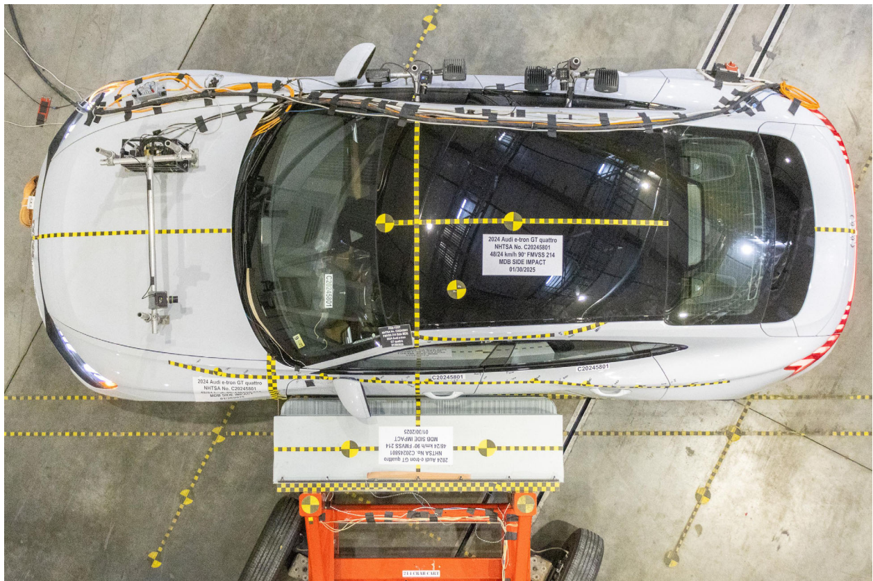
Figure A-15: Pre-Test Overhead View of MDB Positioned Against Impact Side of Test Vehicle at Impact Location
