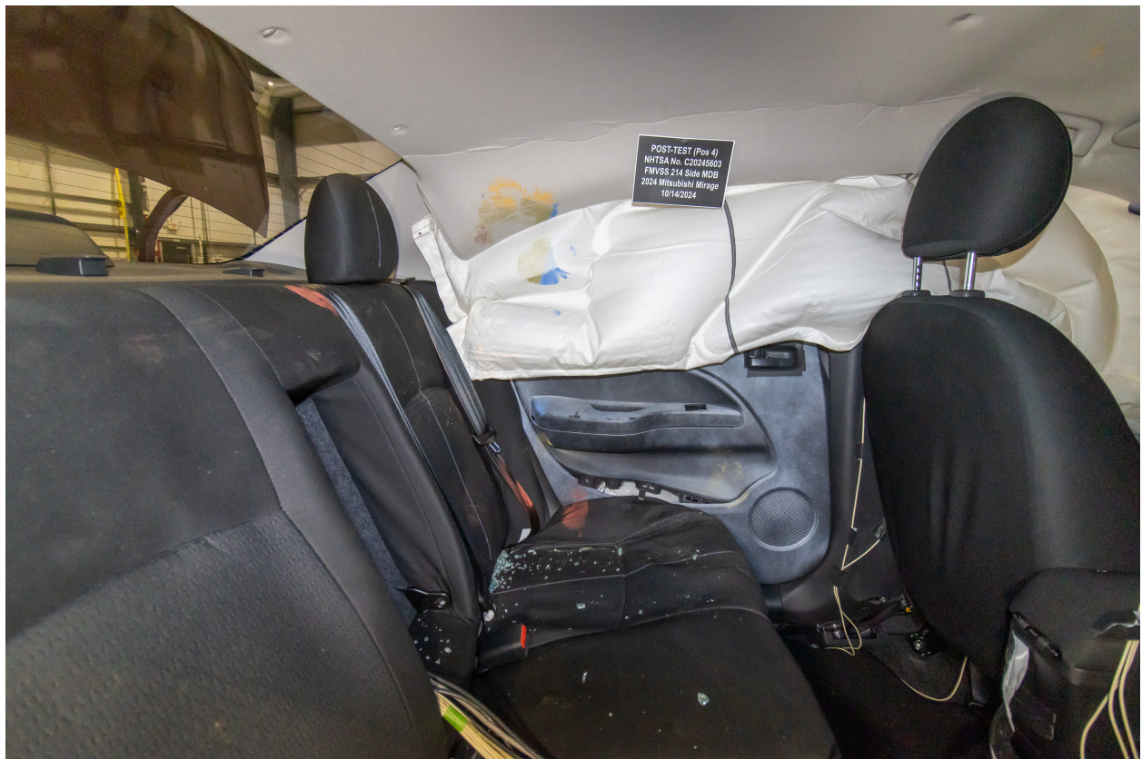
Figure A-29: Post-Test Rear Seat Occupant Area Showing Head & Torso Contact Regions
