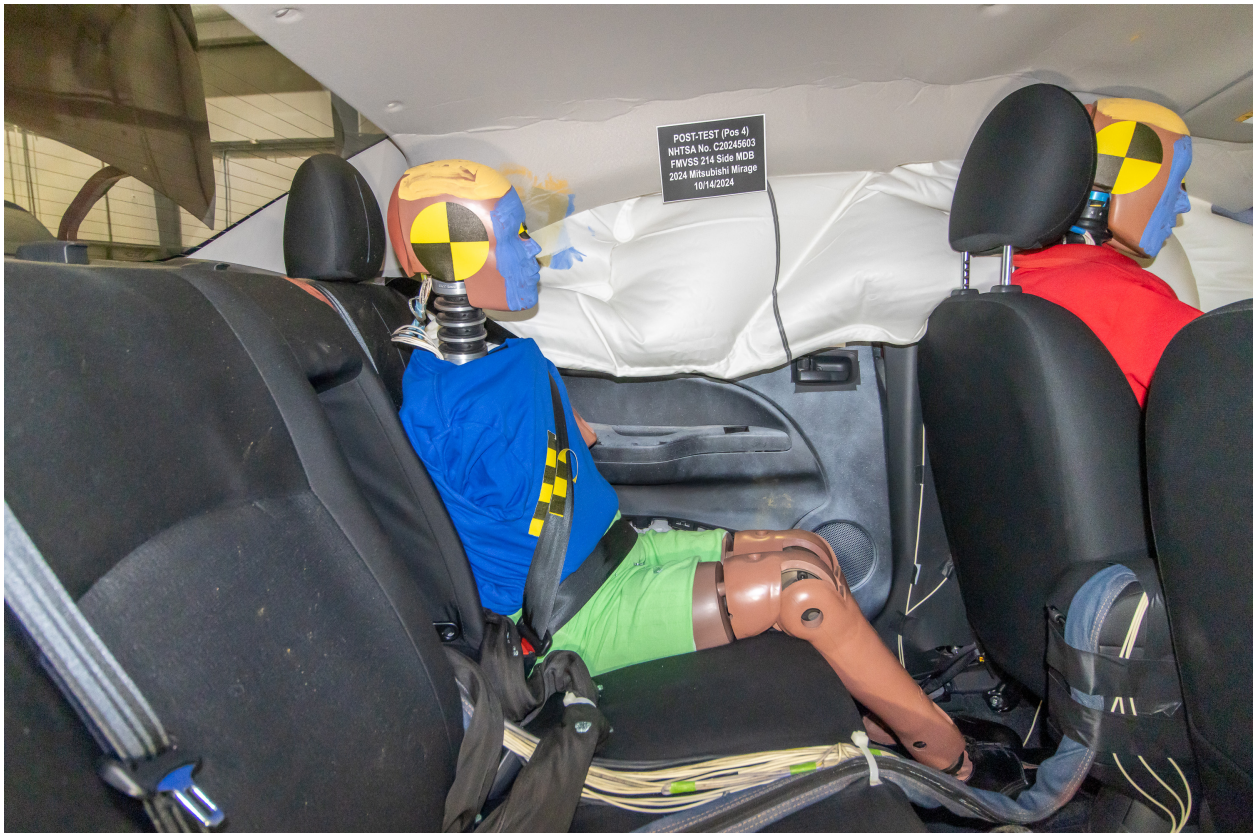
Figure A-24: Post-Test Rear SID - Opposite Side View
