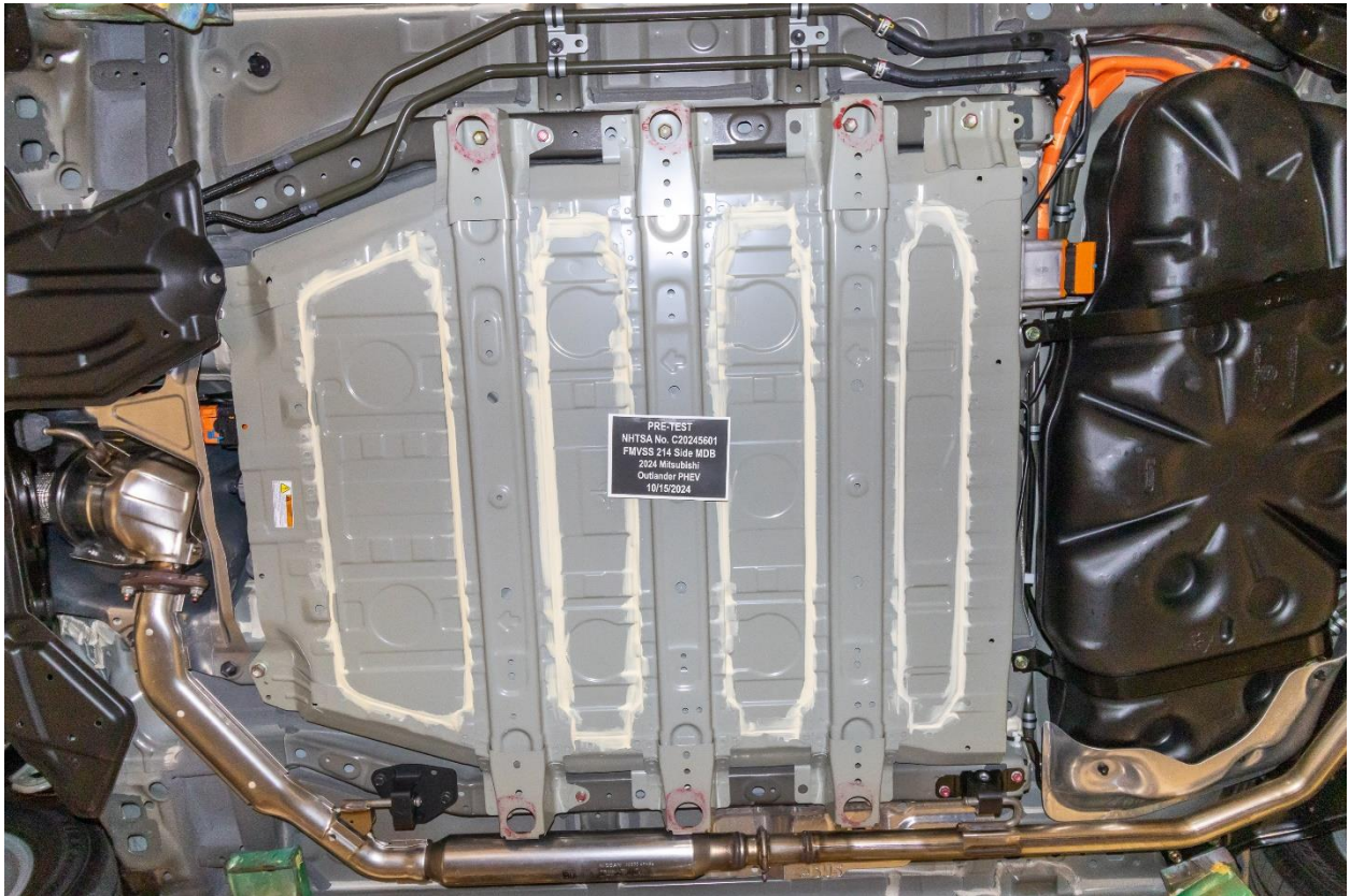
Figure 305-9: Pre-Impact View of Propulsion Battery
