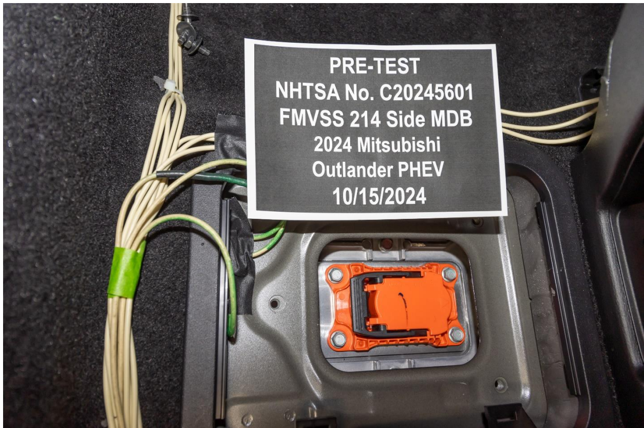
Figure 305-6: Manual High Voltage Service Disconnect in Place
