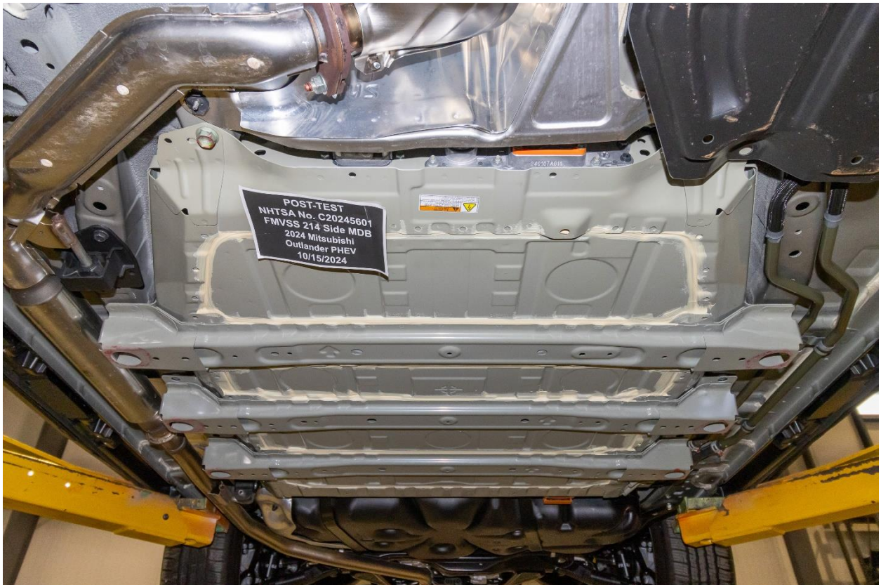
Figure 305-10: Post-Impact Front View of Propulsion Battery
