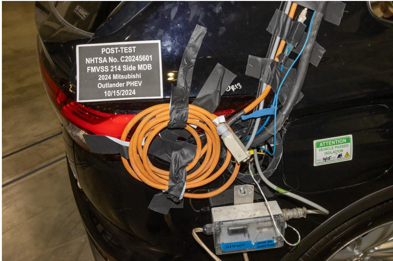
Figure 305-25: Post-Impact View of Installed Test Interface Port
