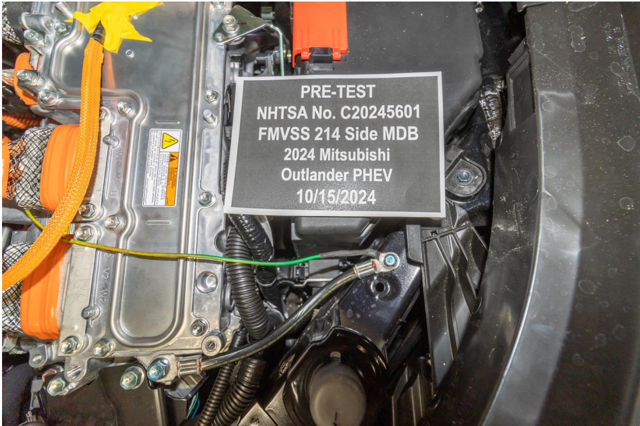
Figure 305-21: Pre-Impact View of Ground Lead Attached
