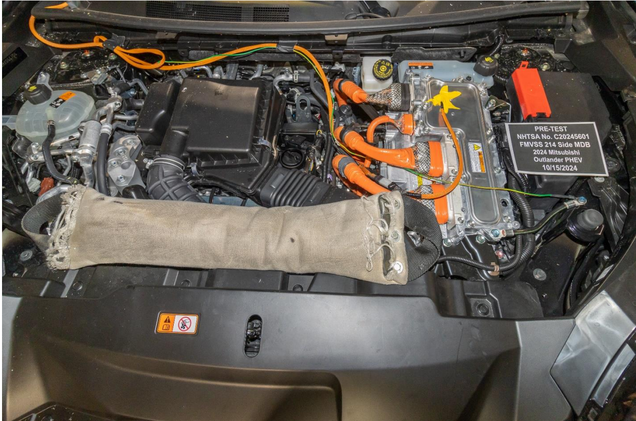
Figure 305-22: Pre-Impact View of High Voltage Leads Attached
