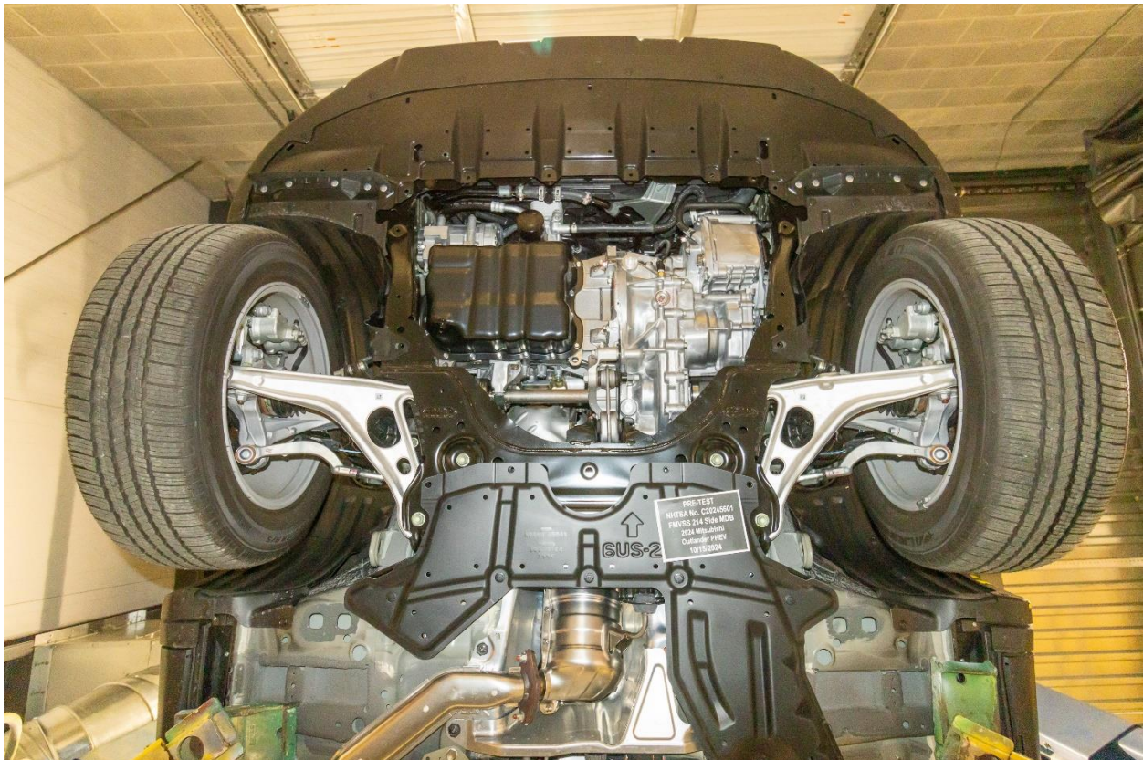
Figure 305-16: Pre-Impact View of Electric Propulsion Drive
