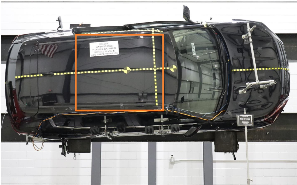
Figure 305-30: FMVSS No. 305 Static Rollover 270 Degrees
