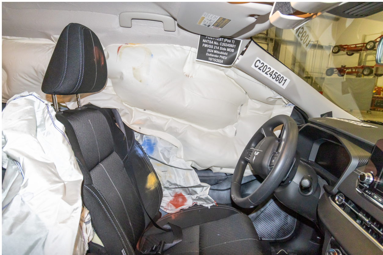
Figure A-28: Post-Test Front Seat Occupant Area Showing Head & Torso Contact Regions
