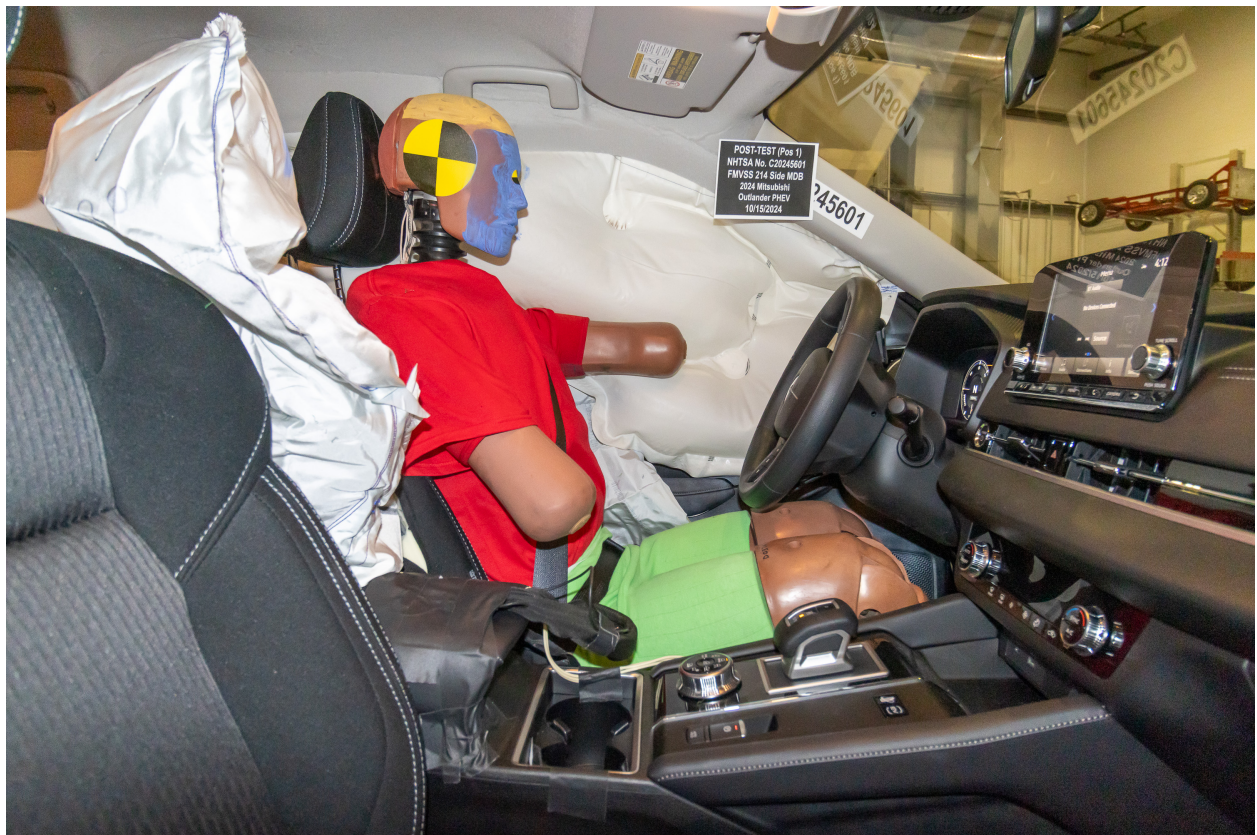
Figure A-20: Post-Test Front ES2-re - Opposite Side View
