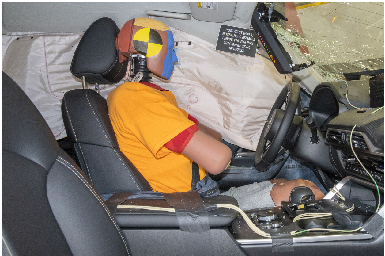
Figure A-12: Post-Test Dummy Through Opposite Window
