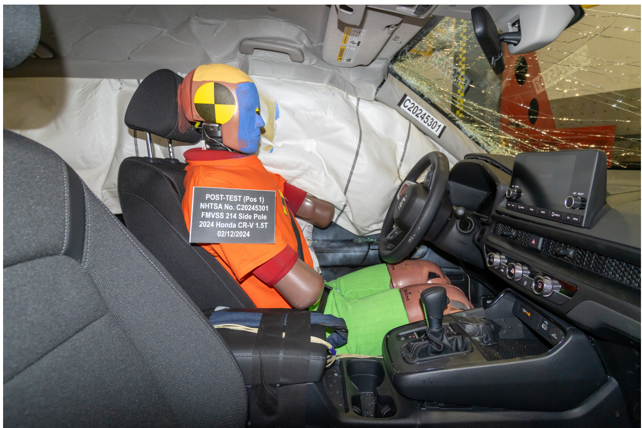
Figure A-12: Post-Test Dummy Through Opposite Window
