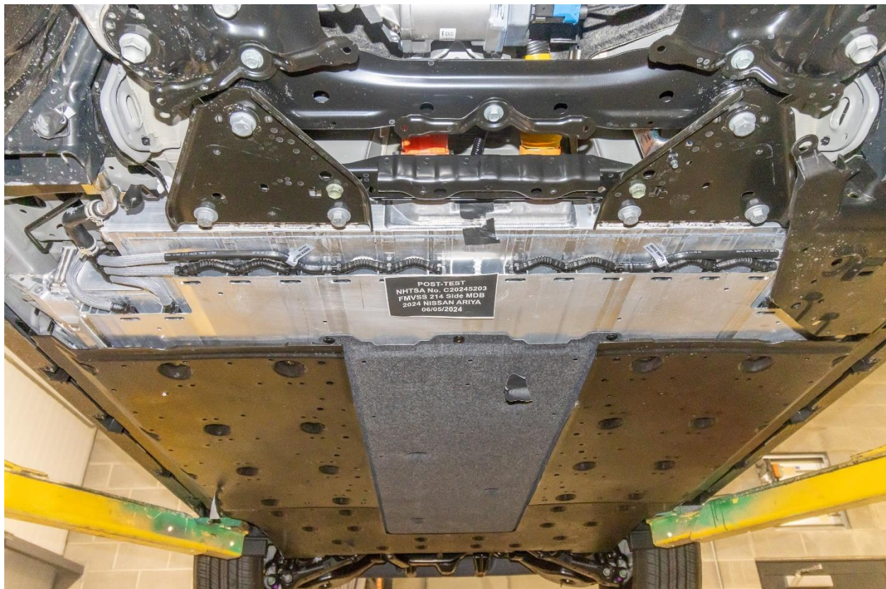
Figure 305-10: Post-Impact Front View of Propulsion Battery
