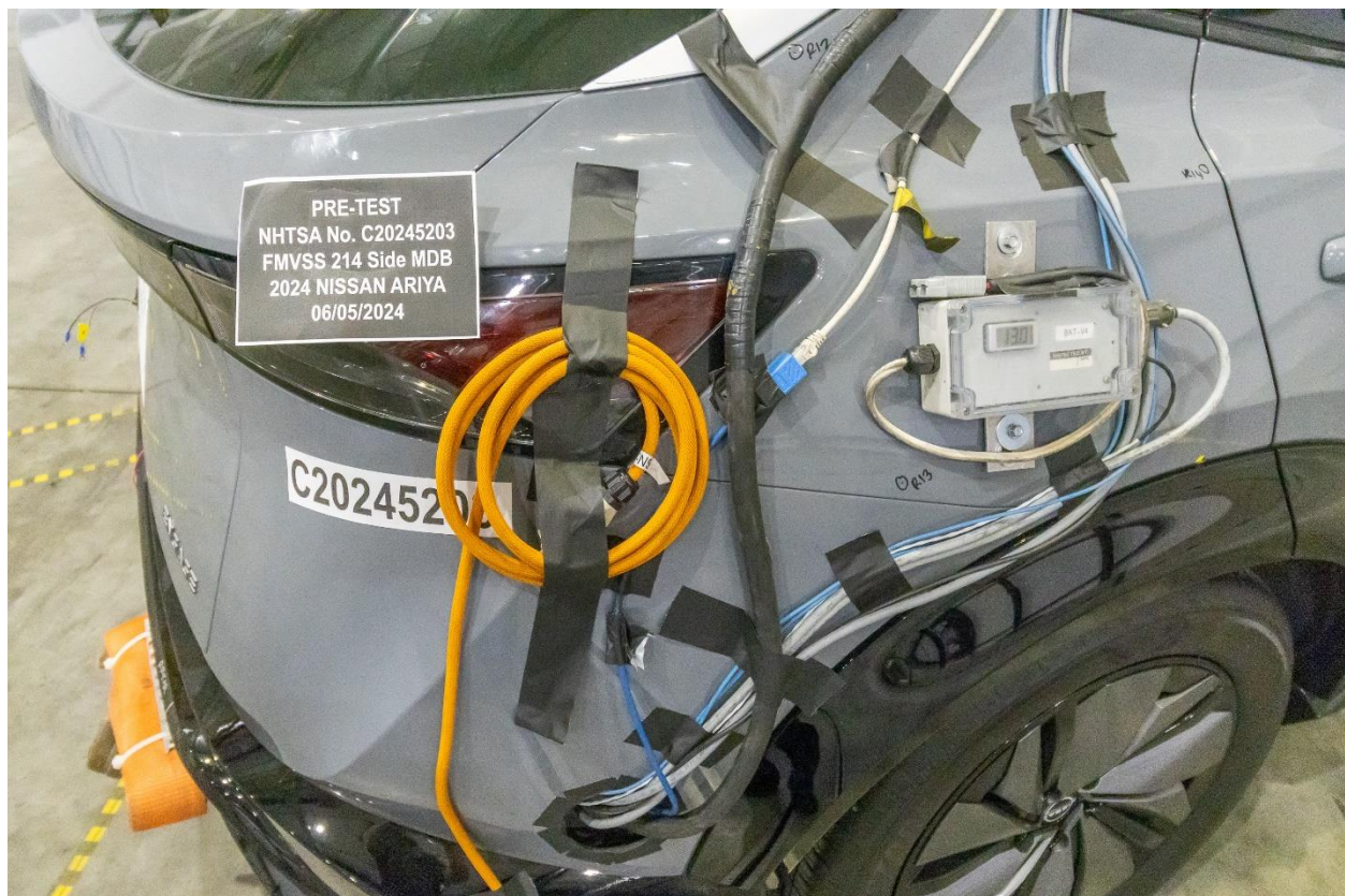
Figure 305-24: Pre-Impact View of Installed Test Interface Port
