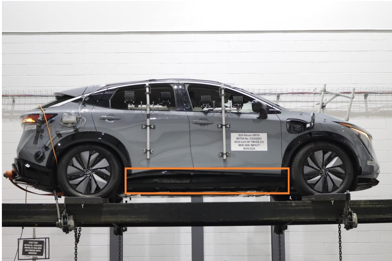
Figure 305-31: FMVSS No. 305 Static Rollover 360 Degrees
