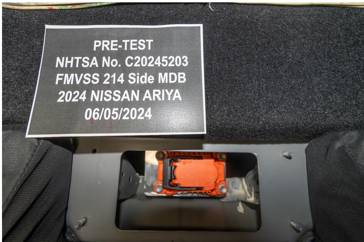
Figure 305-6: Manual High Voltage Service Disconnect in Place
