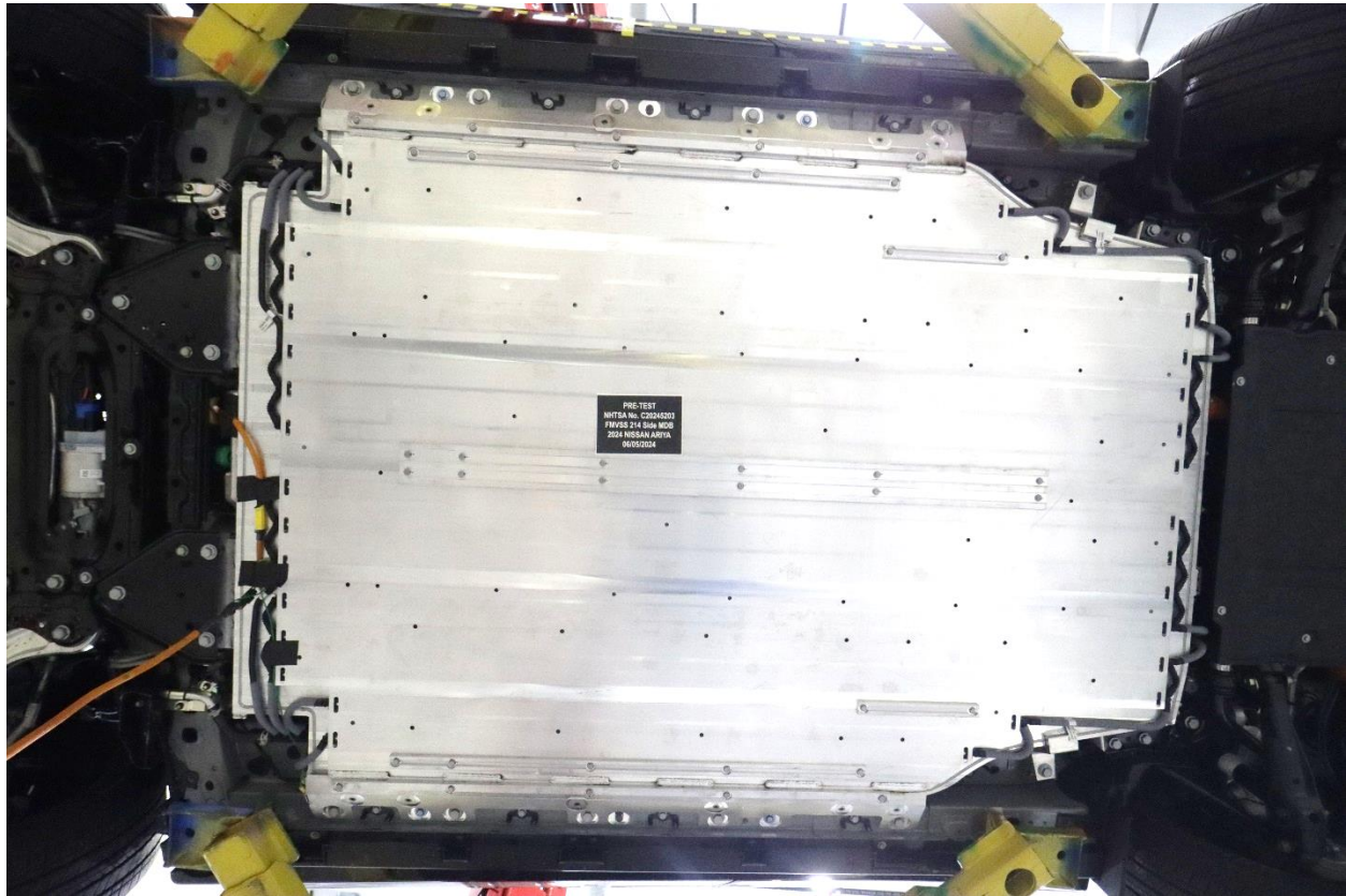
Figure 305-9: Pre-Impact View of Propulsion Battery
