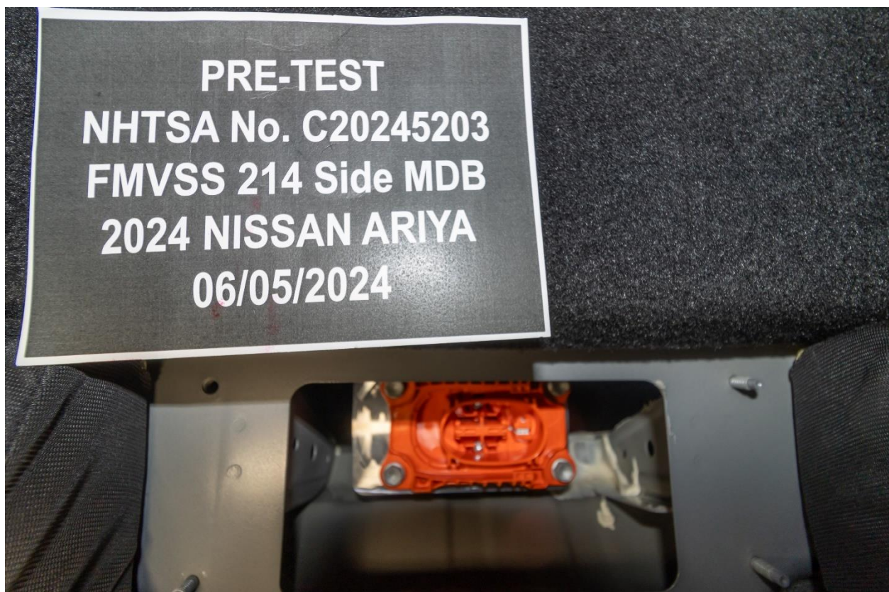
Figure 305-8: Manual High Voltage Service Disconnect Removed Location
