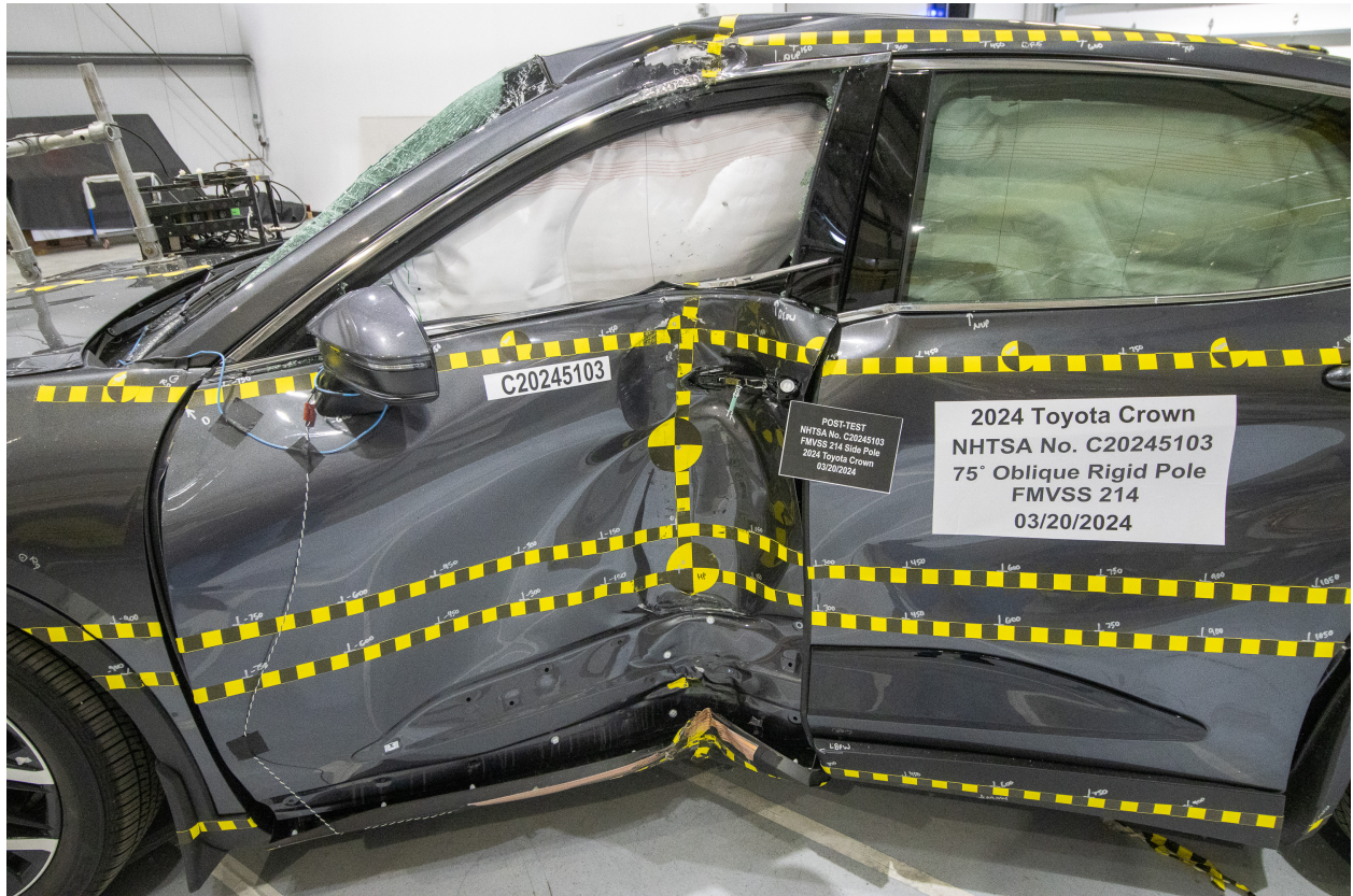
Figure A-21: Post-Test Impact Zone Close-Up View
