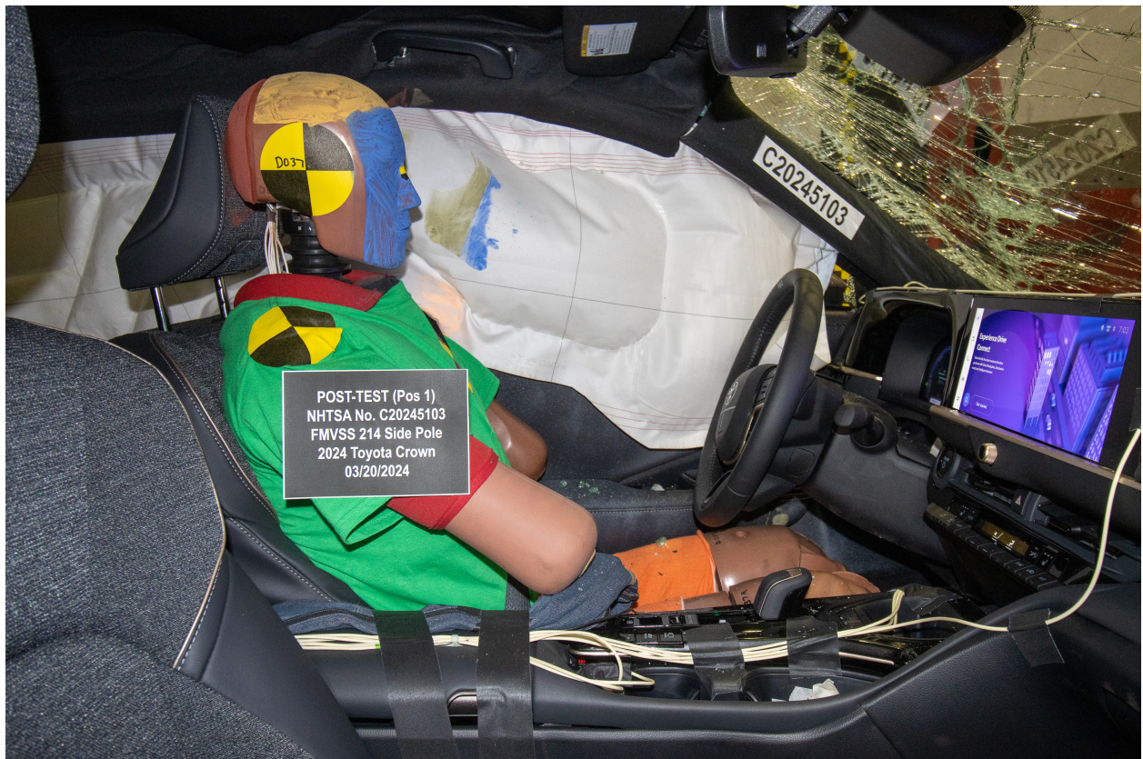
Figure A-12: Post-Test Dummy Through Opposite Window
