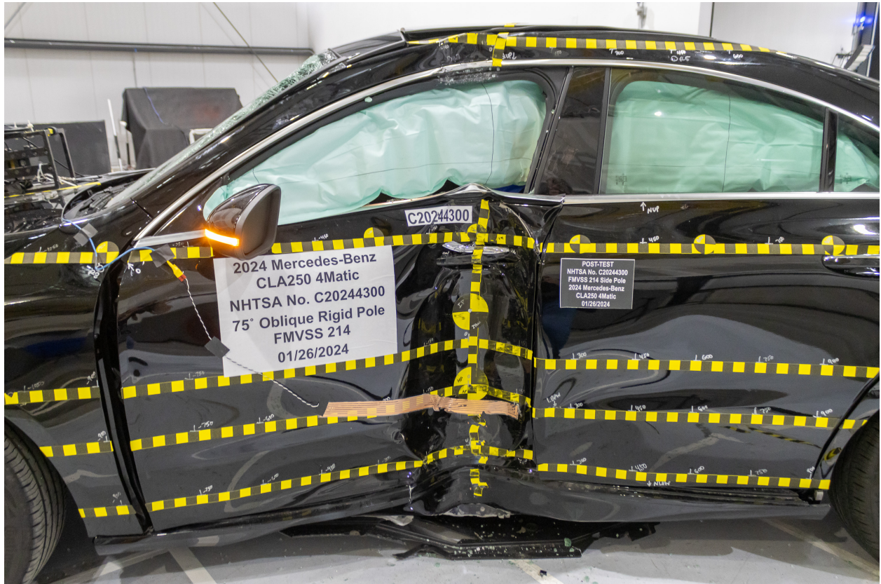
Figure A-21: Post-Test Impact Zone Close-Up View
