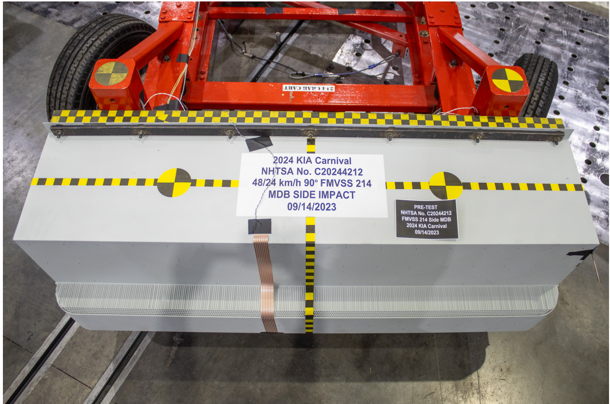
Figure A-13: Pre-Test Top View of Impactor Face
