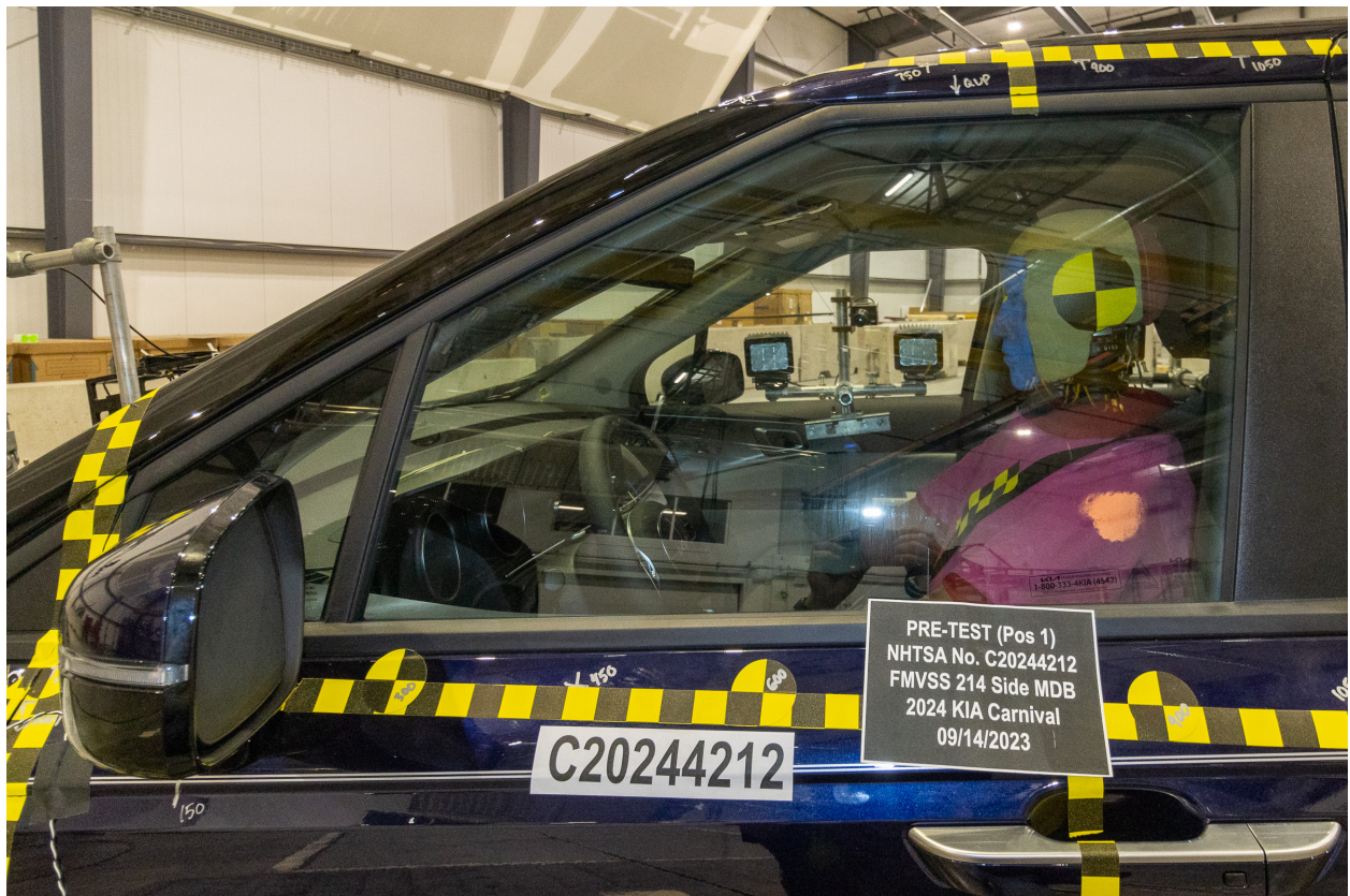
Figure A-18: Pre-Test Front ES2-re in Final Seating Position (Door Closed)
