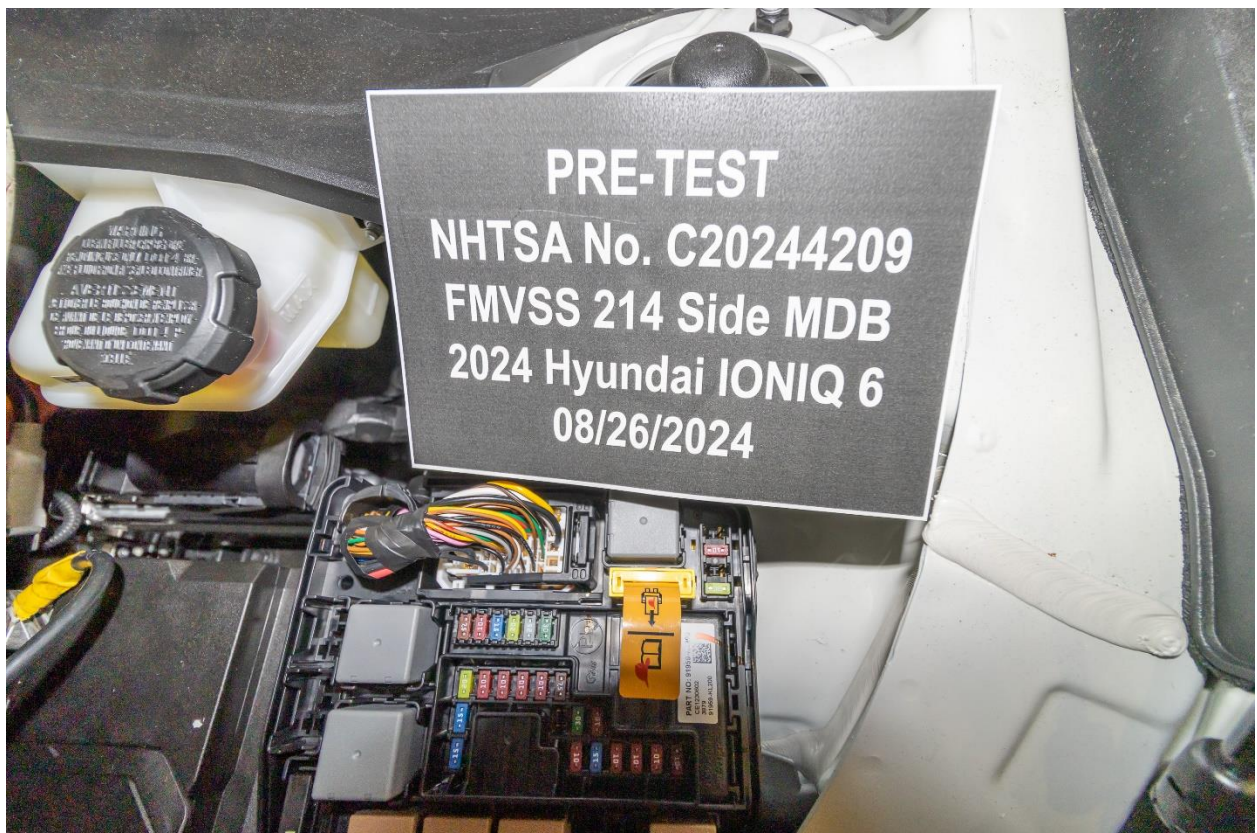
Figure 305-8: Manual High Voltage Service Disconnect Removed Location
