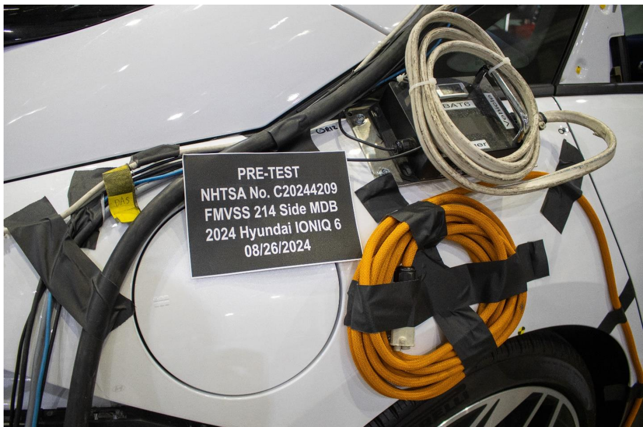
Figure 305-24: Pre-Impact View of Installed Test Interface Port
