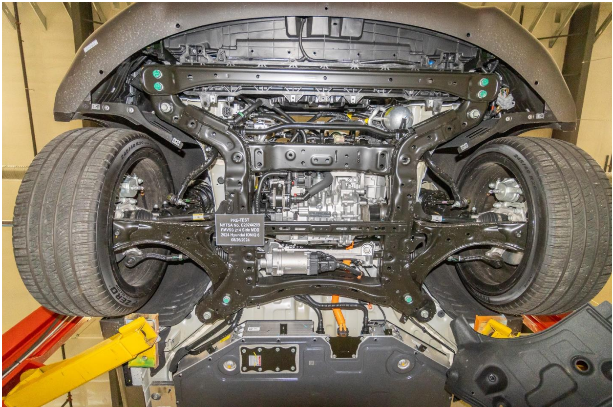
Figure 305-16: Pre-Impact View of Electric Propulsion Drive
