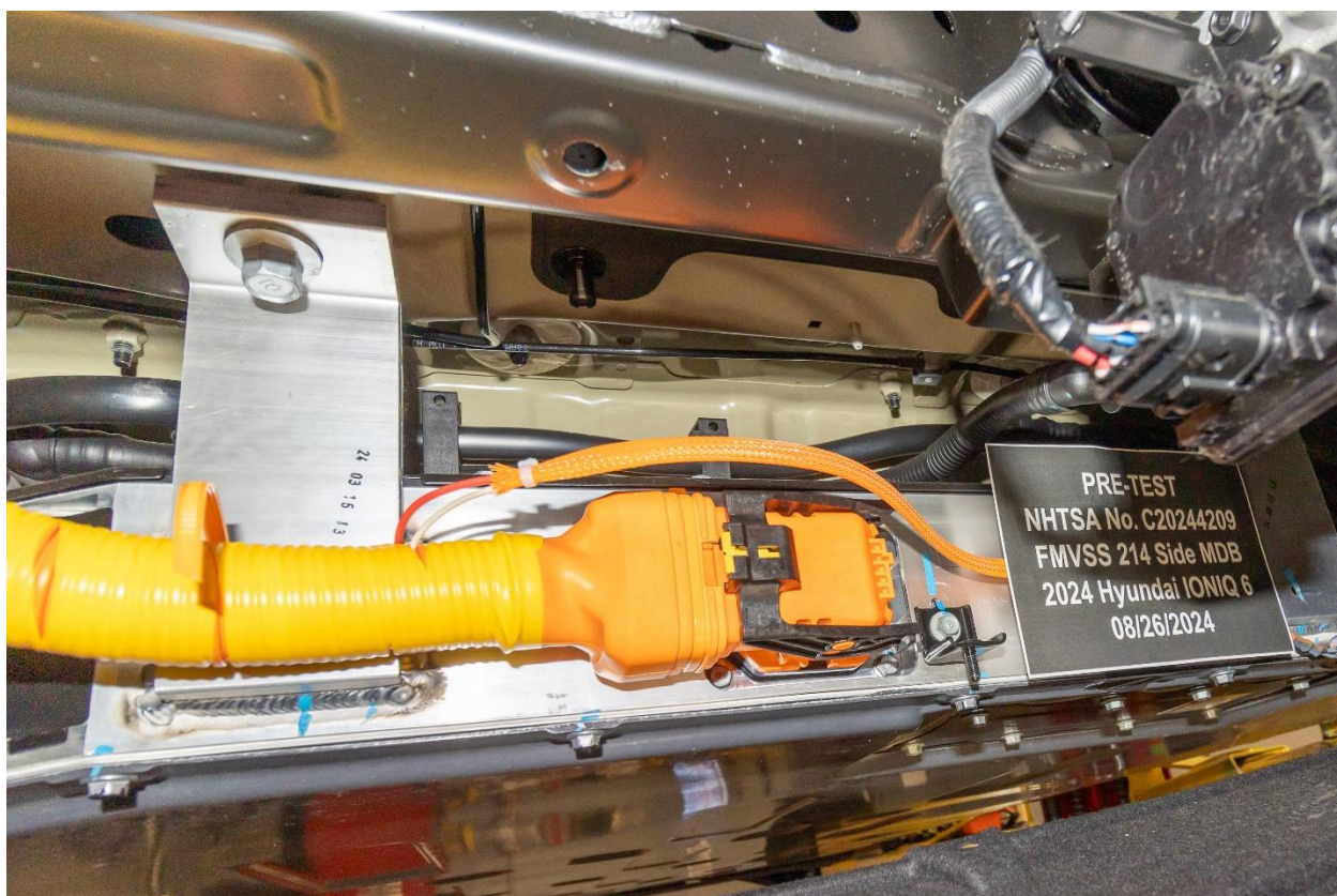
Figure 305-18: Pre-Impact View of High Voltage Interconnects
