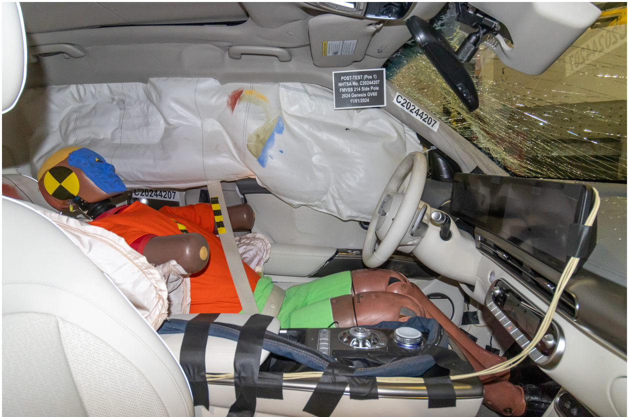
Figure A-12: Post-Test Dummy Through Opposite Window
