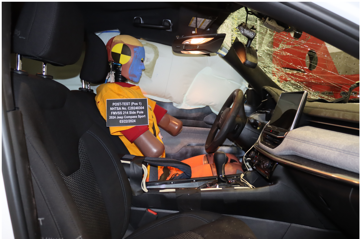
Figure A-12: Post-Test Dummy Through Opposite Window
