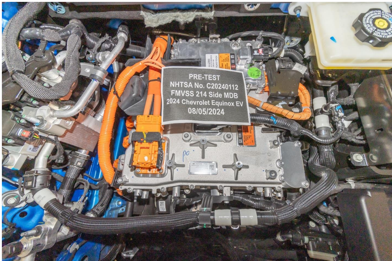
Figure 305-18: Pre-Impact View of High Voltage Interconnects
