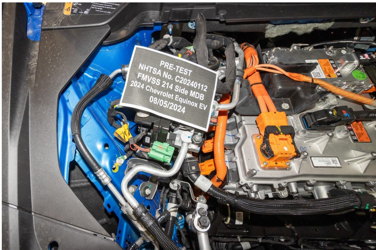
Figure 305-8: Manual High Voltage Service Disconnect Removed Location
