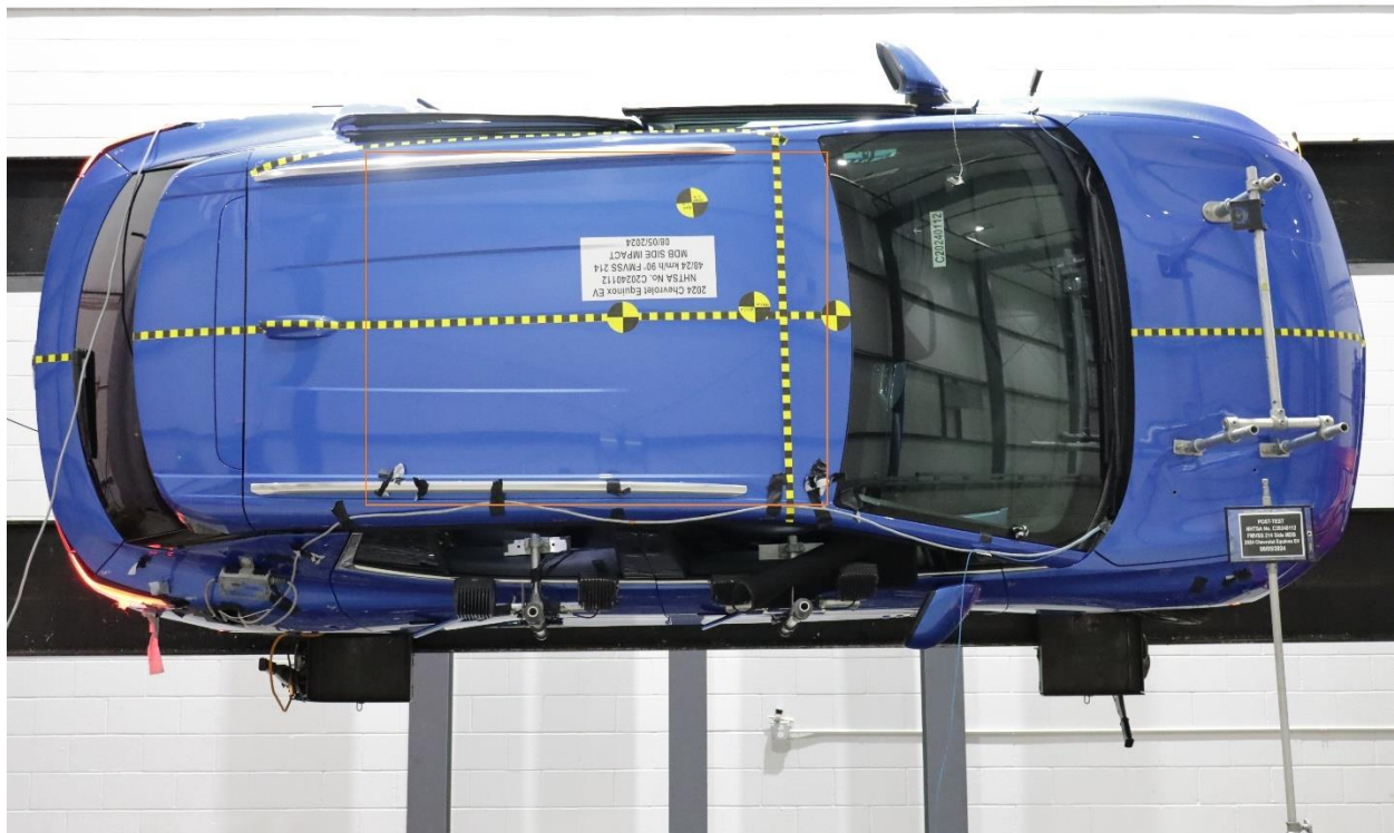
Figure 305-30: FMVSS No. 305 Static Rollover 270 Degrees
