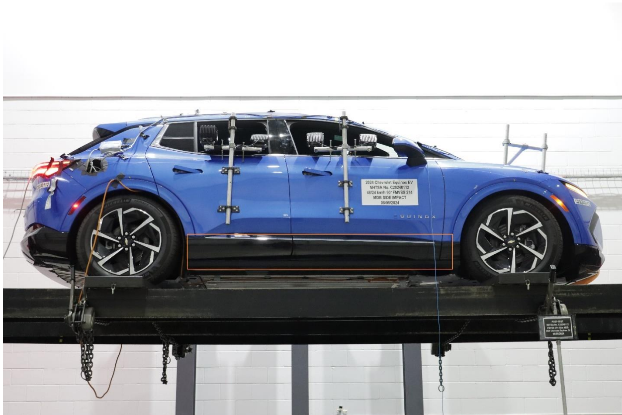
Figure 305-31: FMVSS No. 305 Static Rollover 360 Degrees
