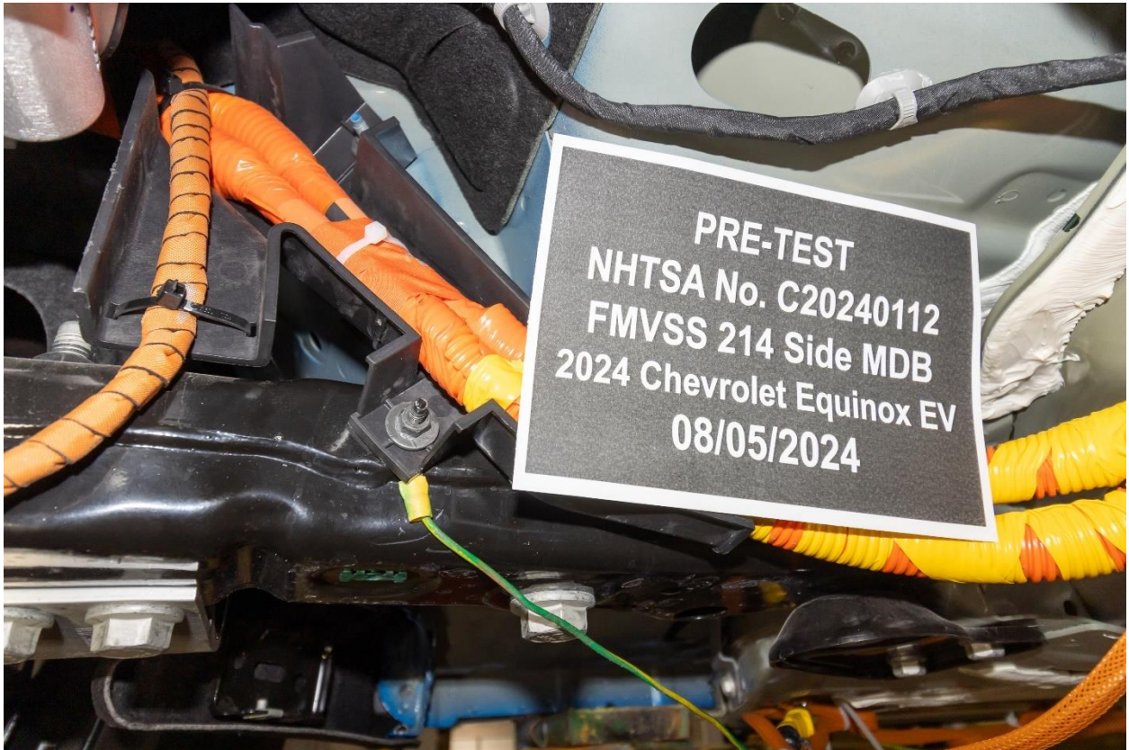
Figure 305-21: Pre-Impact View of Ground Lead Attached
