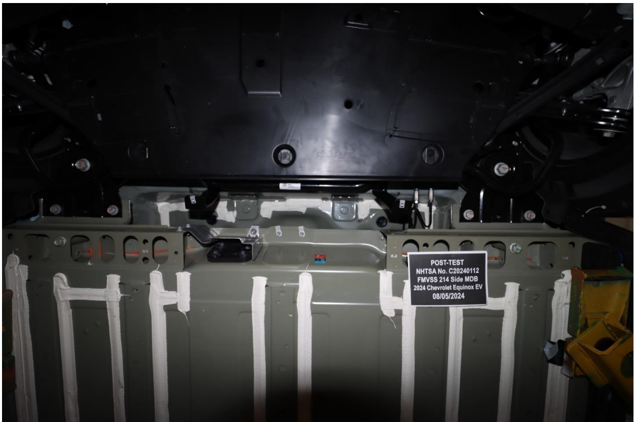
Figure 305-10: Post-Impact Front View of Propulsion Battery
