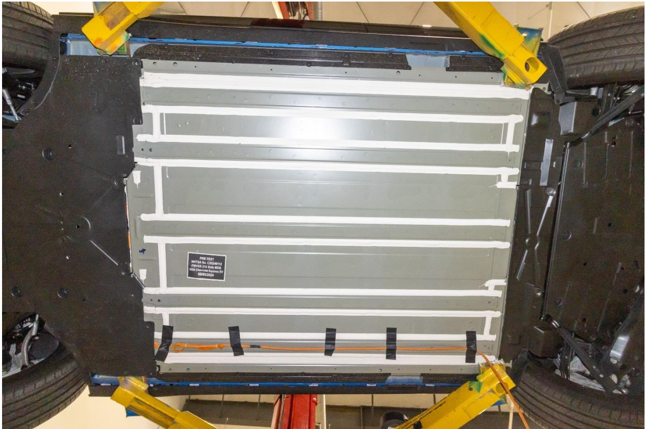
Figure 305-9: Pre-Impact View of Propulsion Battery
