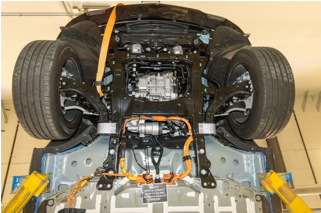
Figure 305-16: Pre-Impact View of Electric Propulsion Drive
