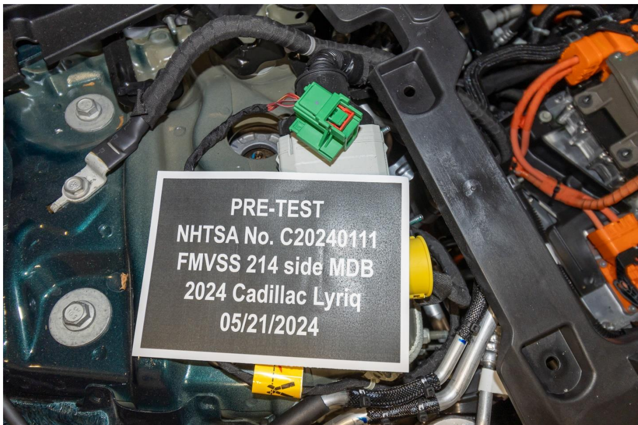
Figure 305-6: Manual High Voltage Service Disconnect in Place
