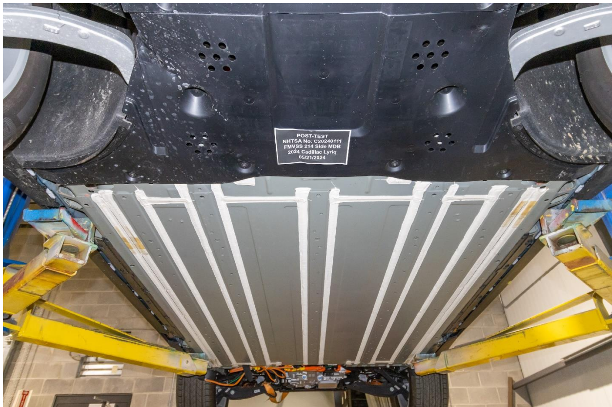
Figure 305-10: Post-Impact Front View of Propulsion Battery
