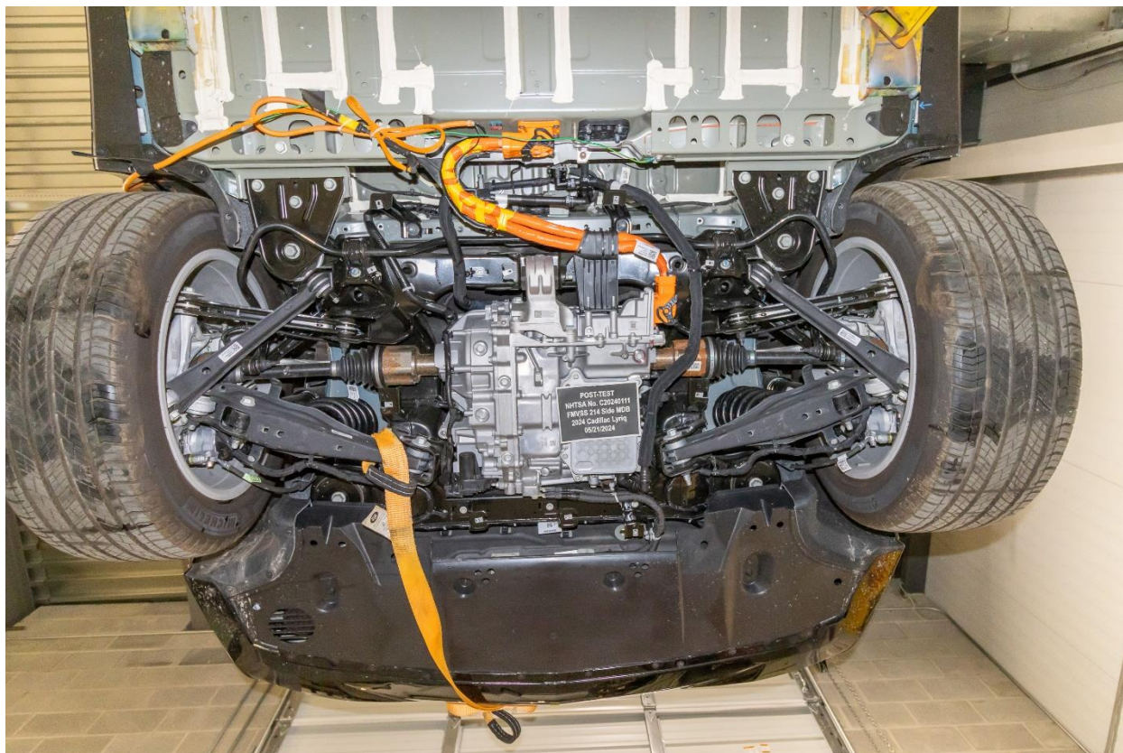
Figure 305-17: Post-Impact View of Electric Propulsion Drive
