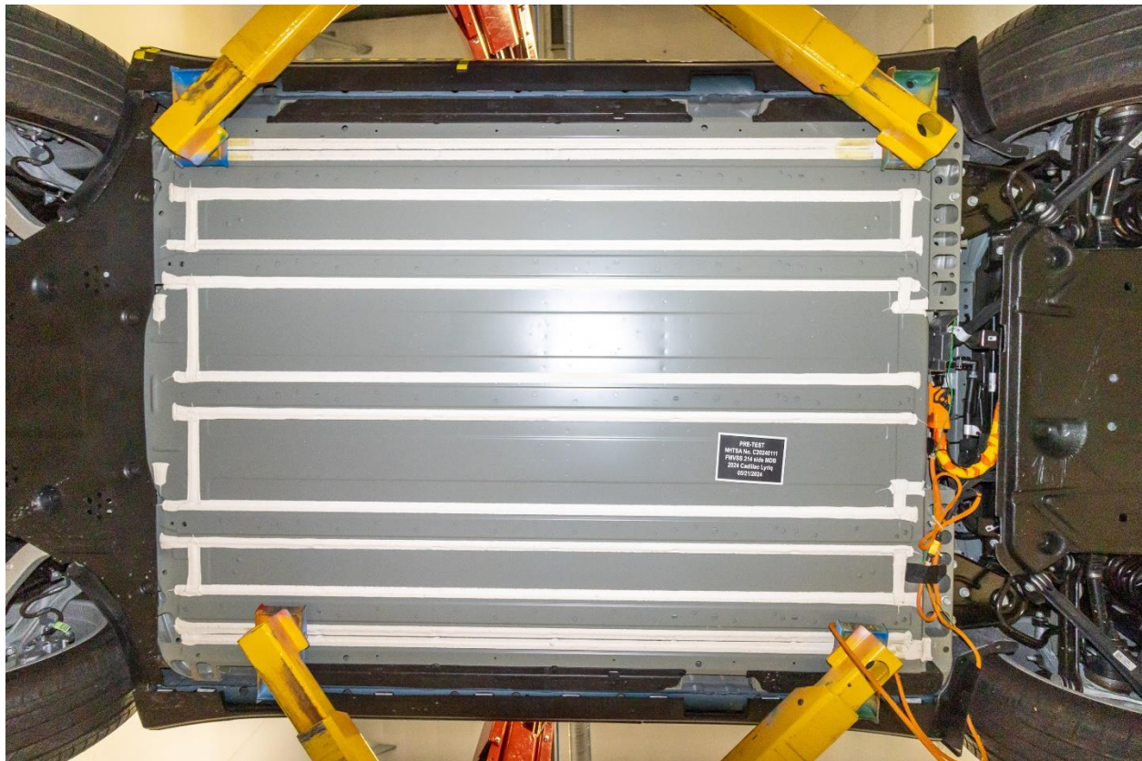
Figure 305-9: Pre-Impact View of Propulsion Battery
