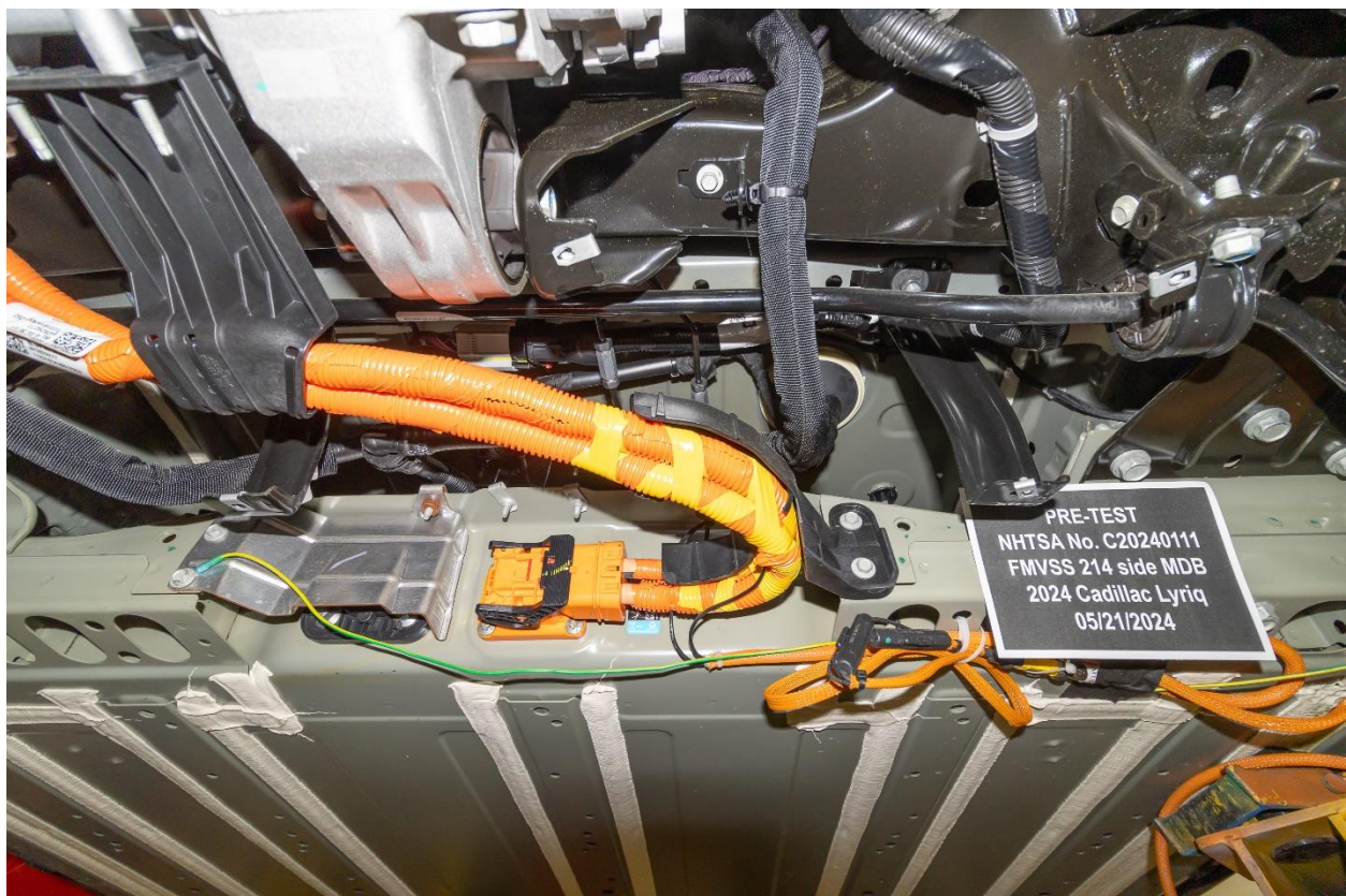
Figure 305-22: Pre-Impact View of High Voltage Leads Attached
