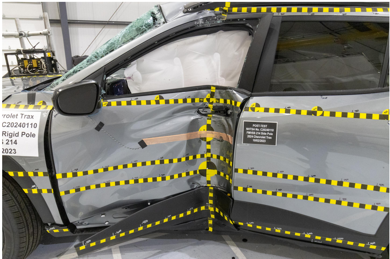
Figure A-21: Post-Test Impact Zone Close-Up View
