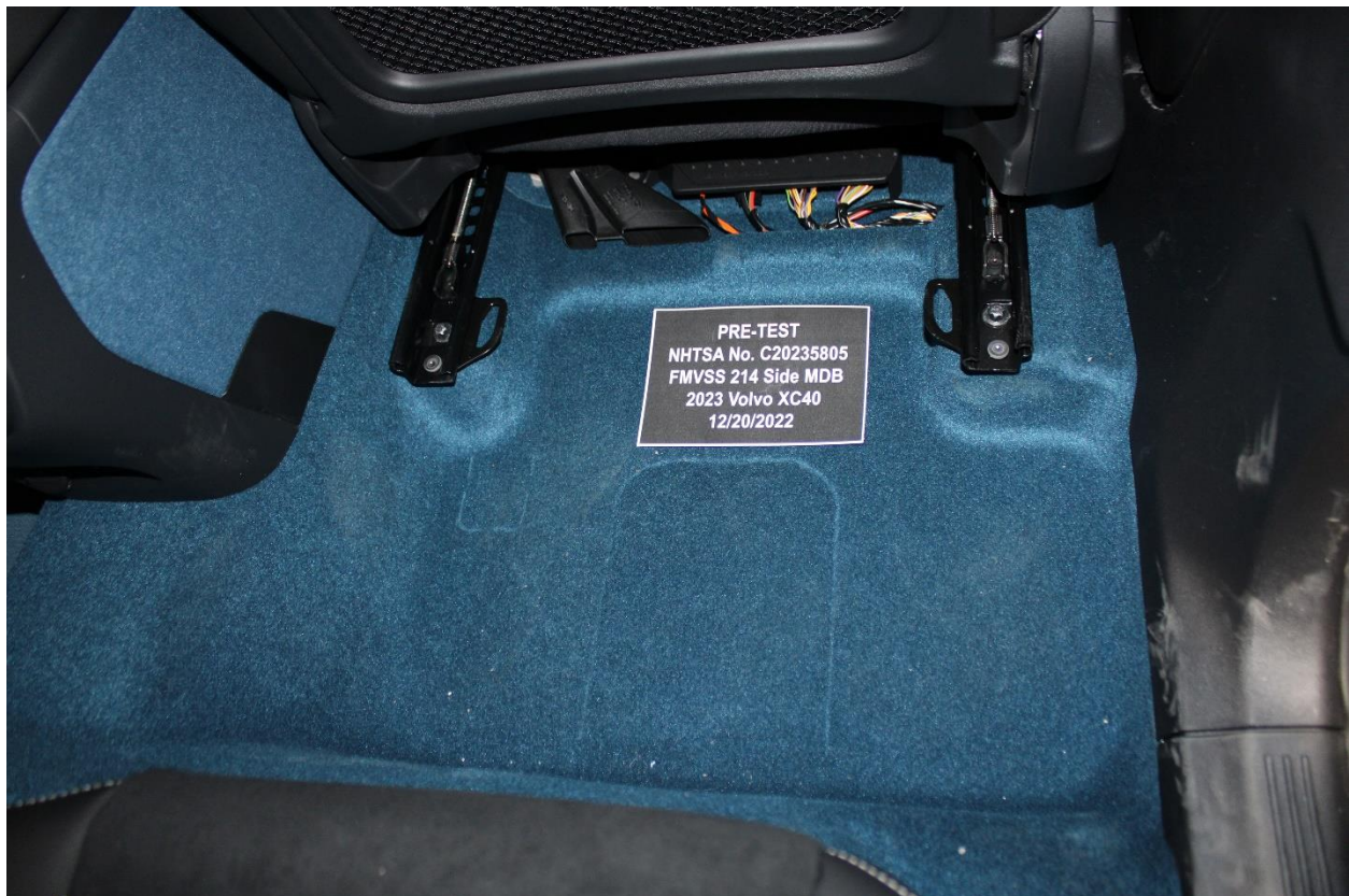
Figure 305-8: Manual High Voltage Service Disconnect Removed Location
