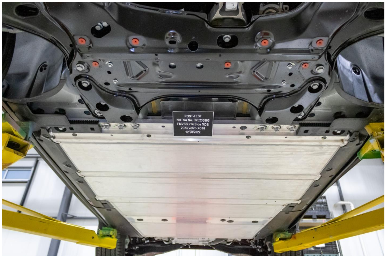
Figure 305-10: Post-Impact Front View of Propulsion Battery
