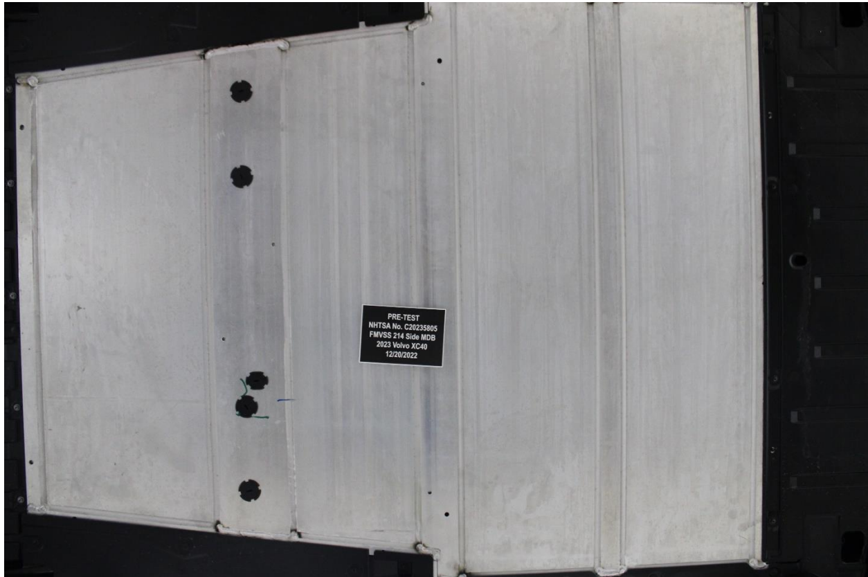
Figure 305-9: Pre-Impact View of Propulsion Battery
