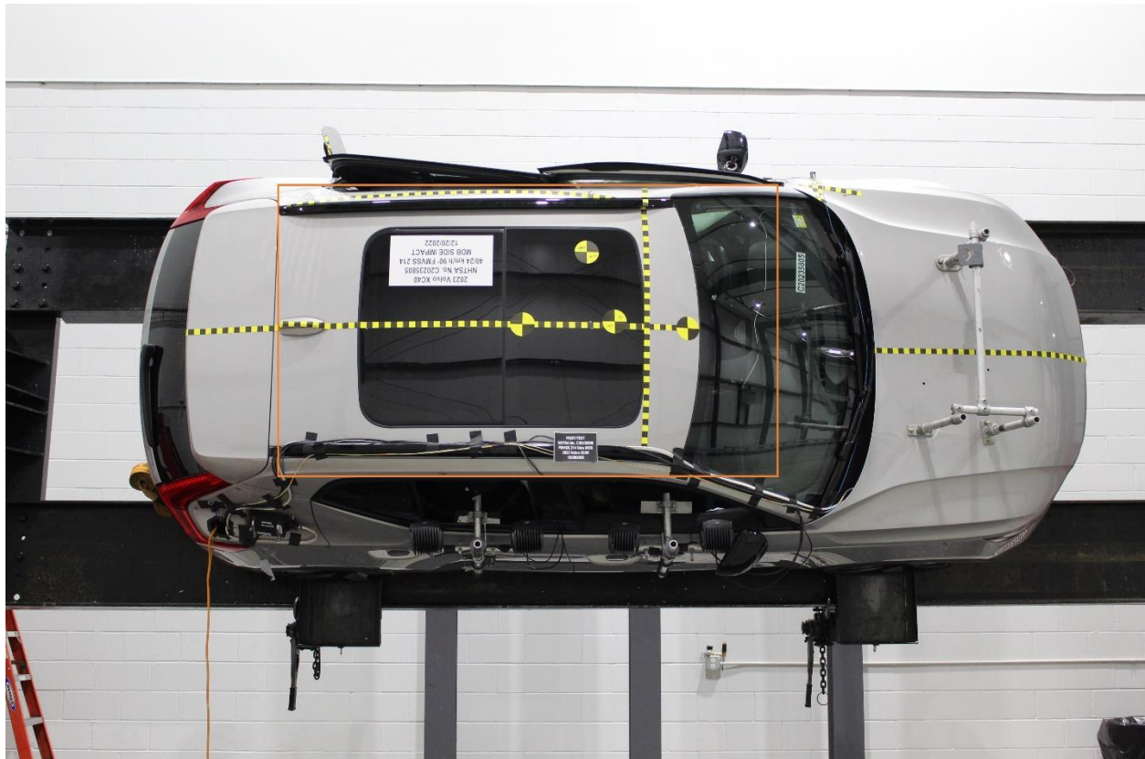
Figure 305-28: FMVSS No. 305 Static Rollover 90 Degrees
