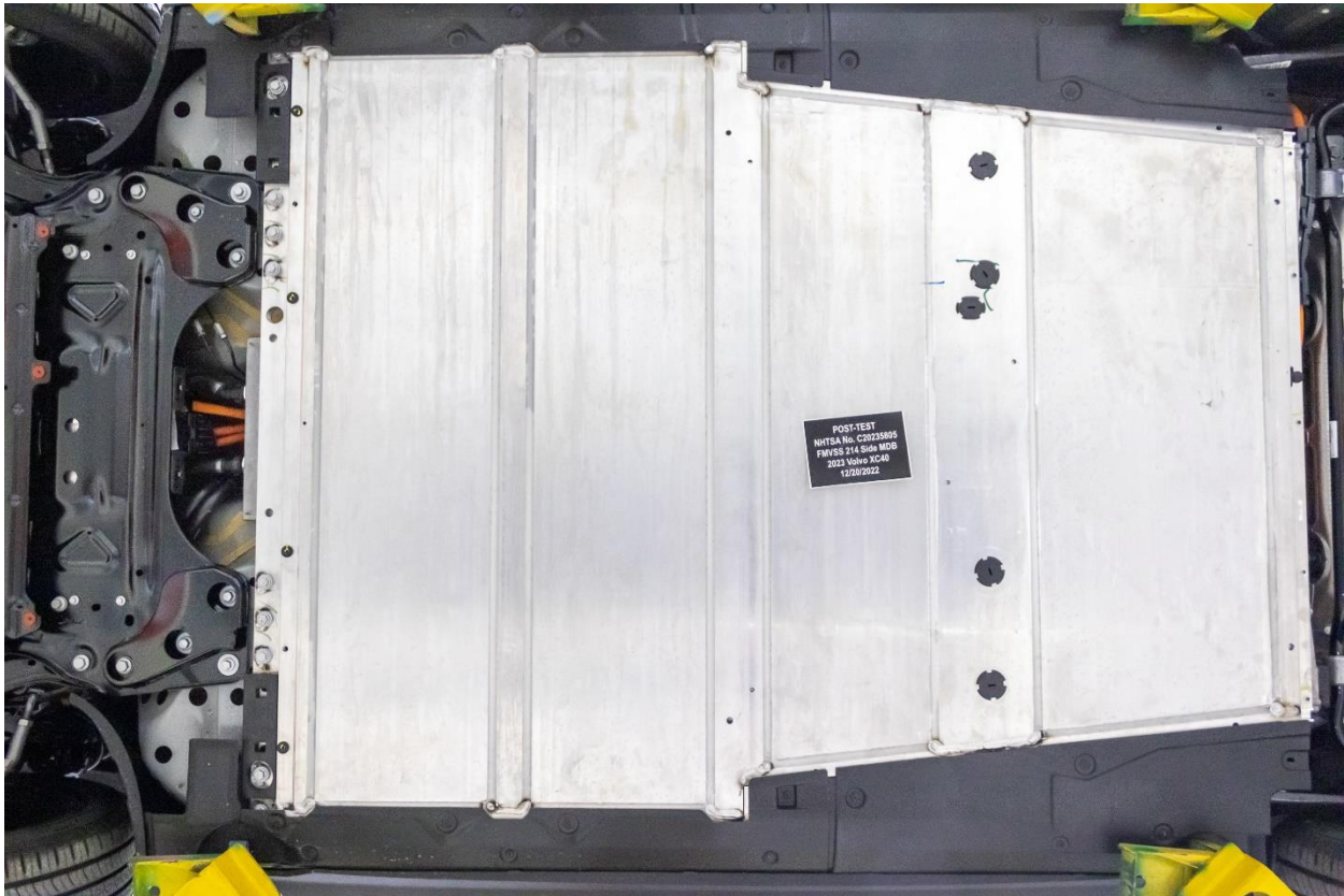
Figure 305-15: Post-Impact View of Propulsion Battery Module(s)
