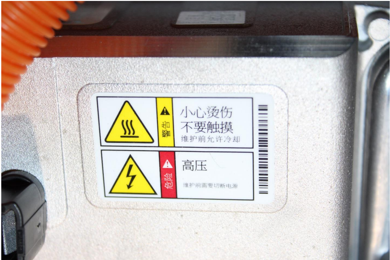
Figure 305-1: Auxiliary Power Module Warning Label
