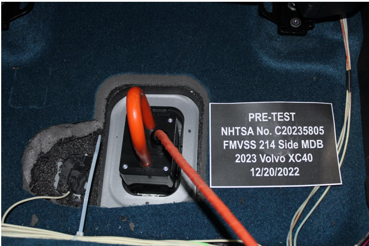
Figure 305-18: Pre-Impact View of High Voltage Interconnects
