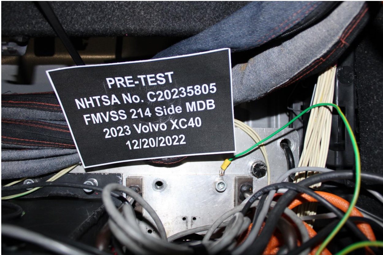
Figure 305-21: Pre-Impact View of Ground Lead Attached
