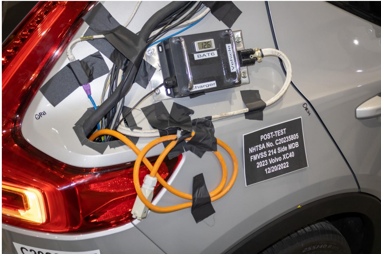
Figure 305-25: Post-Impact View of Installed Test Interface Port
