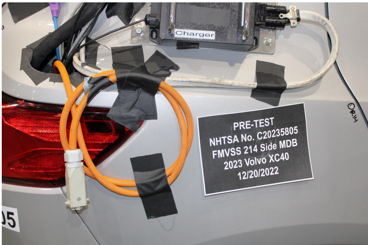
Figure 305-24: Pre-Impact View of Installed Test Interface Port
