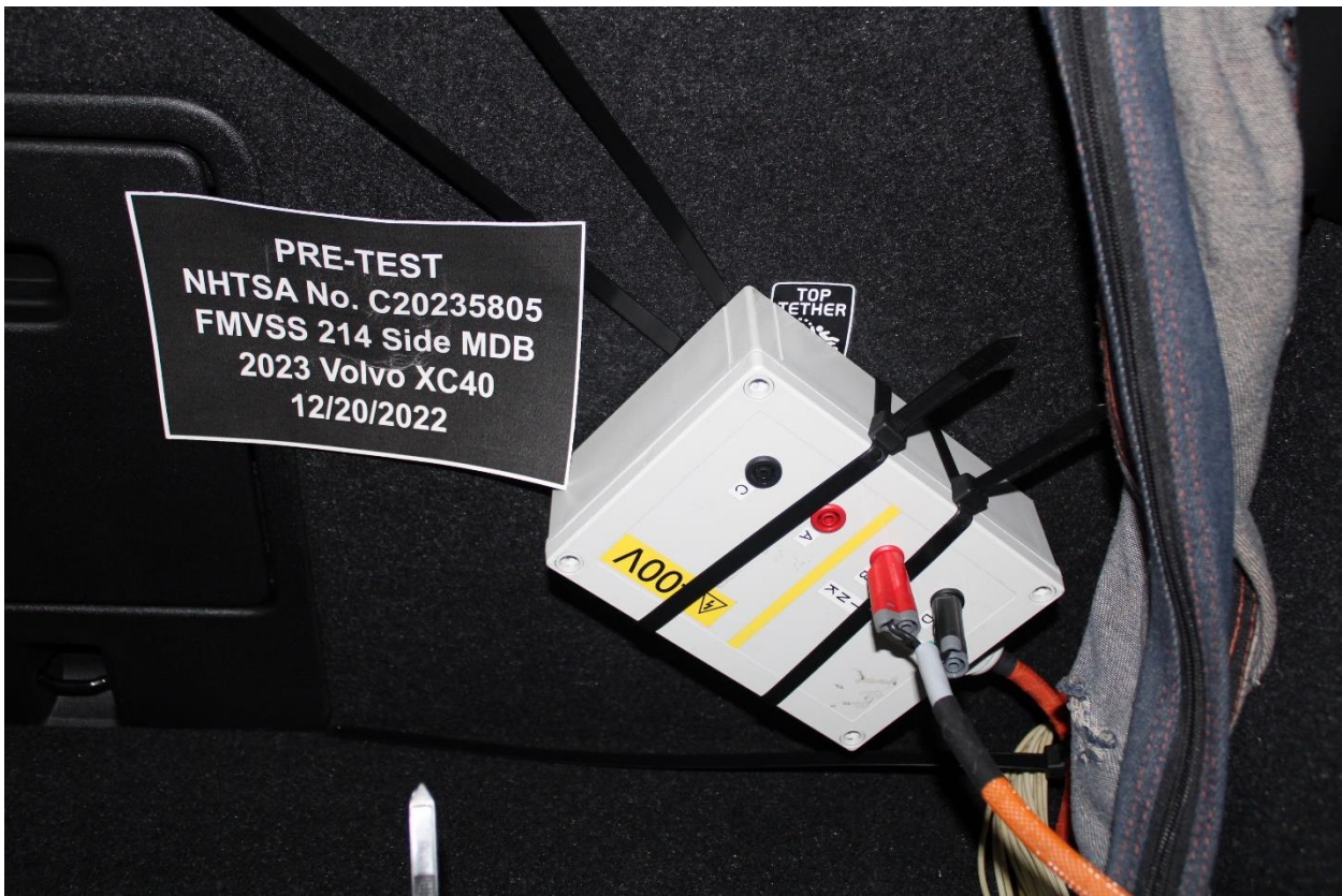
Figure 305-22: Pre-Impact View of High Voltage Leads Attached
