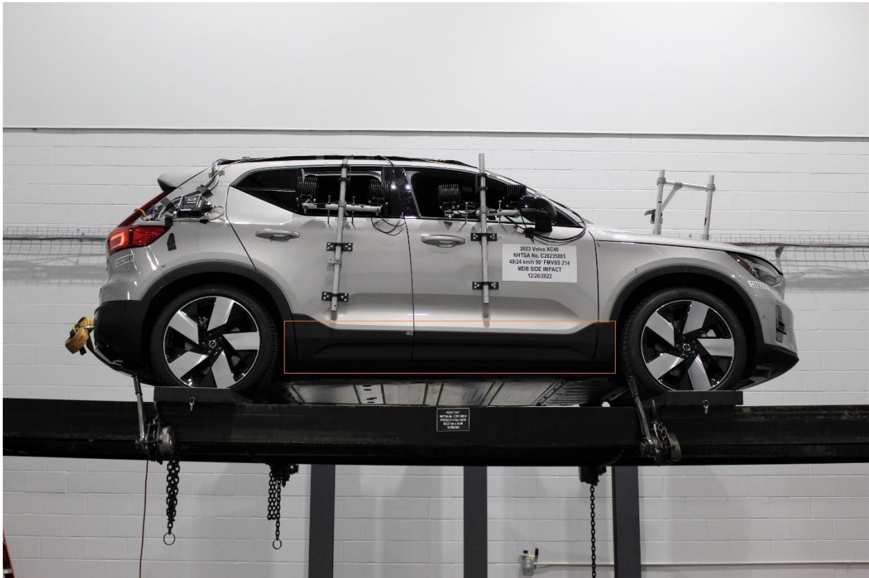
Figure 305-31: FMVSS No. 305 Static Rollover 360 Degrees
