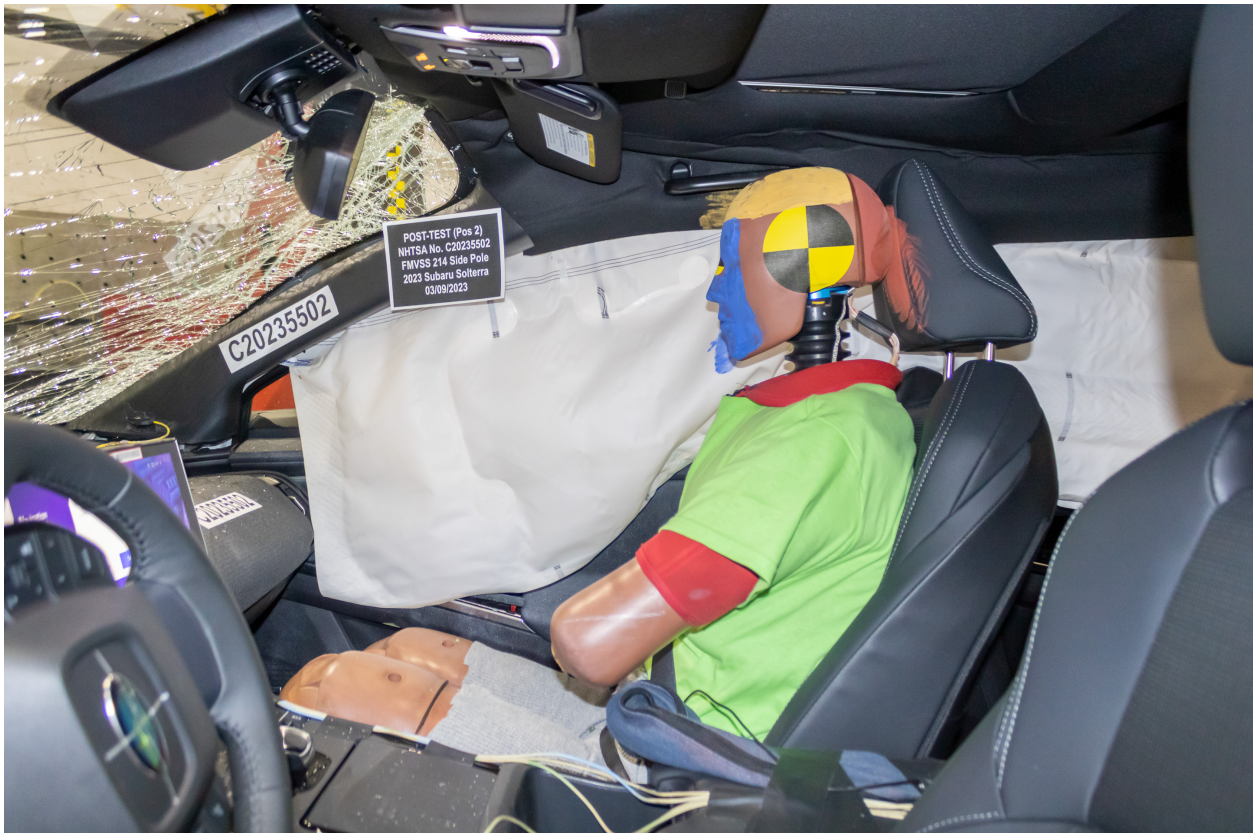
Figure A-12: Post-Test Dummy Through Opposite Window
