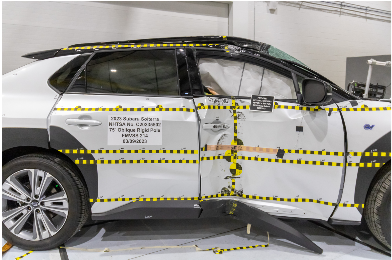
Figure A-21: Post-Test Impact Zone Close-Up View
