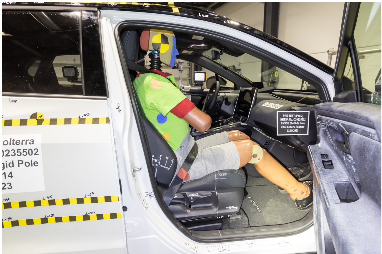
Figure A-15: Pre-Test Dummy with Door Open
