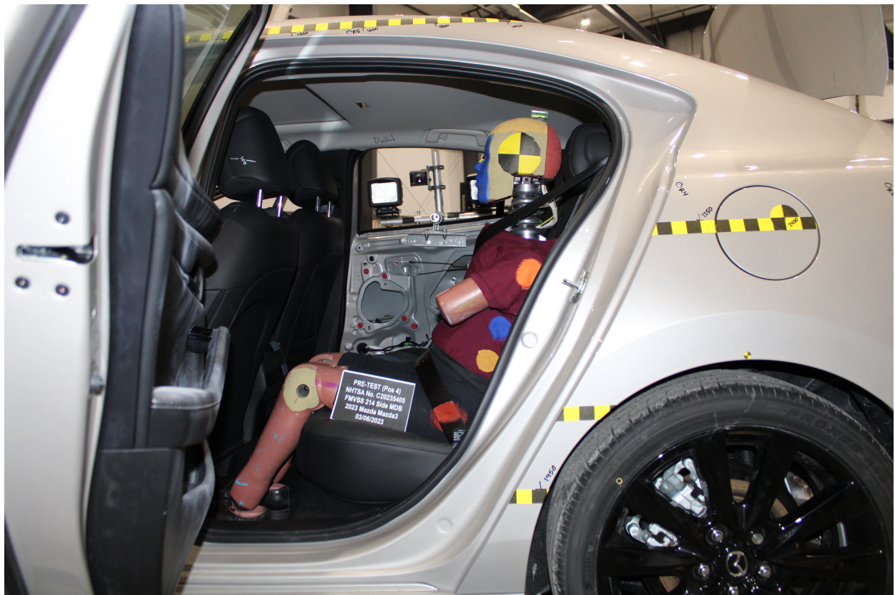
Figure A-21: Pre-Test Rear SID in Final Seating Position (Door Open)
