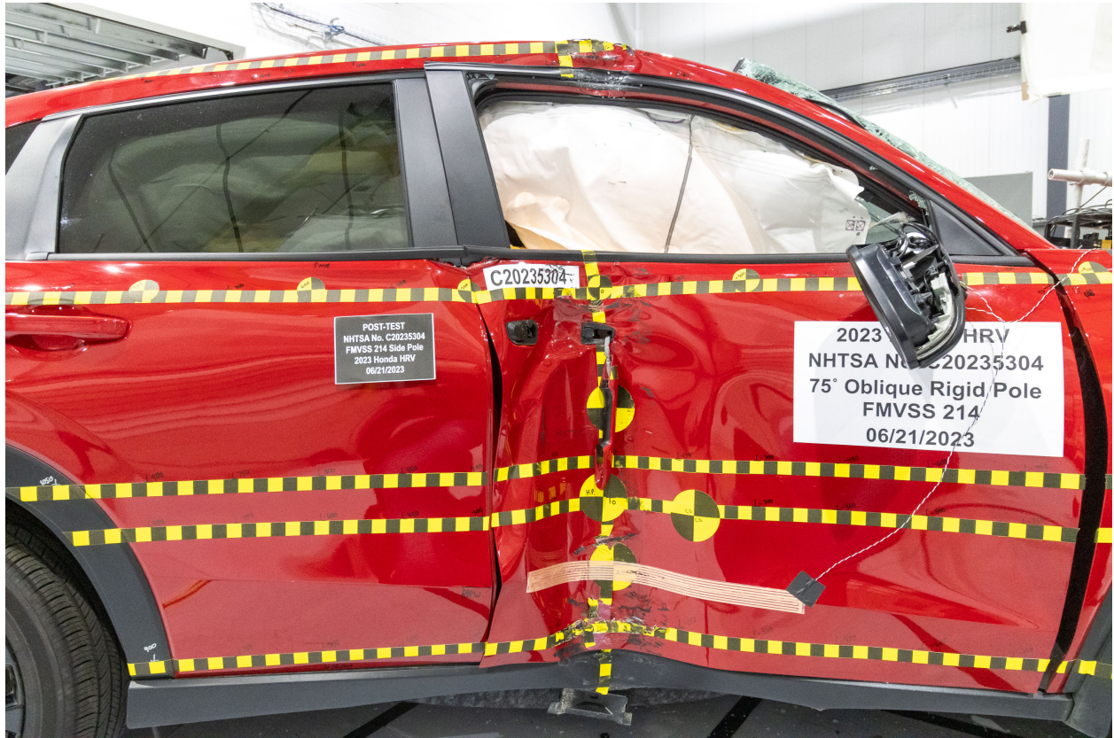
Figure A-21: Post-Test Impact Zone Close-Up View
