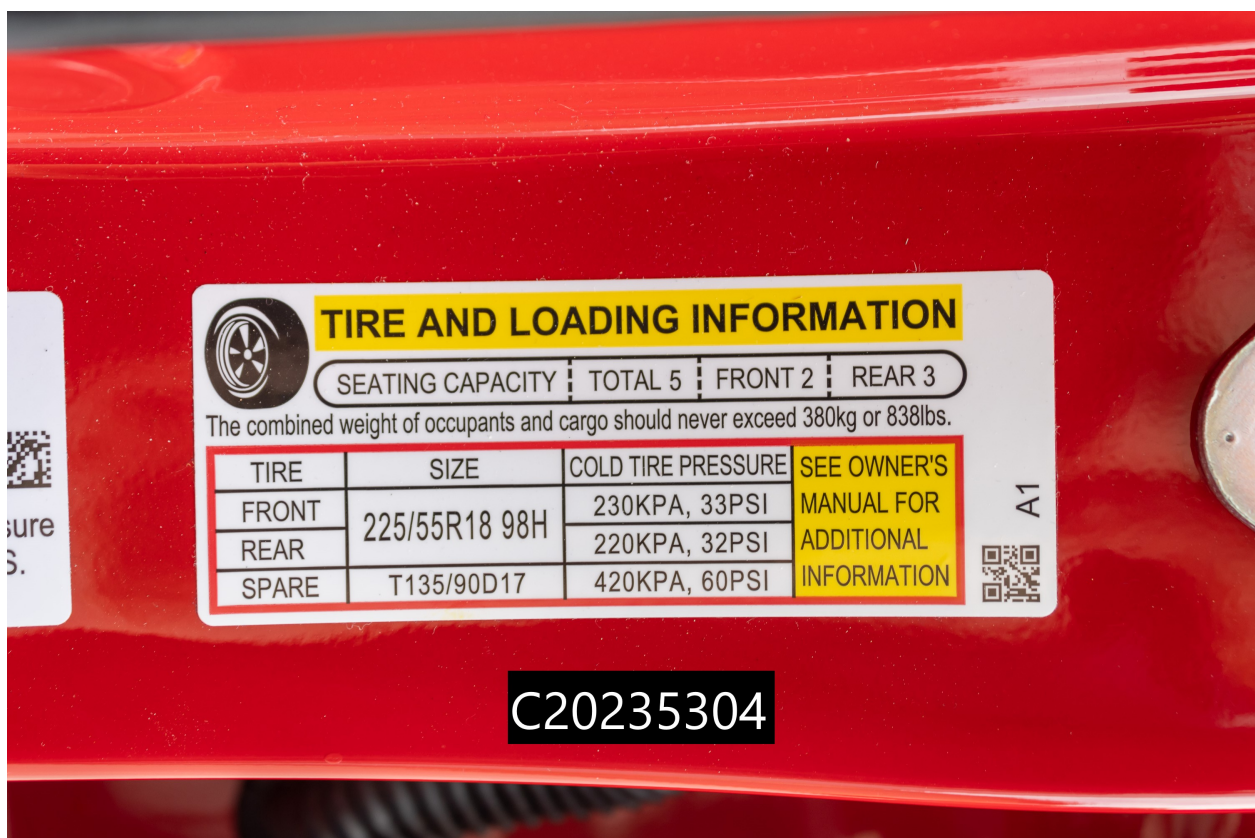
Figure A-26: Close-Up View of Vehicle's Tire Placard Label
