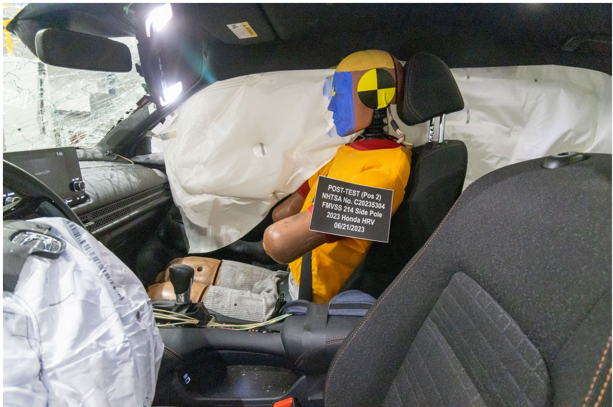
Figure A-12: Post-Test Dummy Through Opposite Window
