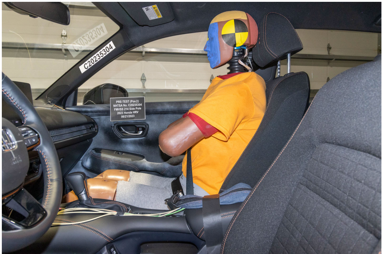
Figure A-11: Pre-Test Dummy Through Opposite Window
