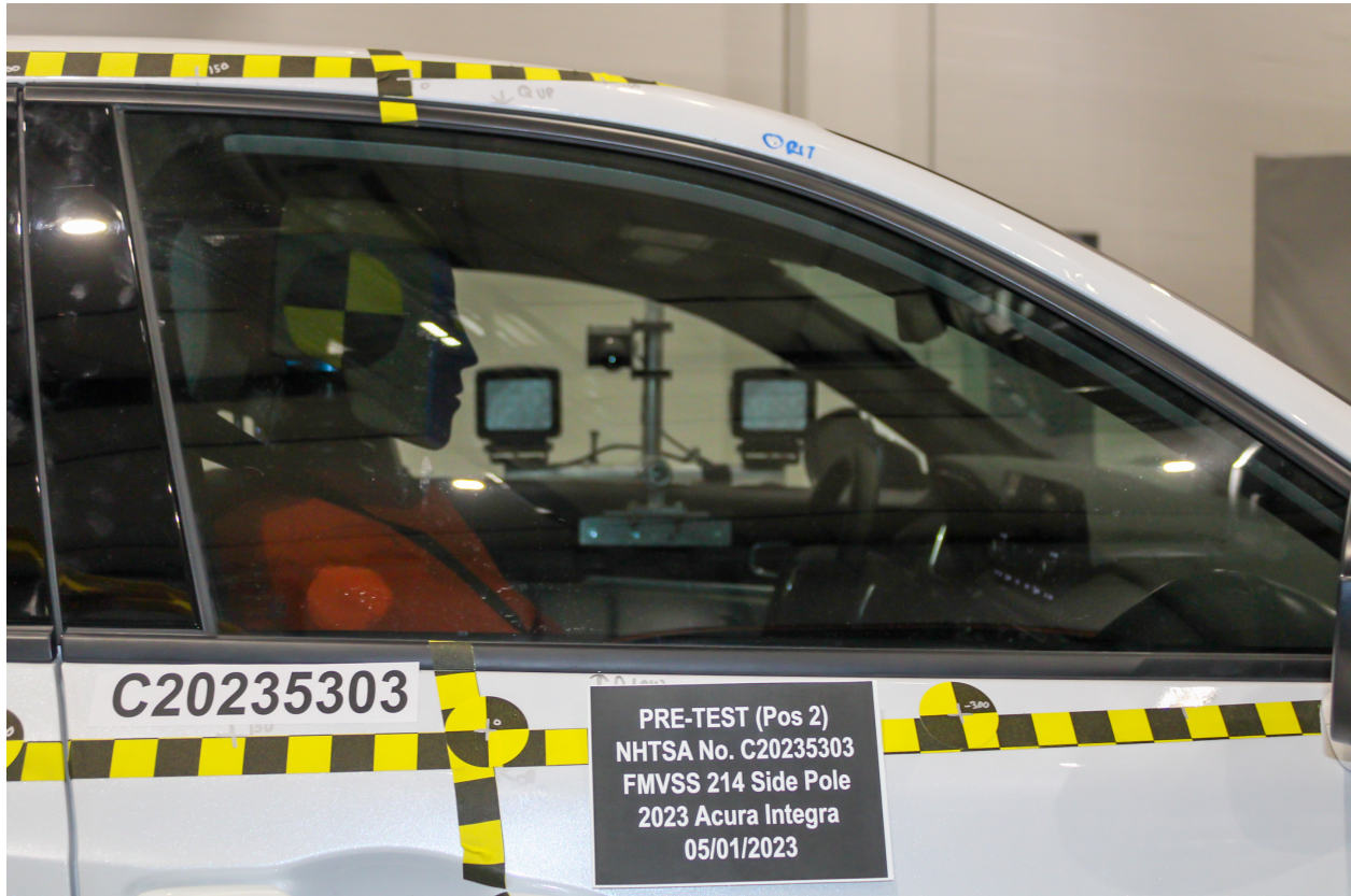
Figure A-13: Pre-Test Close-Up of Dummy with Door Closed (Impact Side)
