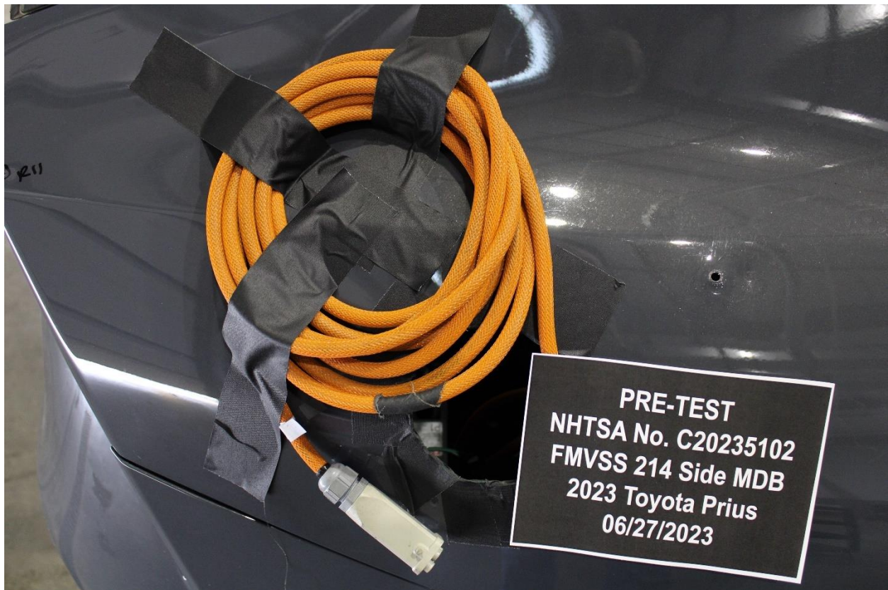
Figure 305-24: Pre-Impact View of Installed Test Interface Port
