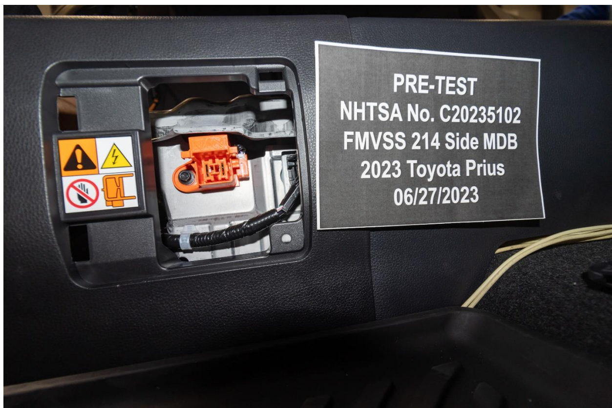
Figure 305-8: Manual High Voltage Service Disconnect Removed Location
