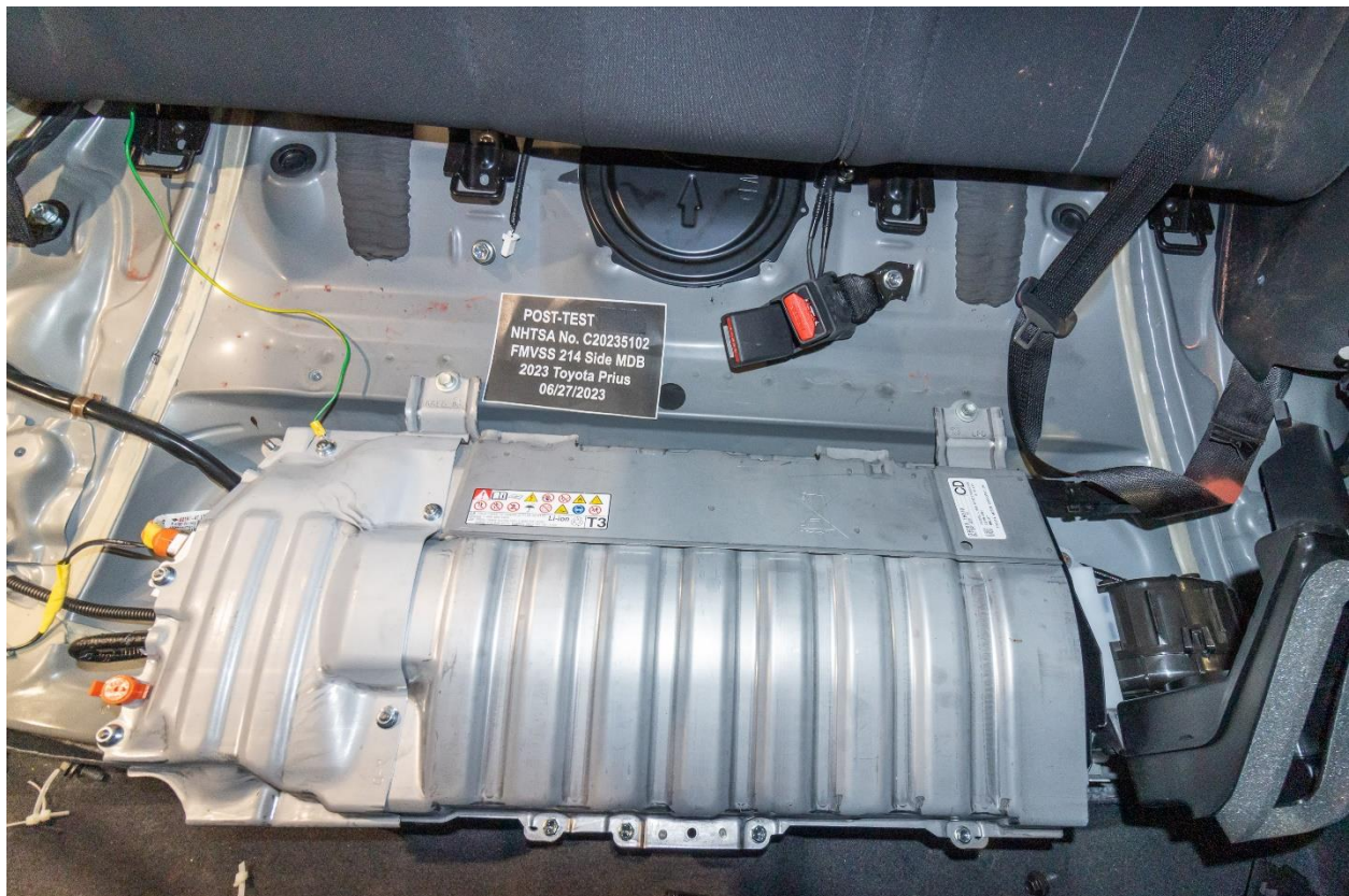
Figure 305-10: Post-Impact Front View of Propulsion Battery
