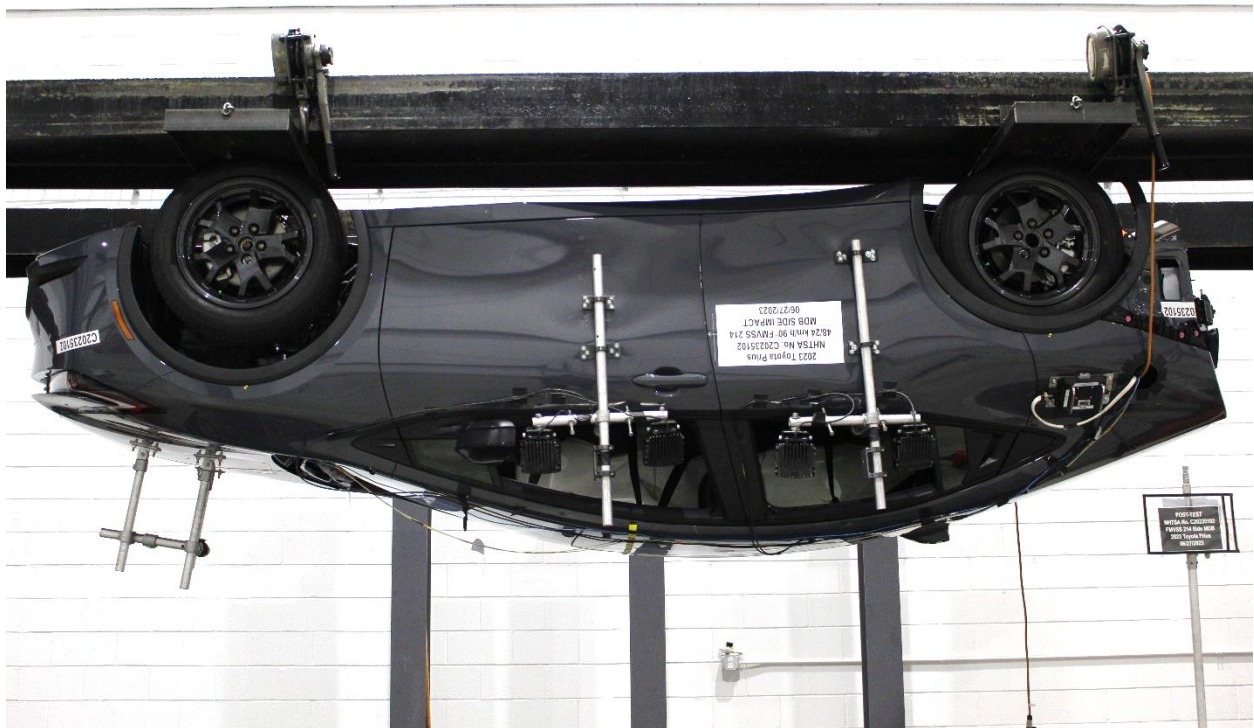
Figure 305-29: FMVSS No. 305 Static Rollover 180 Degrees
