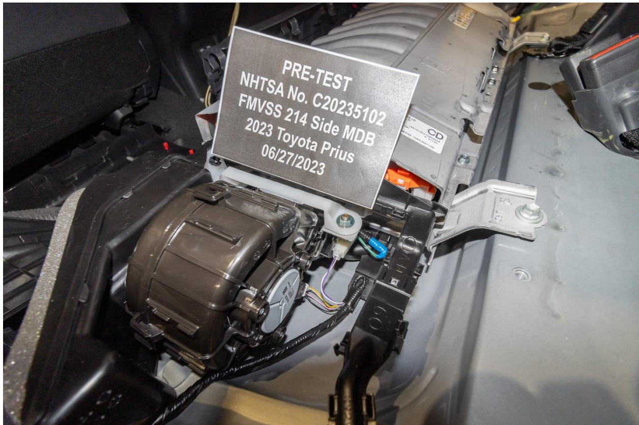
Figure 305-19: Pre-Impact View of Propulsion Battery Venting System
