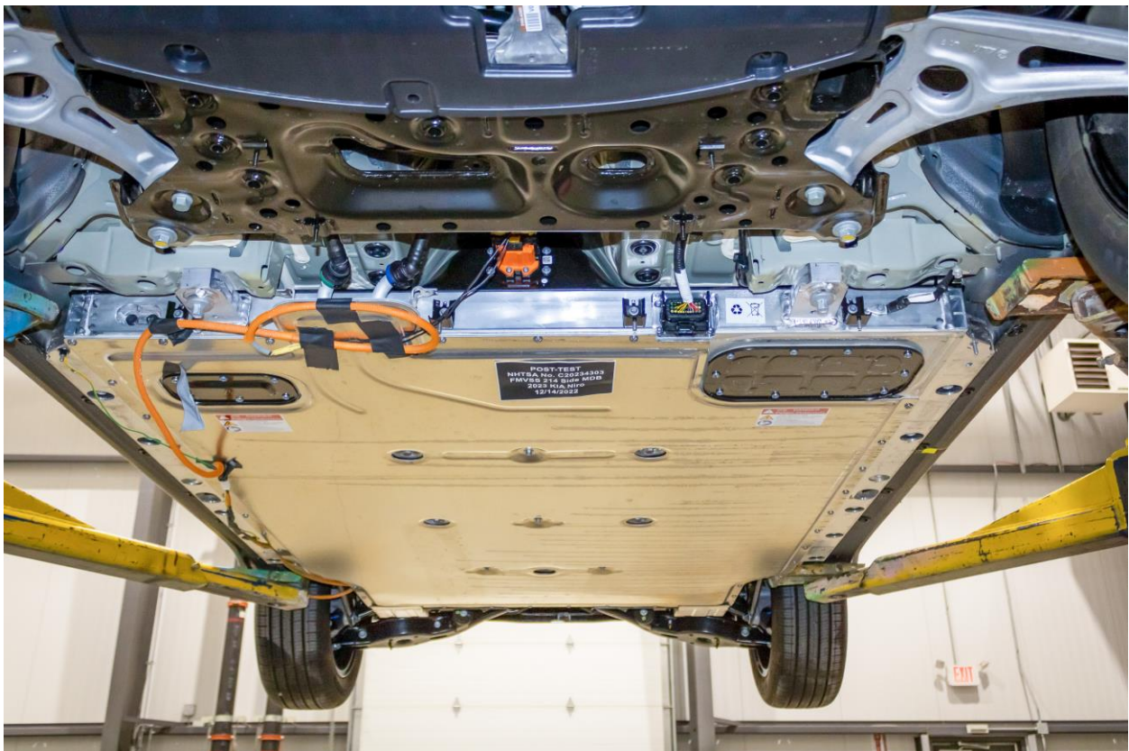
Figure 305-10: Post-Impact Front View of Propulsion Battery
