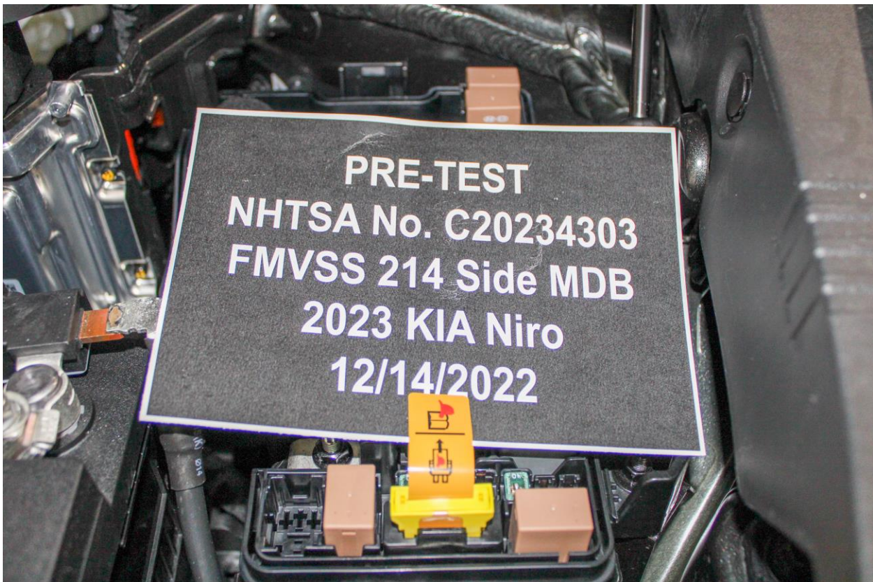
Figure 305-6: Manual High Voltage Service Disconnect in Place
