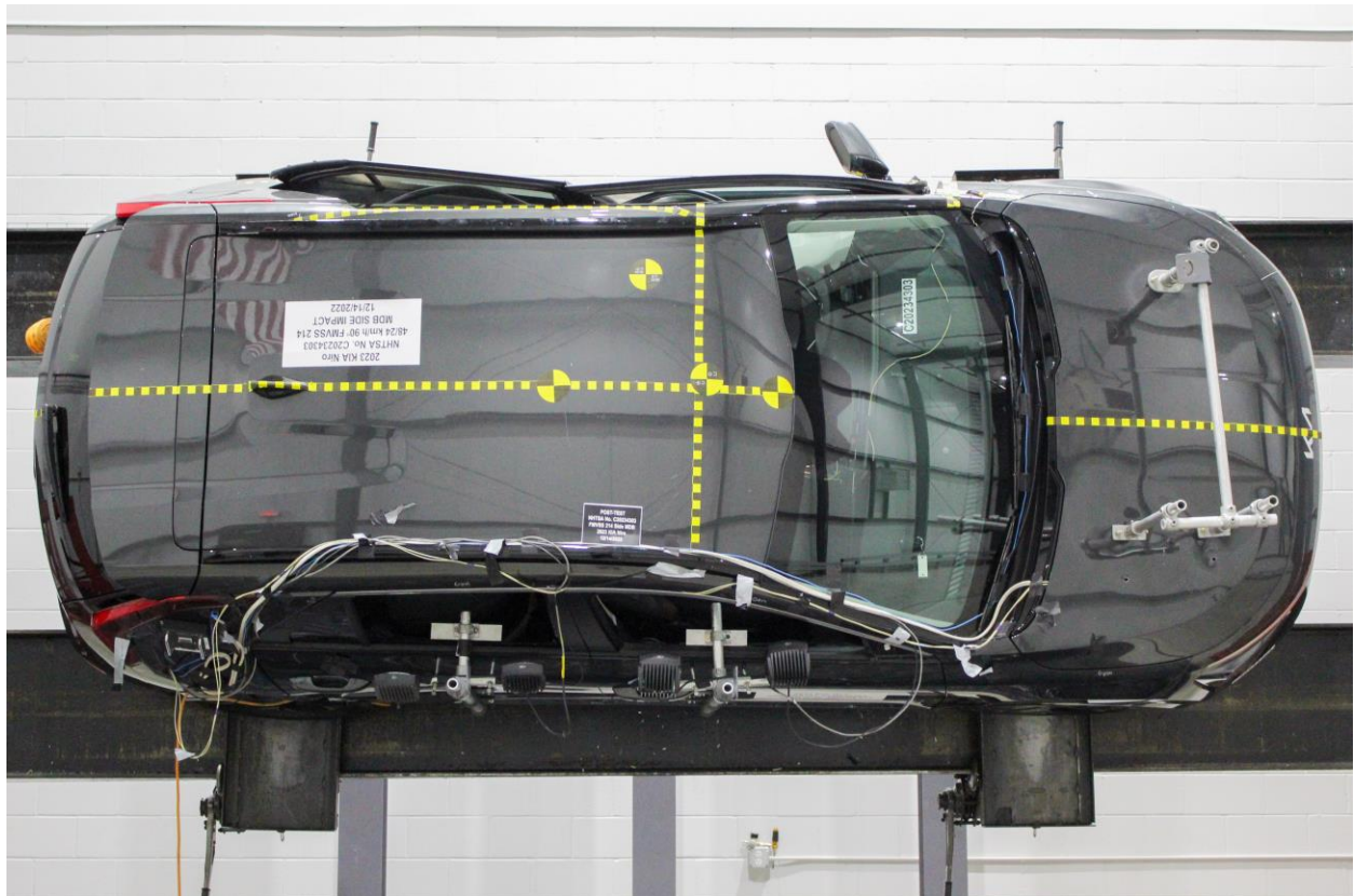
Figure 305-28: FMVSS No. 305 Static Rollover 90 Degrees
