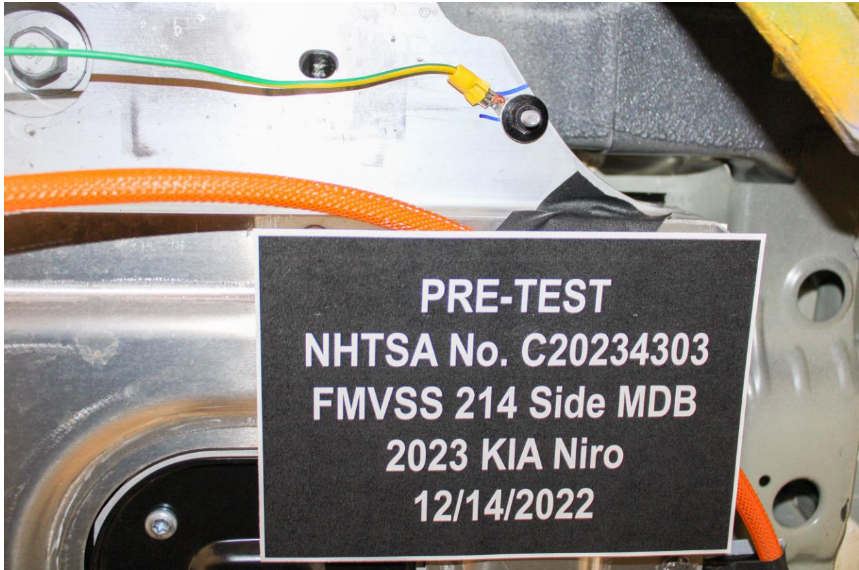
Figure 305-21: Pre-Impact View of Ground Lead Attached
