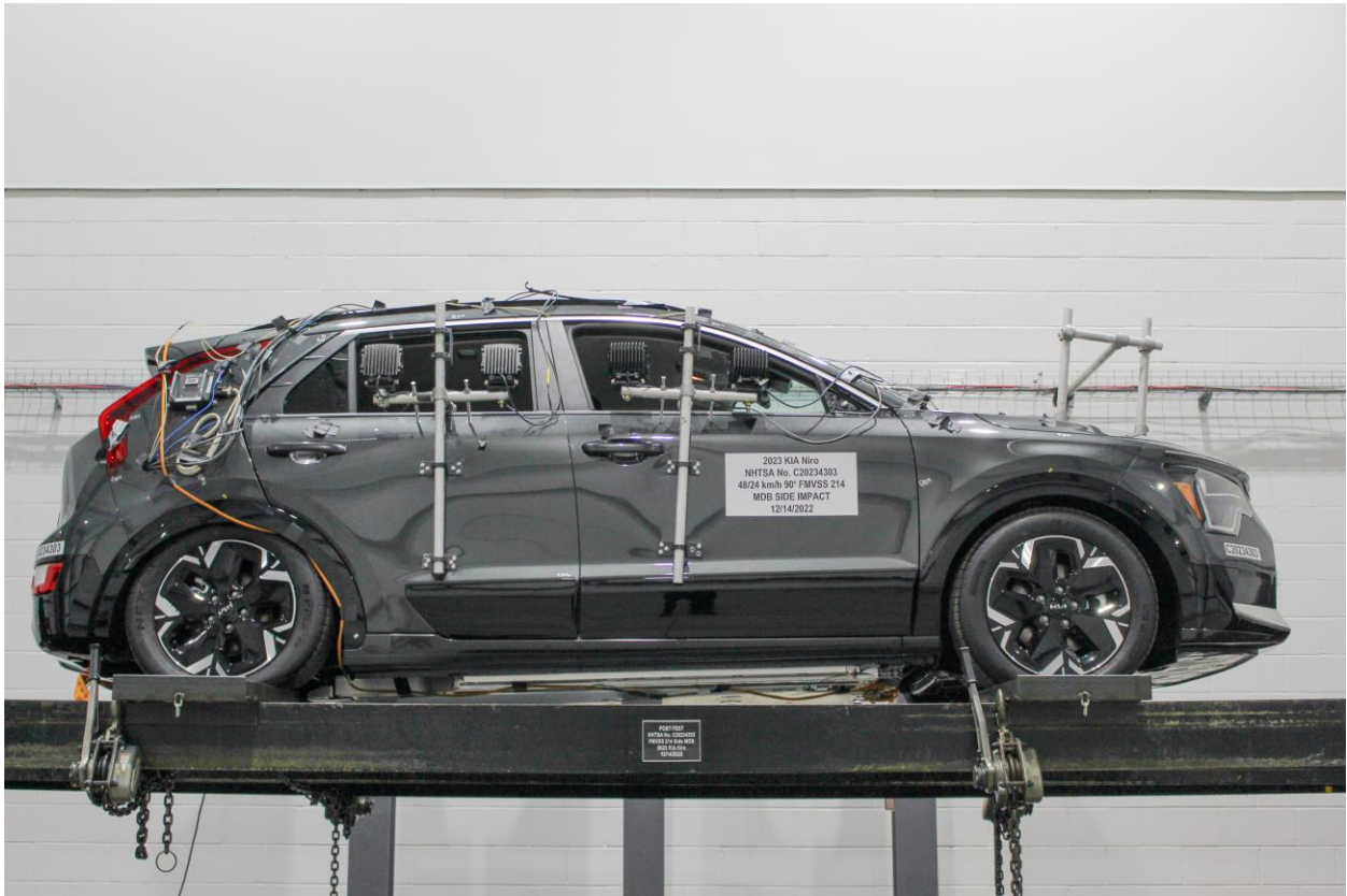
Figure 305-31: FMVSS No. 305 Static Rollover 360 Degrees
