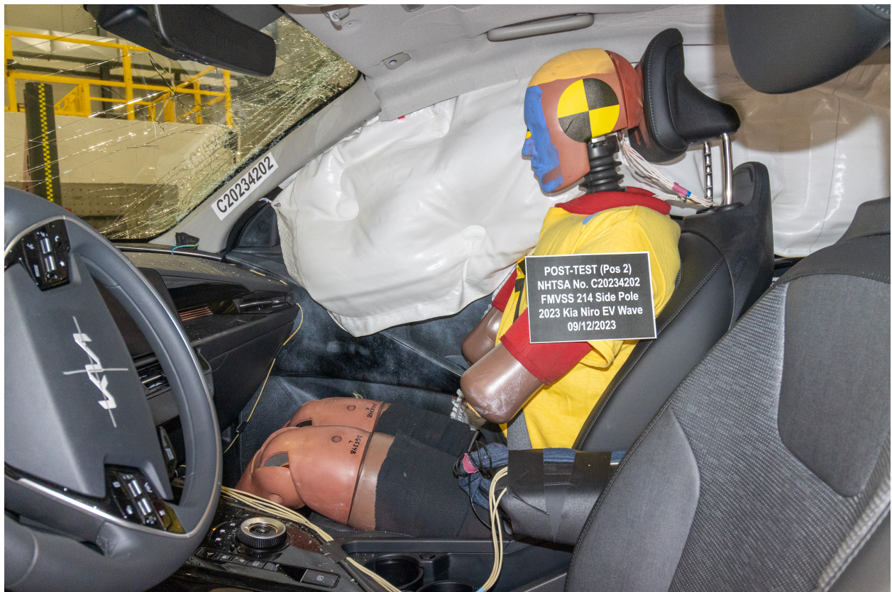
Figure A-12: Post-Test Dummy Through Opposite Window
