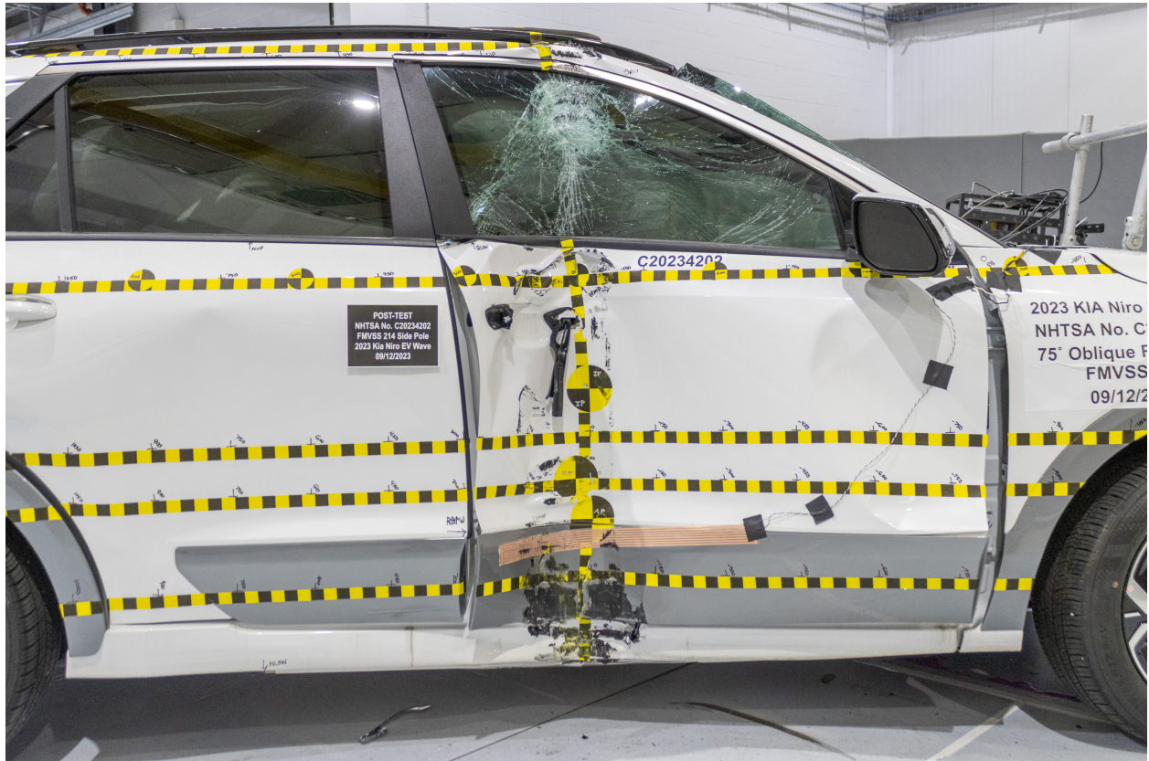
Figure A-21: Post-Test Impact Zone Close-Up View
