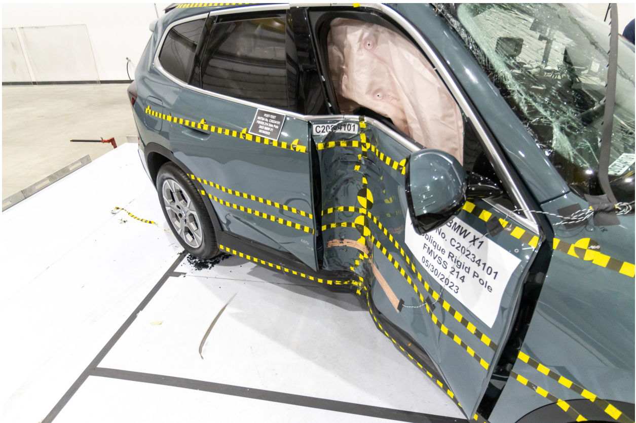
Figure A-22: Post-Test 3/4 Front View of Impact Zone
