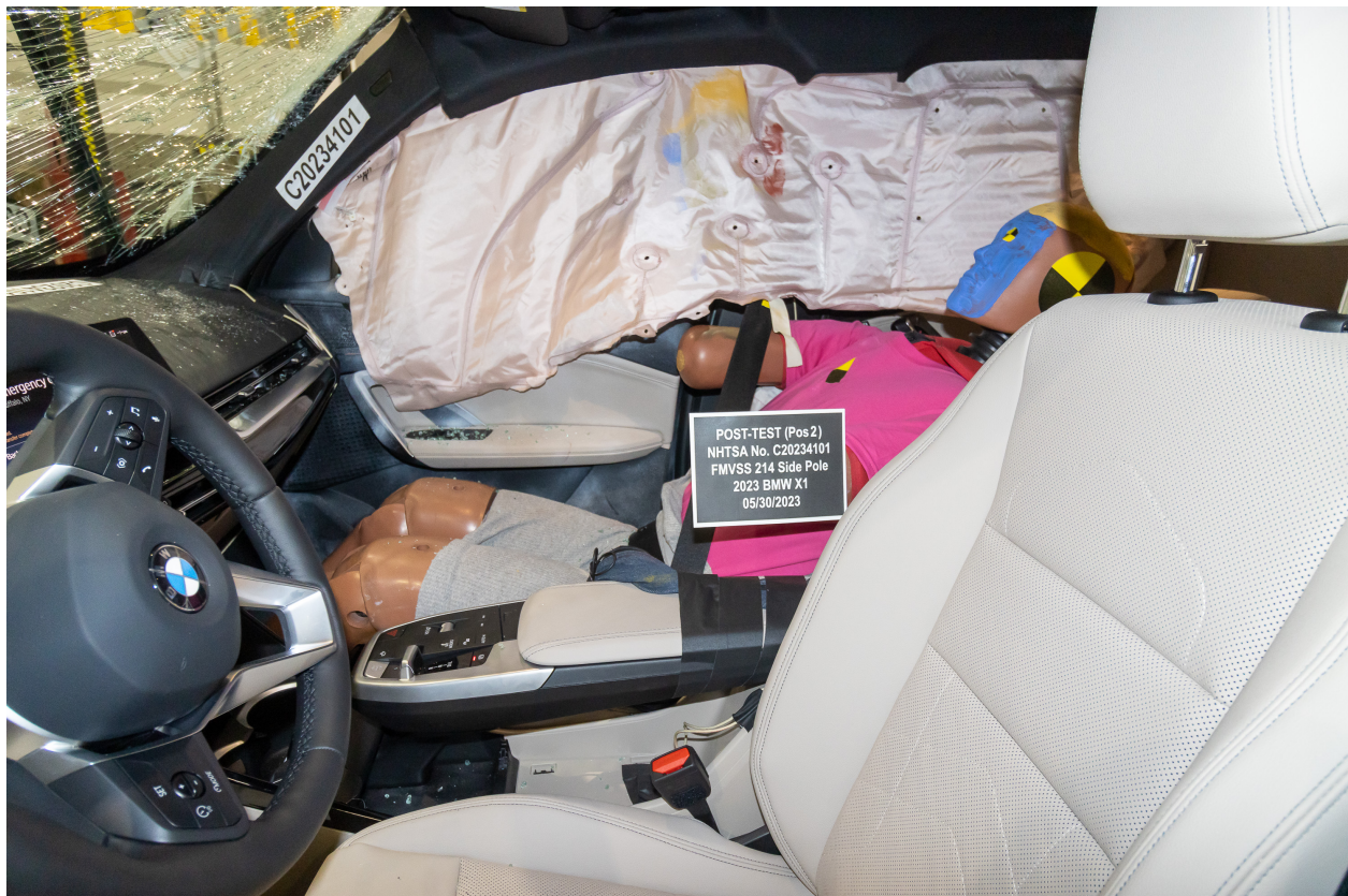
Figure A-12: Post-Test Dummy Through Opposite Window
