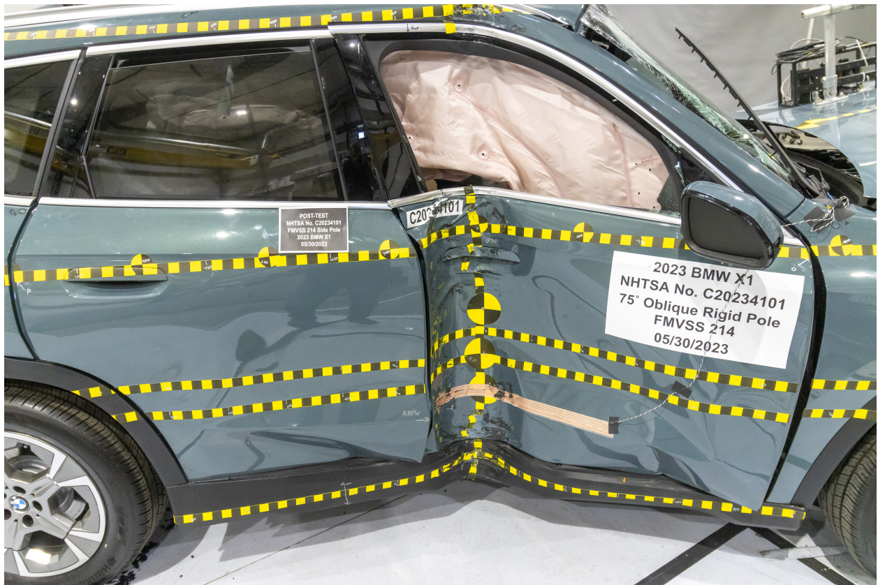
Figure A-21: Post-Test Impact Zone Close-Up View
