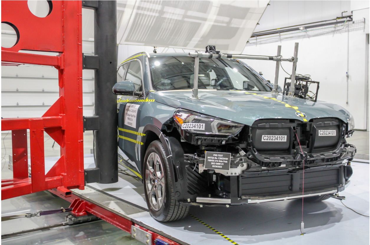
Figure A-7: Pre-Test Right 3/4 Front View of Vehicle and Pole
