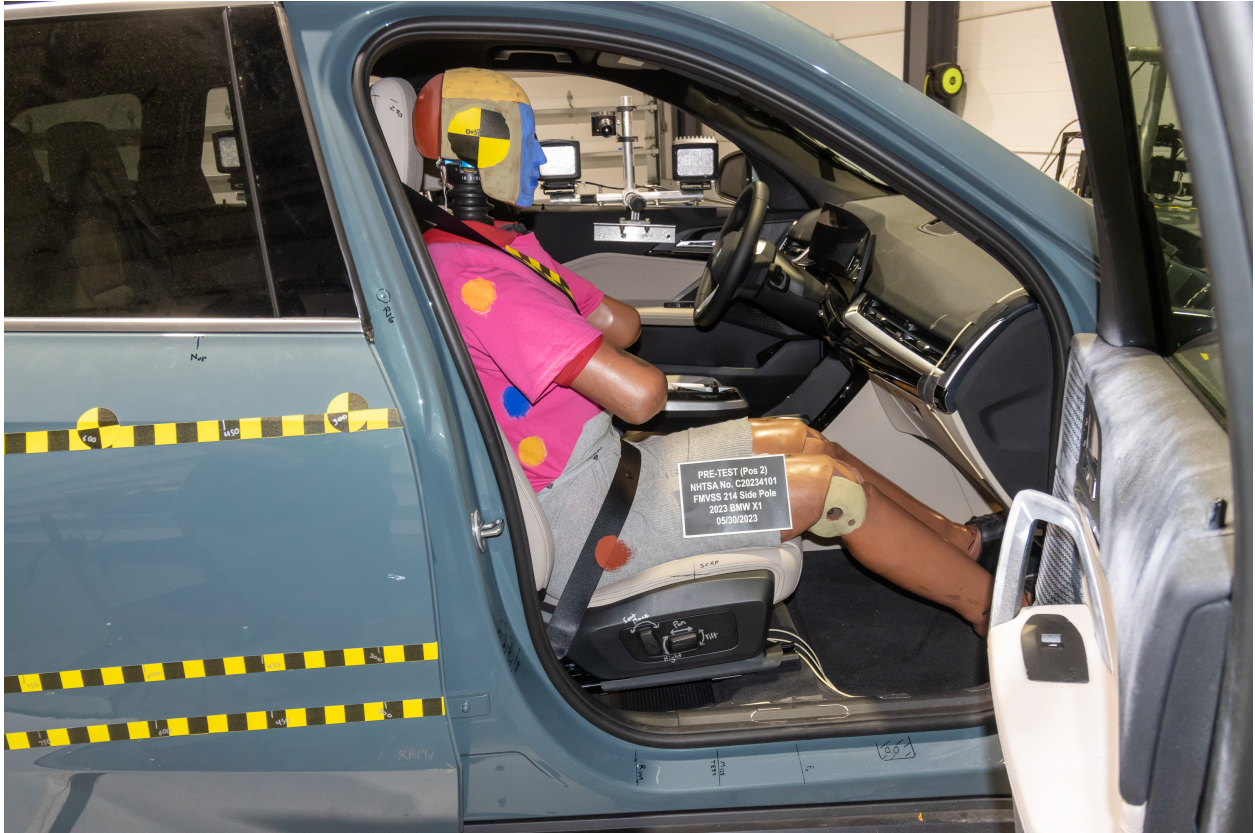
Figure A-15: Pre-Test Dummy with Door Open
